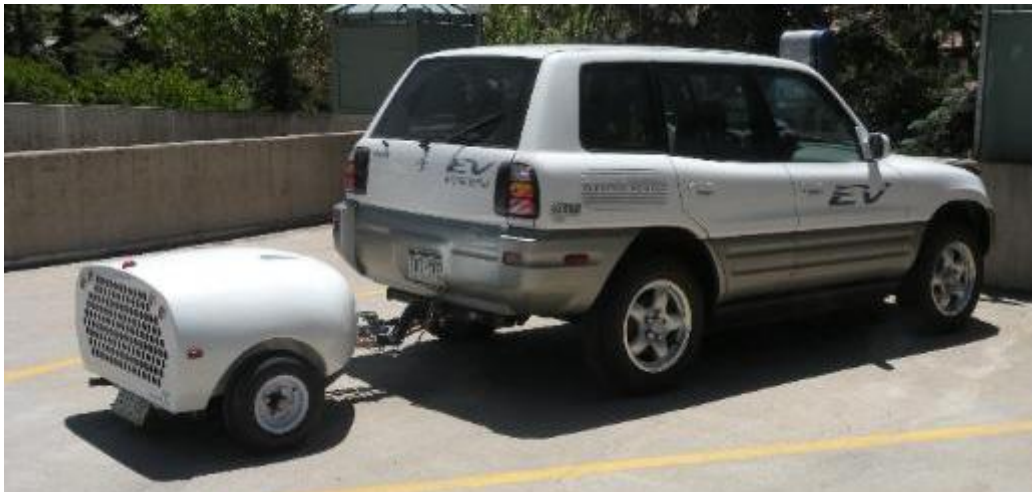
Figure 2.8. An AC Propulsion LongRanger RXT attached to a Toyota RAV4 BEV.
