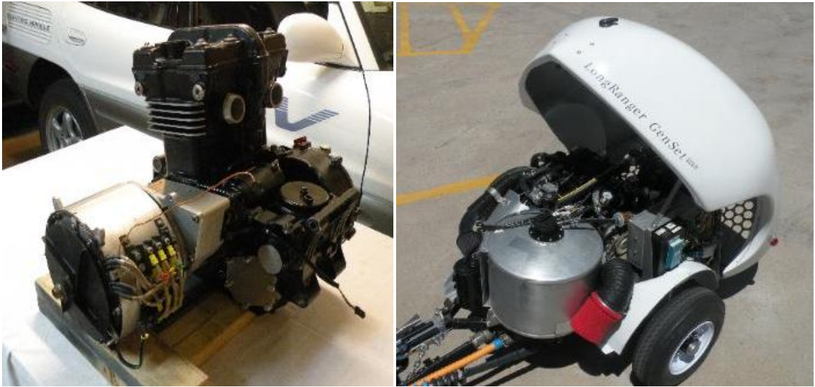
Figure 2.9. AC Propulsion RXT engine and alternator (left) and assembled trailer (right).
