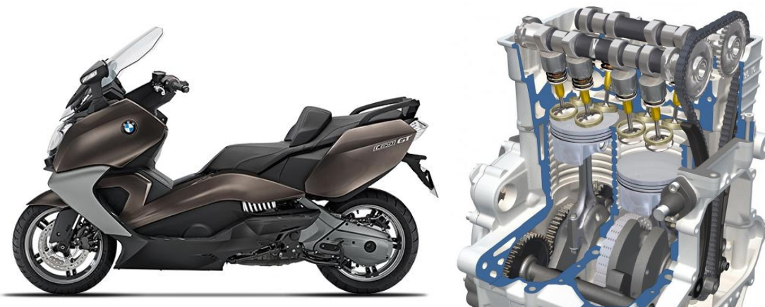
Figure 6.9. BMW Motorrad C 650 GT scooter (left) and engine (right).
