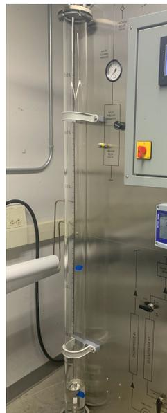
*Figure 3.5: Water Reservoir for CWL*
