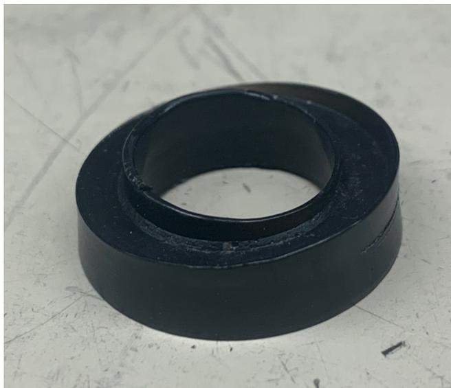
*Figure 3.7: Failed High Pressure Seal*
