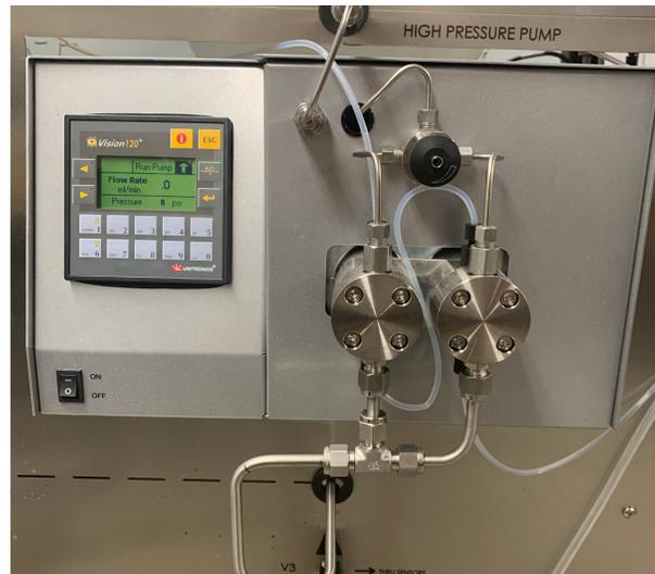
*Figure 3.4: High Pressure Pump Used by the CWL*
