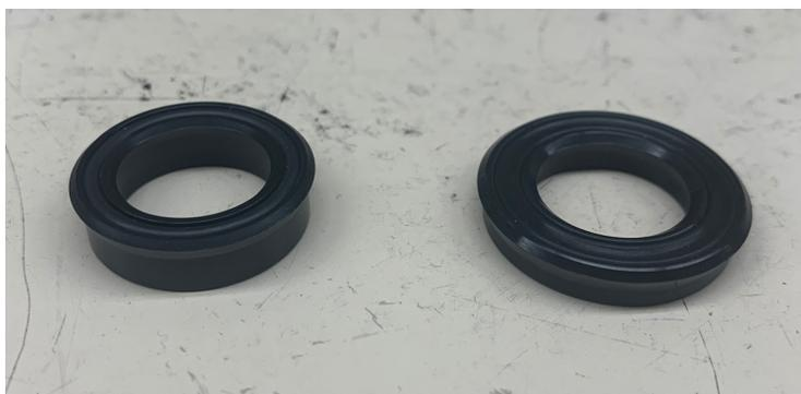
*Figure 3.2: Original Seals Used in the Cooling Jacket*
