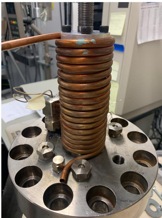
*Figure 3.8: Cooling Jacket with Coils Attached*
