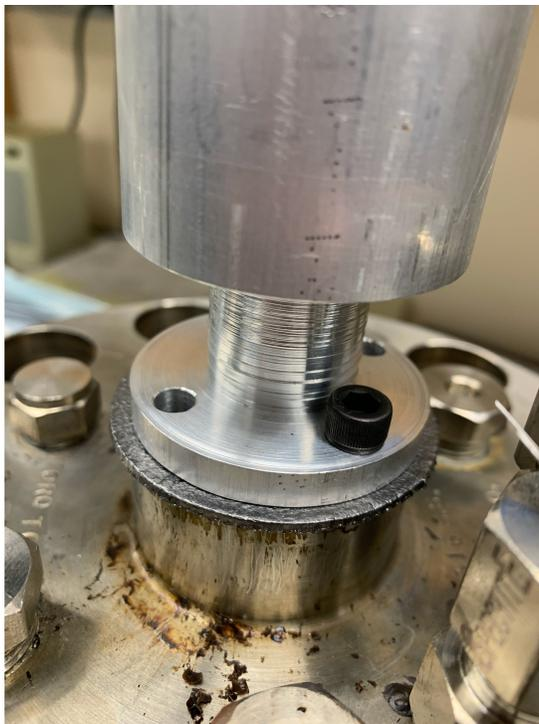
*Figure 3.14: Lower Gasket Attached to Cooling Jacket*
