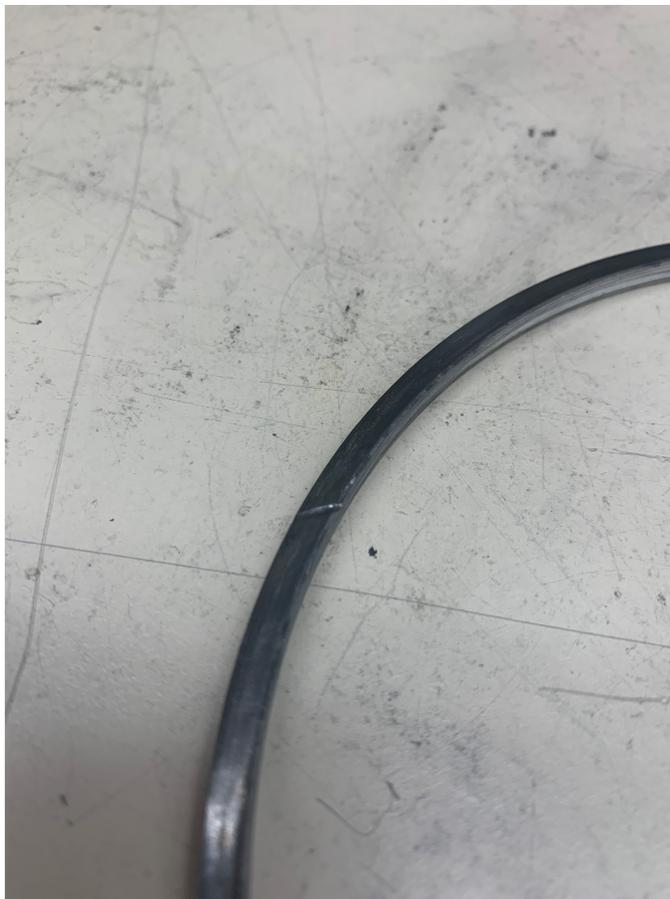
*Figure 3.15: Damage to Autoclave Metal Seal*
