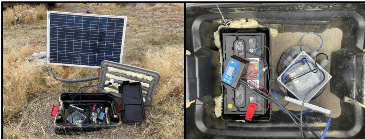
Figure 4. Seismic station composed of the buried, sealable container with solar panel and an inner view of the container with the marine battery and weatherproof case containing the seismometer.
