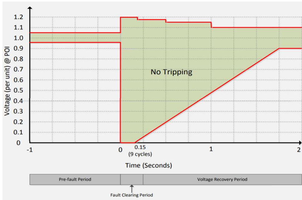
Figure 3-7. Typical voltage ride-through requirements [21].
