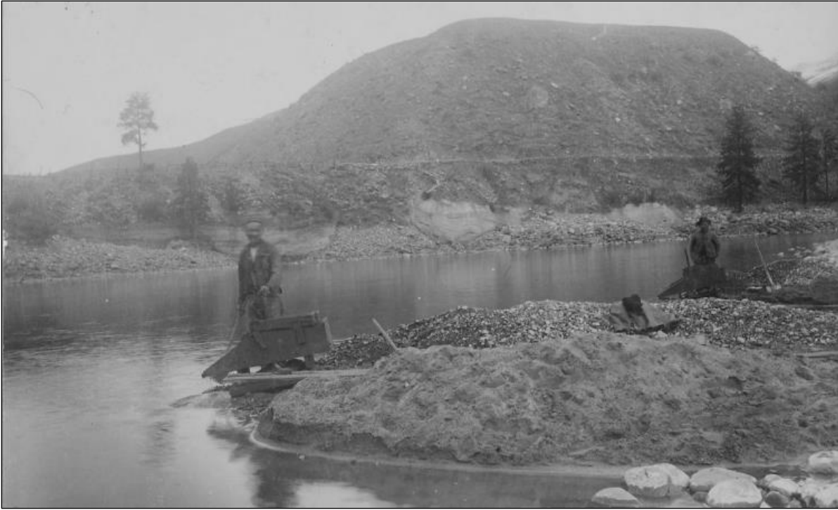
Figure 1.3. Two Chinese placer miners using rockers near Slate Creek, Idaho. The stacked rock behind the miner in the foreground is a tailings pile. Idaho State Archives photo no. 1268-A.
