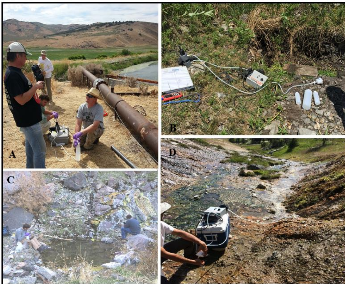
Figure A1. (A) Sample team comprised of U of I graduate student Cody Cannon (mid left), INL scientist Travis McLing (mid right), Dr. Mark Conrad (foreground) of the LBNL, and Dr. Pat Dobson (background) of the LBNL. (B) Sample equipment set up showing the peristaltic pump and tubing, 0.45µm filter, YSI® Professional Plus Multimeter and Flow-Through Cell, and three sample bottles. (C) Sampling of Driscoll Spring near Twin Falls, ID. (D) Utilization of a coiled cooling system prior to sampling collection at Worswick Hot Springs, ID.
