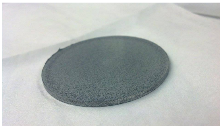
FIGURE 3.6: A photograph of a custom made \text{Mg}_{0.07}\text{Zn}_{0.93}\text{O} target, made to contain 7% Mg, pressed by a Carver hydraulic press.
