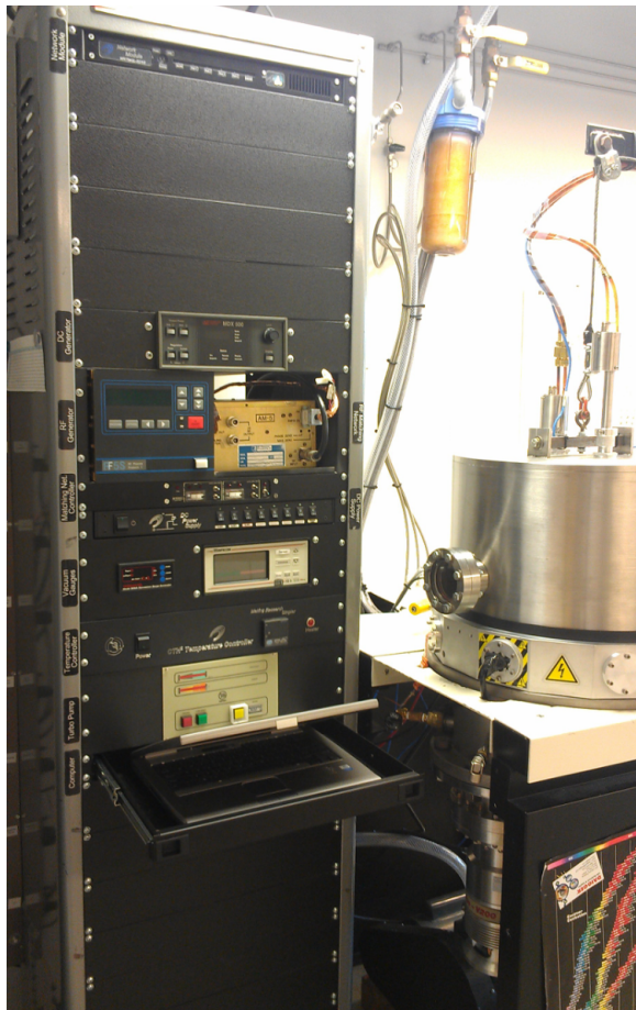
FIGURE 3.5: A photograph of the sputtering system used in this work. On the right is the growth chamber, beneath which can be seen the turbo molecular vacuum pump backed by the mechanical roughing pump. On the left is an equipment rack with all accompanying control electronics and power sources.
