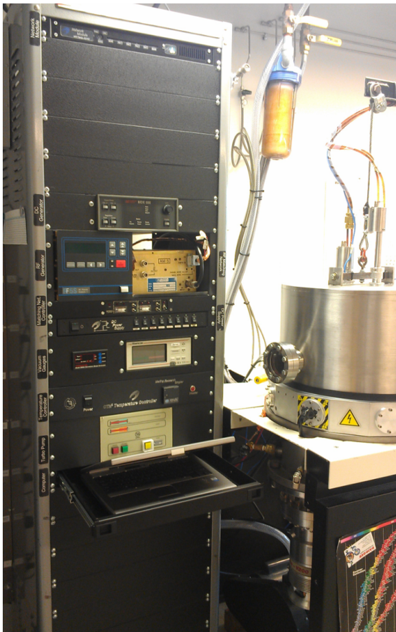
FIGURE 2.5: A photograph of the sputtering system used in this work. On the right is the growth chamber, beneath which can be seen the turbo molecular vacuum pump backed by the mechanical roughing pump. On the left is an equipment rack with all accompanying control electronics and power sources.
