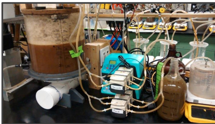
Figure 19: Enrichment reactor with feed and decant pumps
