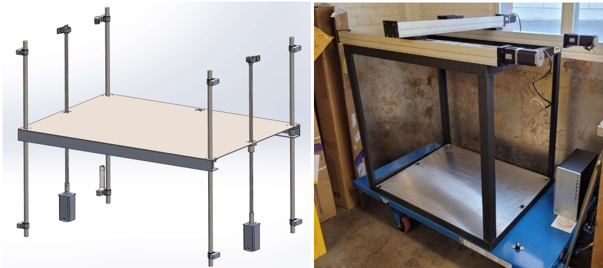
Figure 3-2: (Left) Two linear screws for Z-axis. (Right) Welded 3D printer frame with enclosed linear screws.
