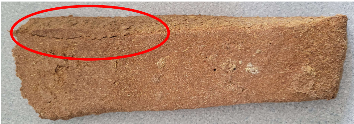
Figure 6-19: Failure occurred in the base material not at layer boundary.
