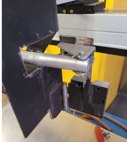
Figure 3-35: 957 N linear actuator with nozzle in 90-degree position.
