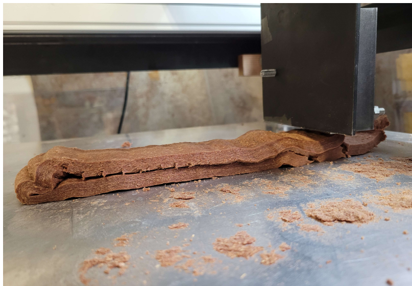
Figure 5-11: Printed material held at beginning of print with second layer.
