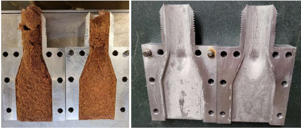
Figure 3-26: (Left) WSSC cured inside nozzle. (Right) Residue left behind after cleaning.
