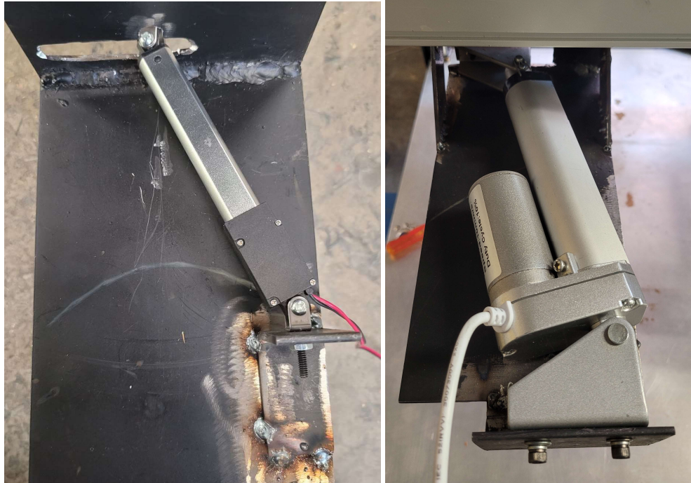
Figure 3-33: (Left) 63 N holding force linear actuator. (Right) 957 N holding force linear actuator.
