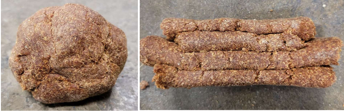
Figure 5-14: (Left) Pressed ball extrudate. (Right) Vertically pressed extrudate.
