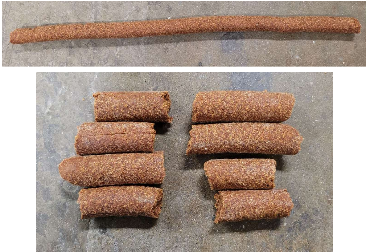
Figure 5-13: (Top) Extruded Rod. (Bottom) Rods broken into pieces.
