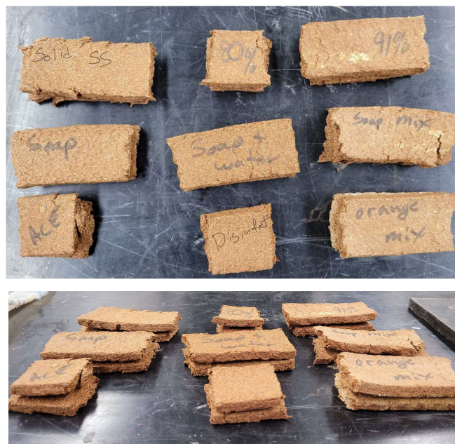
Figure 6-14: Failed interlayer connections
