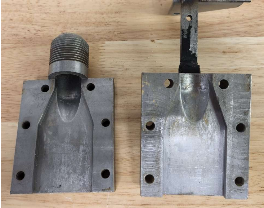
Figure 3-28: V5 nozzle made of 1018 steel.
