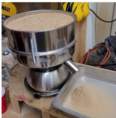
Figure 5-1: Less than 40 mesh wood flour being sieved.
