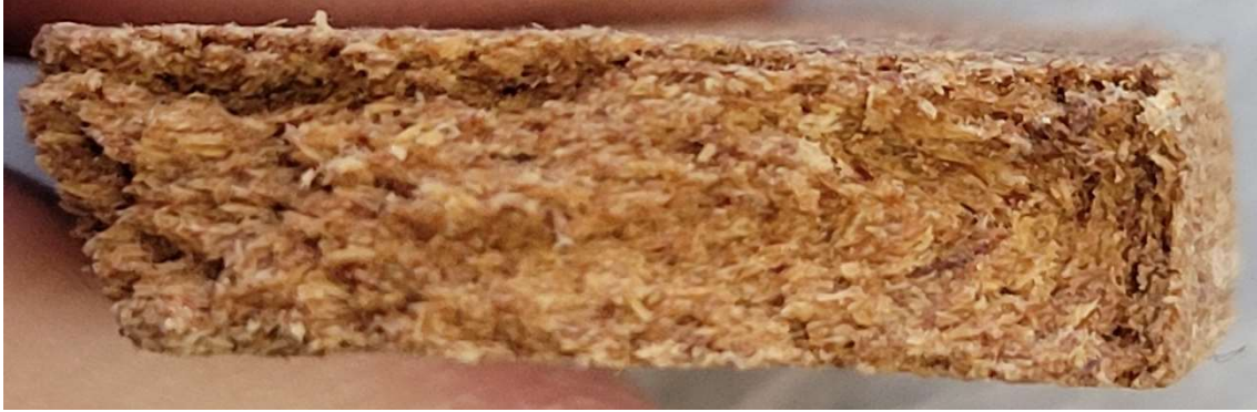
Figure 6-4: Fiber configuration of rectangular extrudate.
