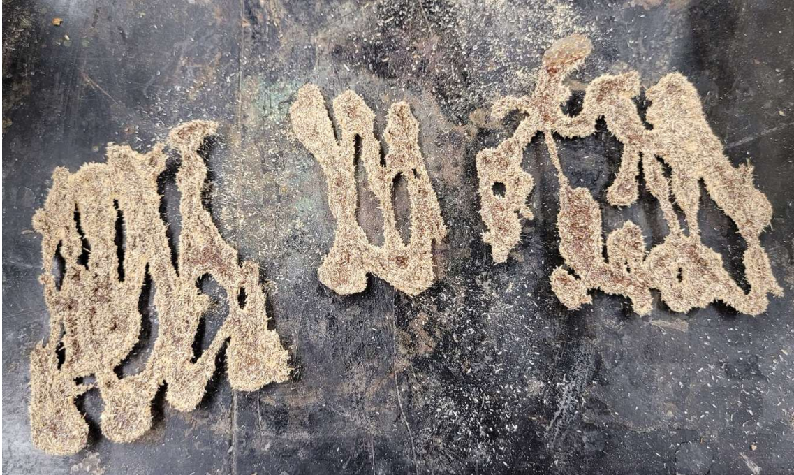
Figure 6-10: Ink jetting of sodium silicate onto wood flour.
