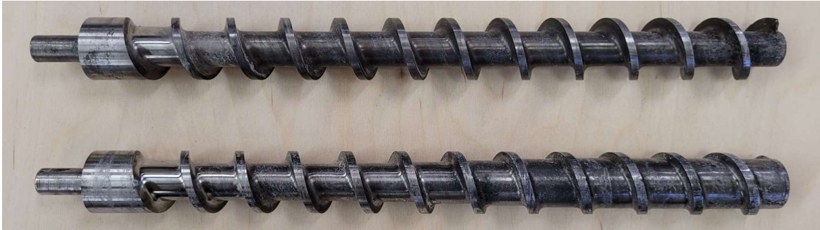
Figure 5-7: Zero-compression and compression screws.
