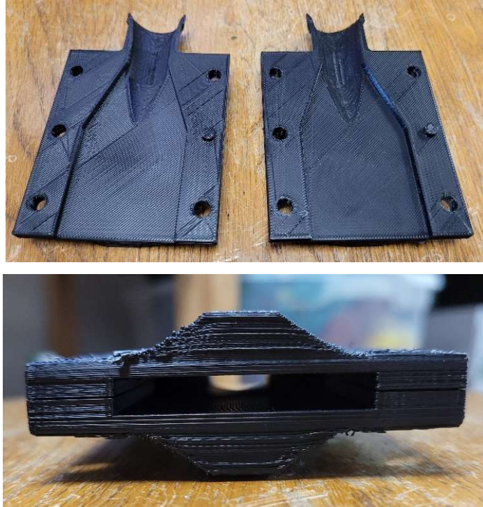
Figure 3-20: (Top) V2 nozzle halves. (Bottom) Exit of nozzle.
