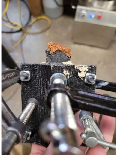
Figure 3-22: Failed V2 nozzle.
