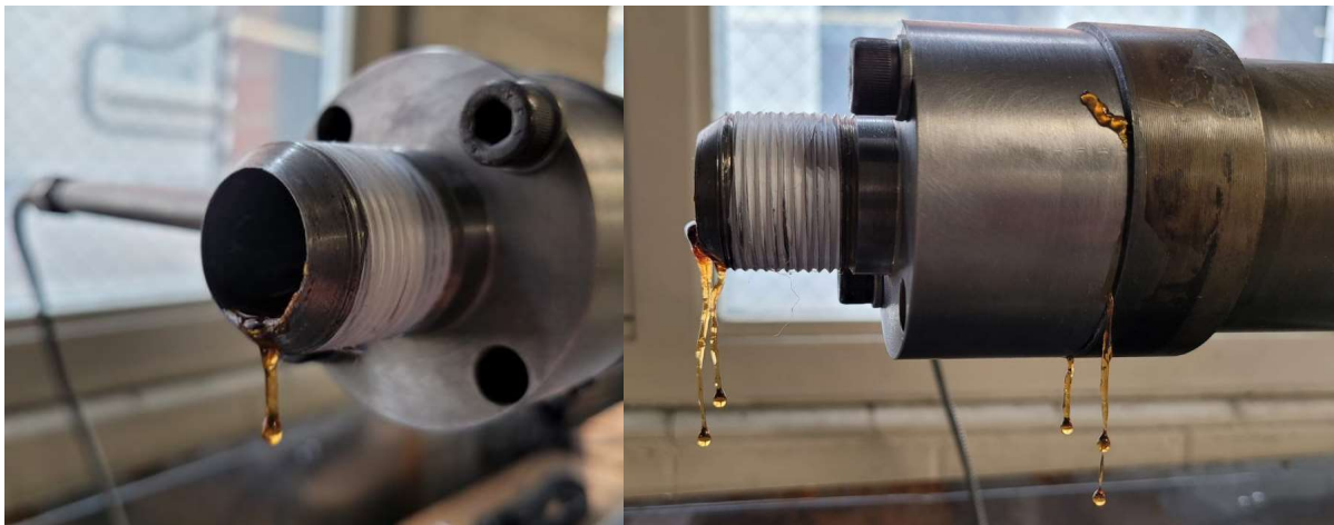
Figure 6-7: Sodium silicate and water mix leaking from die.
