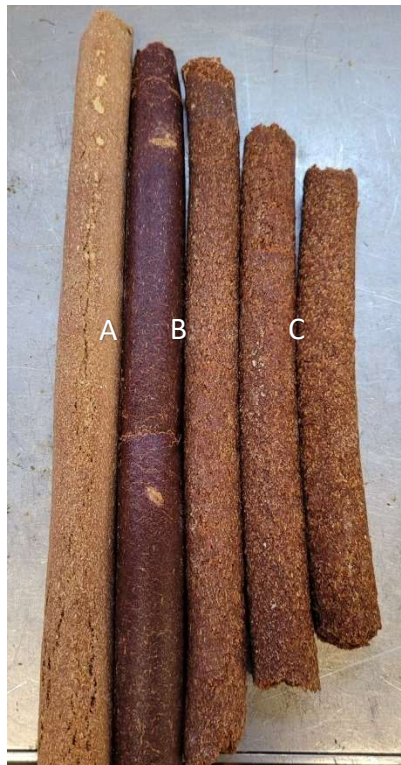
Figure 6-5: (A) Fresh extrudate. (B) Extrudate held at room temperature. (C) Extrudate stored in freezer.
