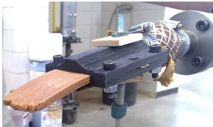
Figure 3-21: Successful rectangular extrusion.
