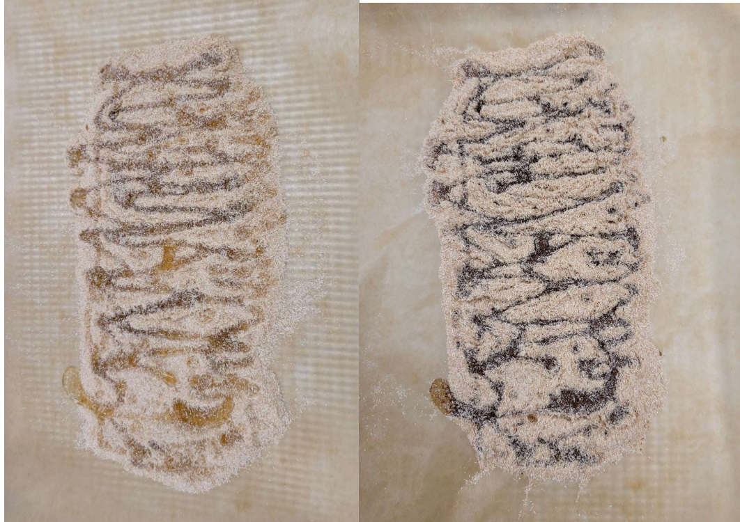
Figure 5-4: (Left) Pour-over mixing before curing. (Right) After curing.
