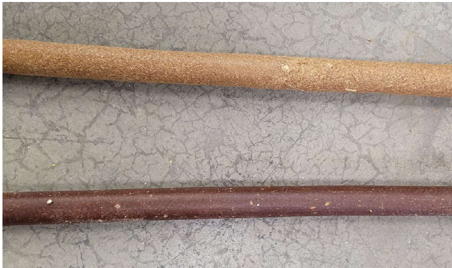
Figure 3-29: (Top) Extrudate at room temp. (Bottom) Extrudate at 52.5^{\circ}\text{C} .
