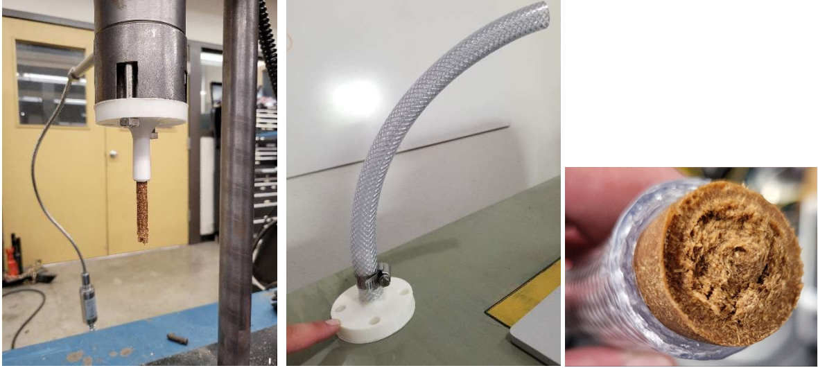
Figure 3-5: (Left) Extrudate coming out of hose attachment bolted to die. (Middle) 300psi clear reinforced hose. (Right) extruded material leaving exit of reinforced hose.
