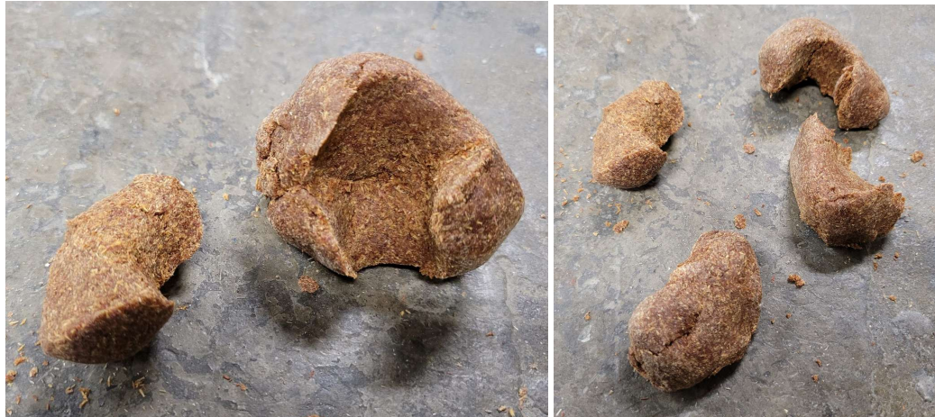
Figure 6-13: (Left) Segment separates at boundary layer. (Right) All four sections of extrudate separated.
