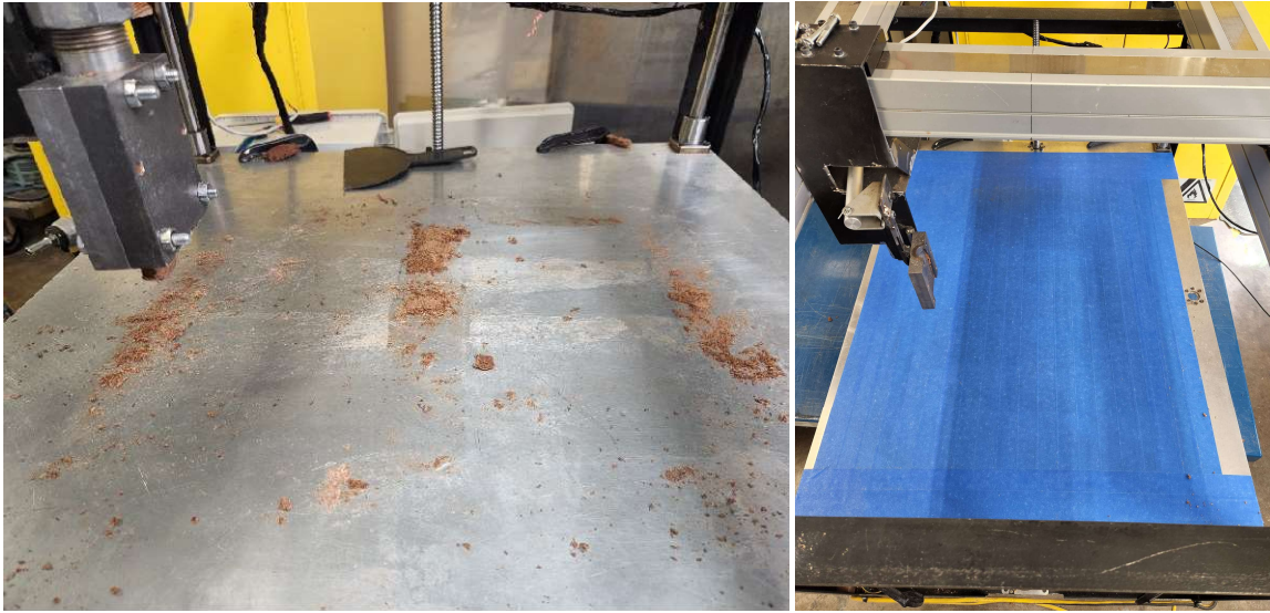
Figure 5-12: (Left) Printed Extrudate left on aluminum bed. (Right) Blue painters tape applied to bed surface.
