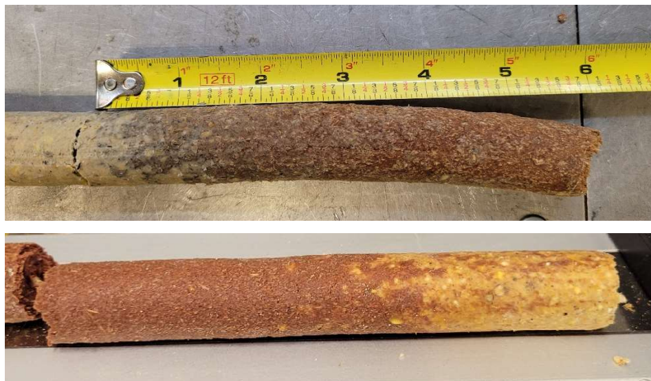
Figure 3-15: Transition zone between the sodium silicate and scratch grains.
