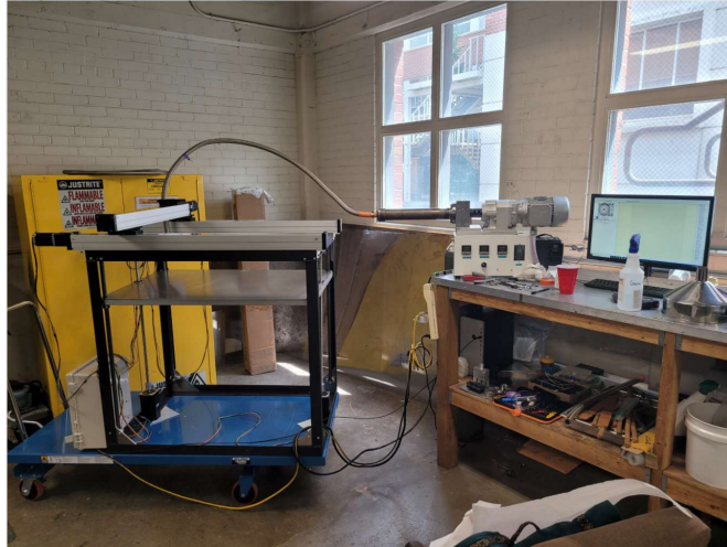
Figure 3-14: 3D printer and extruder height problem.
