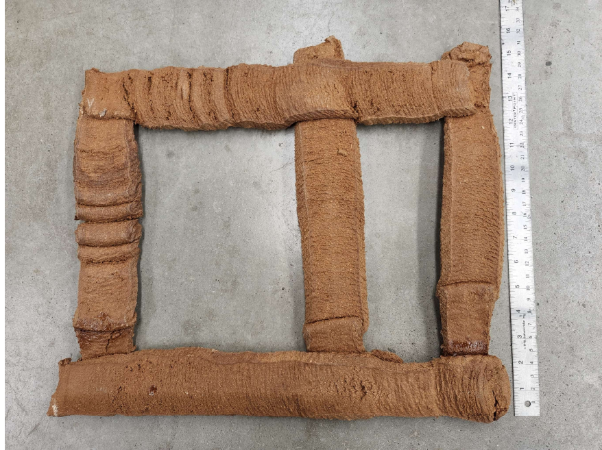
Figure 6-17: 3D printed material in both X and Y directions.
