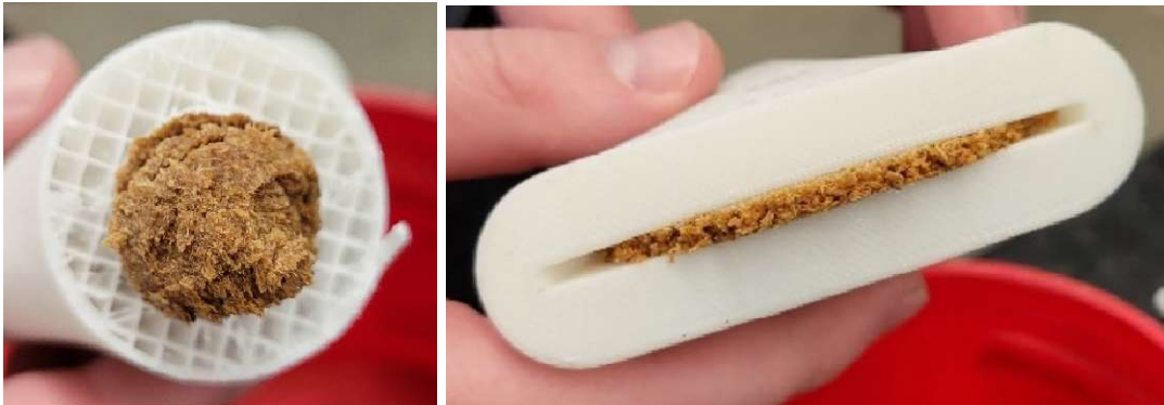
Figure 3-19: (Left) Nozzle filled with material at failure. (Right) Deformed material at exit of nozzle.
