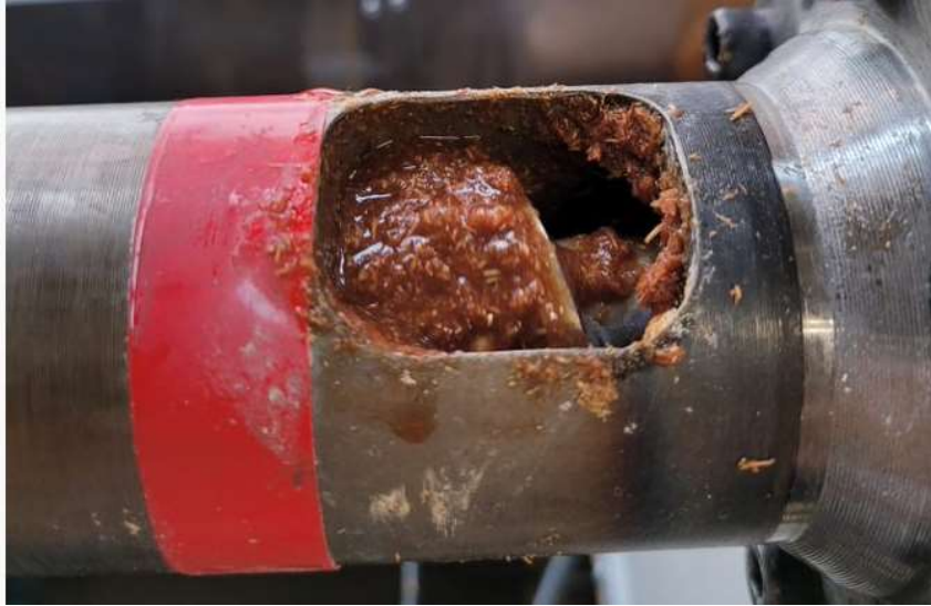
Figure 6-6: Water added to mixture unable to extrude.
