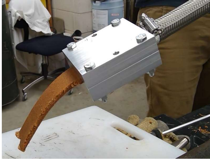
Figure 3-24: V3 nozzle with rectangular extrudate.
