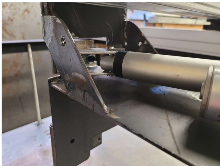
Figure 3-34: Added gussets to bracket to support larger actuator.
