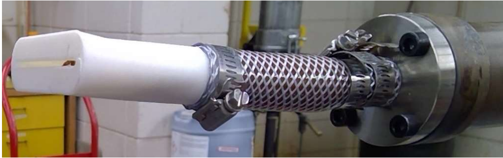
Figure 3-18: Nozzle, hose, and die attached together with hose clamps.
