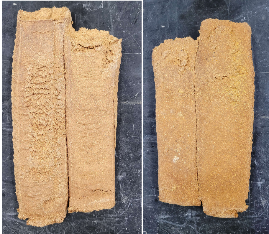
Figure 6-18: Side-by-side layering of WSSC with interlayer adhesion. (Left) Top. (Right) Bottom.
