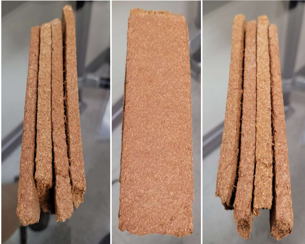
Figure 6-15: Layers separate during curing.
