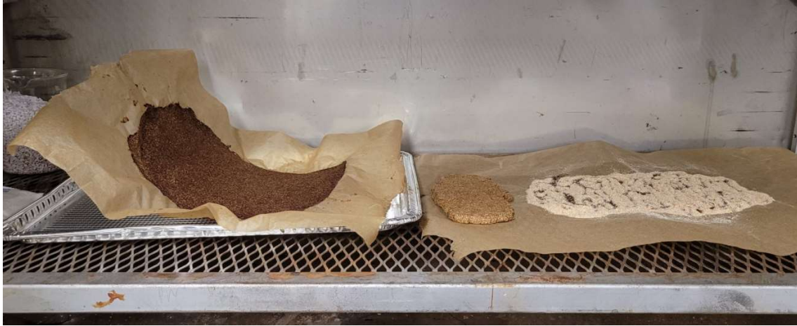
Figure 6-8: (Left) Liquid mixture (Center) Hand Mixed (Right) Binder Jetting
