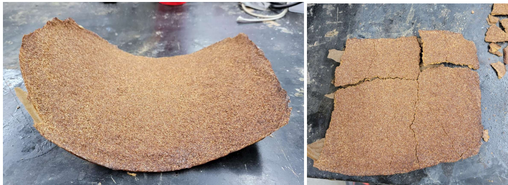
Figure 6-9: (Left) Cured mixture with water added. (Right) Broken wood composite.
