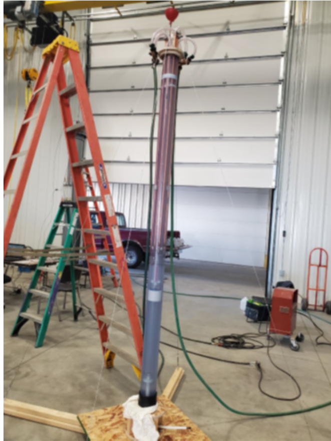
Figure 3.30: Photograph of the Ohmic Heated "clear vessel". The heat sink can be seen in the upper half of the assembly as copper piping. The lower portion of the tube column contains the ohmic heat source electrodes. The WHIP is not present in this configuration. Courtesy of Kristen Geddes, Graduate Student at University of Idaho, Nuclear Engineering.
