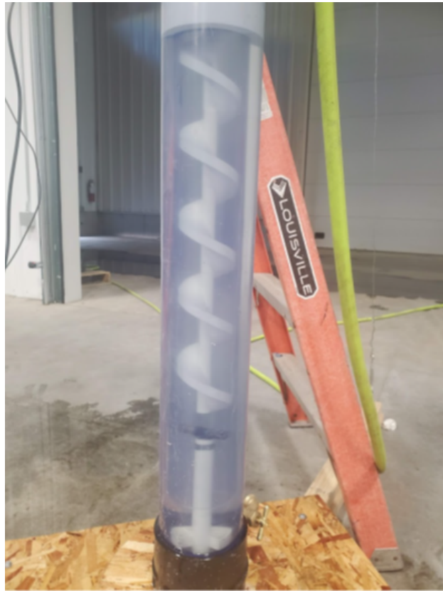
Figure 3.31: Photograph of the Ohmic Heated "clear vessel" with the 5-pitch WHIP installed. Courtesy of Kristen Geddes, Graduate Student at University of Idaho, Nuclear Engineering.
