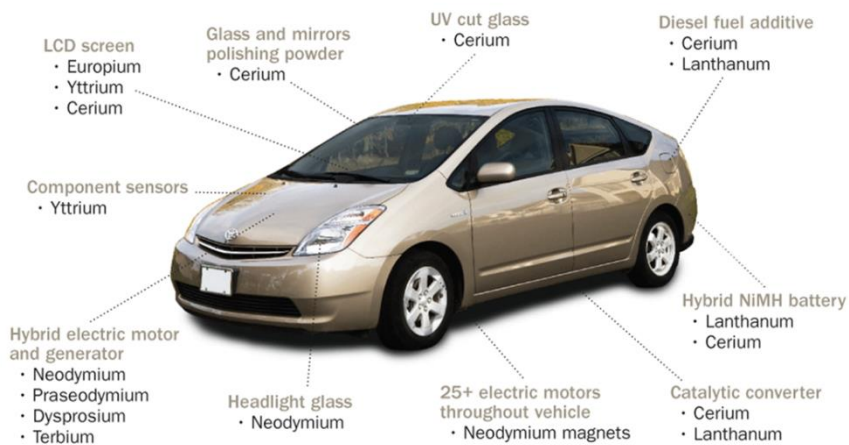
Figure 3: Extent of REE usage in hybrid vehicles [5].
