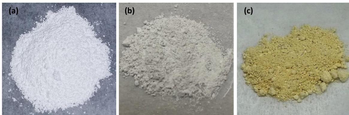
**Figure 4-17.** (a) non-treated phosphor (b) phosphor sonicated with H<sub>2</sub>O at 80°C for 1 hour (c) phosphor sonicated with NaOH at 80°C for 1 hour
