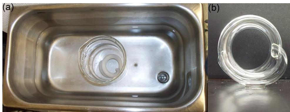
**Figure 2-1.** Ultrasound-assisted collection of rare earth phosphors from used compact fluorescent lamps. (a) Sonication bath (42kHz 100 watt) with a compact fluorescent lamp, (b) the lamp after 30 seconds of sonication and rinsing.
