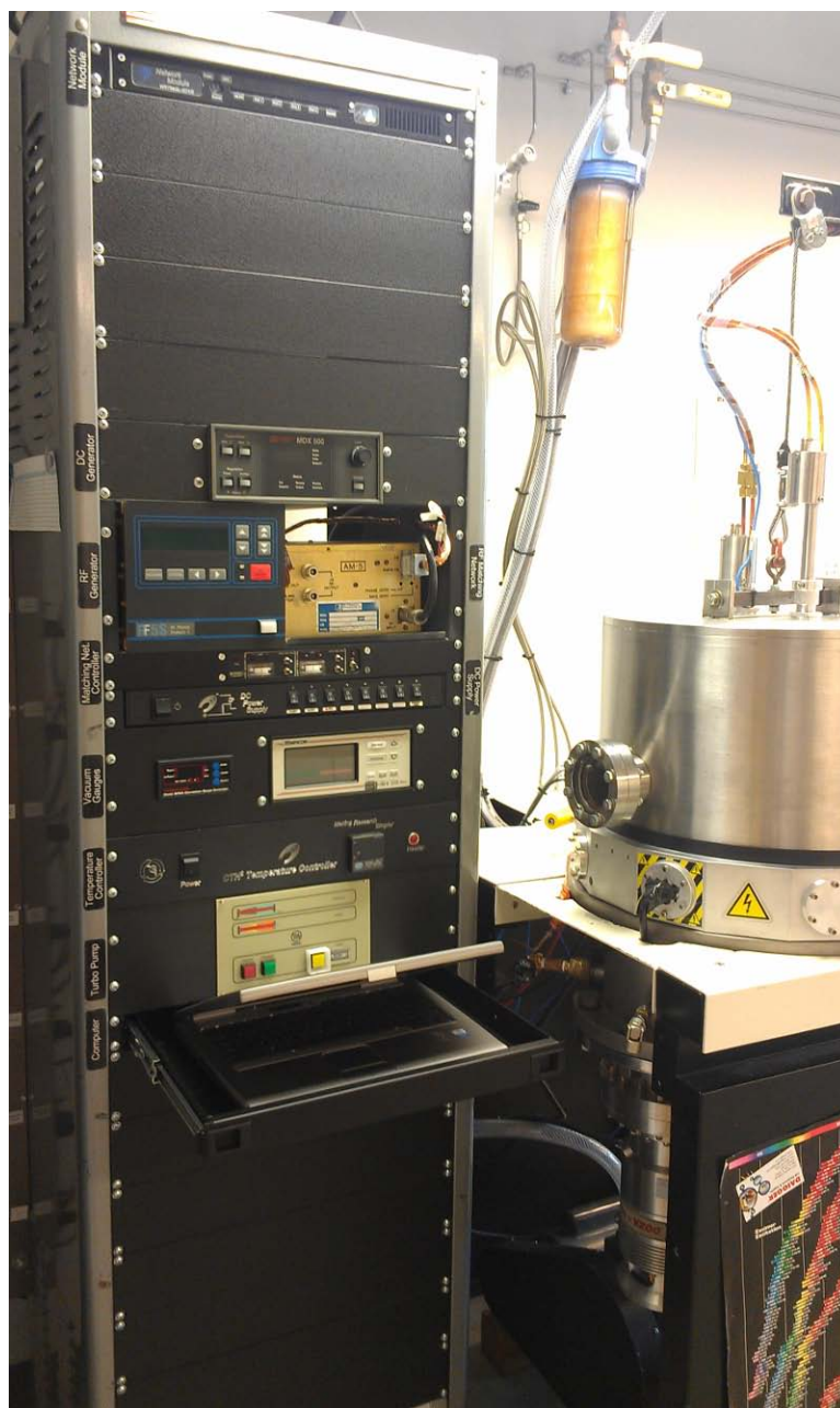
Figure 2.4: A photograph of the sputtering system utilized in this work. On the right is the growth chamber and underneath is the turbo molecular vacuum pump backed up by the mechanical roughing pump. On the left is the equipment rack with all the accompanying control electronics and power sources.
