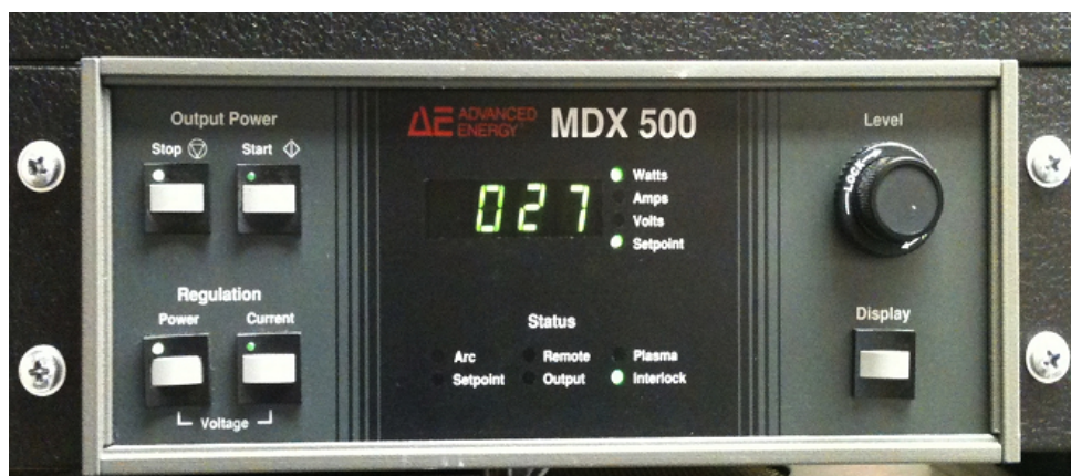
Figure 2.6: The MDX 500 DC generator used in this work for the creation of ZnO and Mg x Zn 1-x O thin films. It has a capability of delivering 500W of power to the sputtering target and has a built-in arc suppression circuitry.
