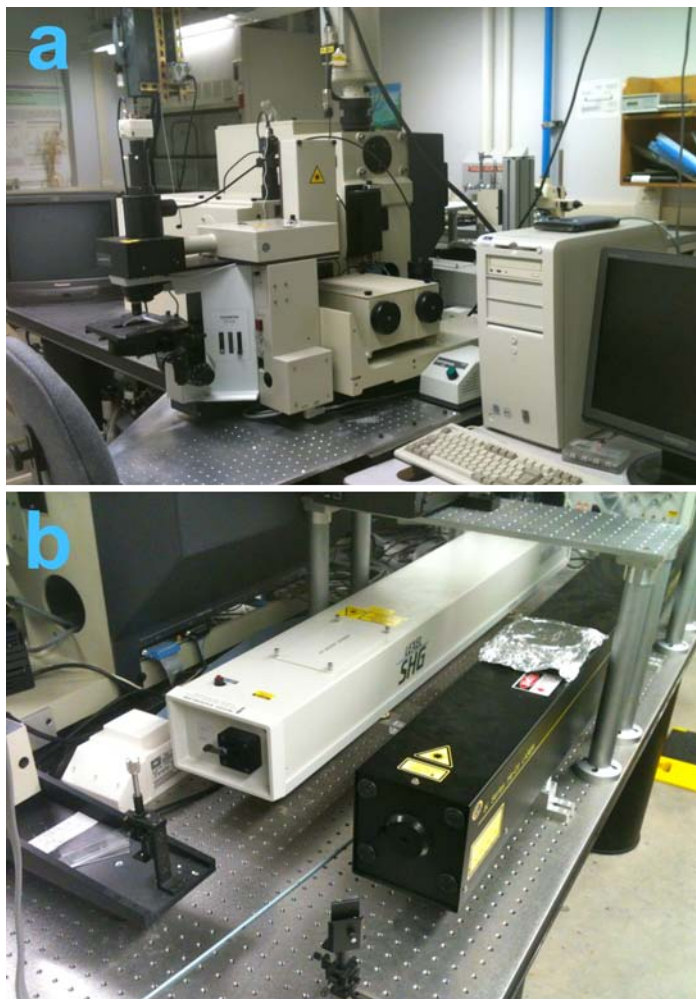
Figure 2.19: The equipment configuration in this work. a) The JobinYvon/Horiba T64000 Photoluminescence/Raman system and b) the Kimmon He-Cd laser of 325 nm (at right) and the Lexel SHG frequency doubled argon ion laser operating at 244 nm (at left).
