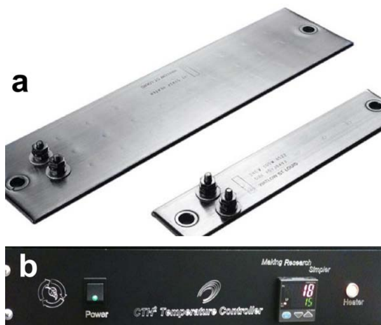
Figure 2.8: a) The Watlow stainless steel strip heaters used for substrate heating and b) the custom built temperature controller based around a Yokogawa UT-150 PID controller. Such a system is capable for controlling the temperature of substrates tightly from room temperature to 780 °C.
