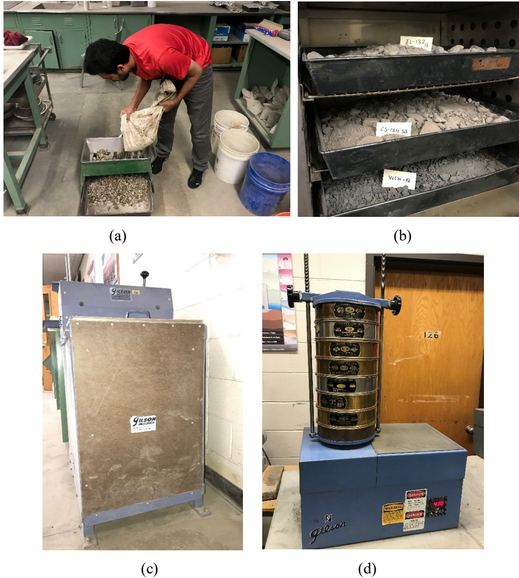
Figure 3.2 Grain size distribution of the aggregates. (a) splitting the materials, (b) drying materials in the oven, (c) using the large sieve shaker, and (d) using the small sieve shaker
