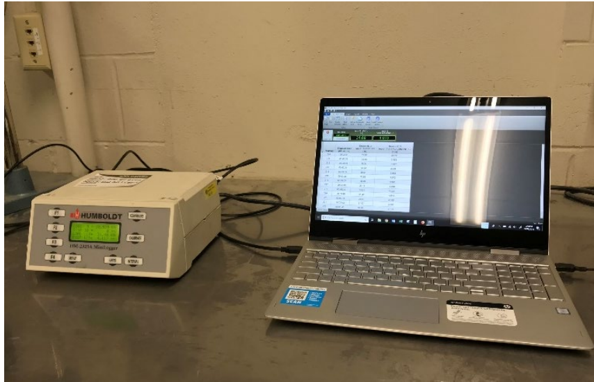
Figure 3.15 Data acquisition system for the CBR testing
