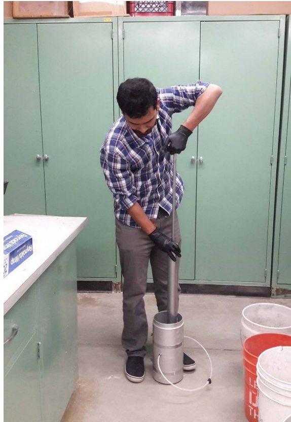
Figure 3.10 Compaction of specimen for resilient modulus
