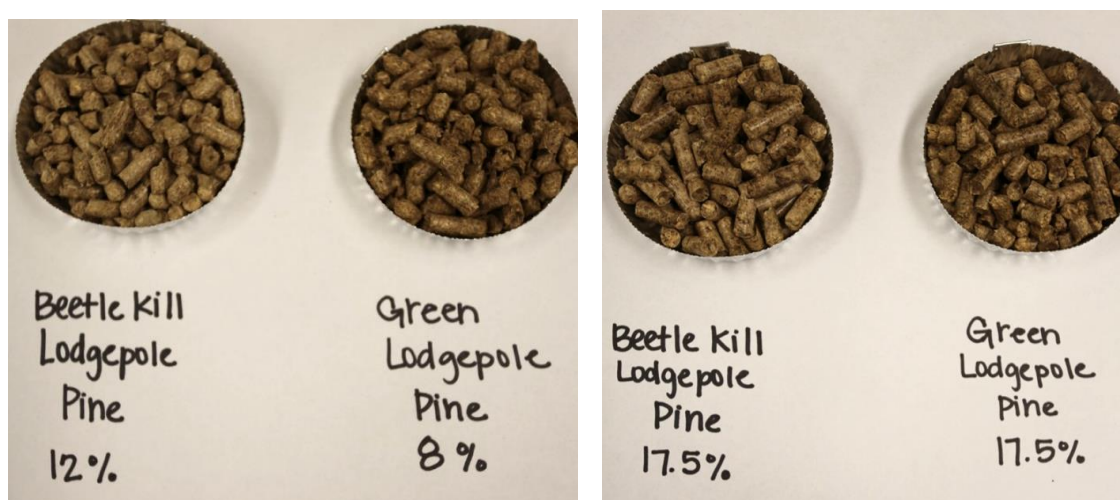
Figure 2.9. Pellets from both residue types, produced on the portable mill (left) and the laboratory mill (right) with varying MC.
