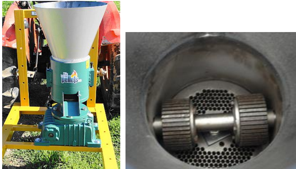
Figure 2.3. Make Your Own Pellets, LLC., portable PTO driven, flat die pellet mill (Make Your Own Pellets, LLC, 2014).
