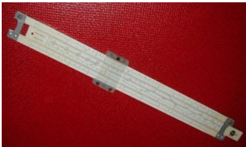
Figure 8.3 The slide ruler; the basic tool of engineers, was invented in 1622 ( Wikipedia 2022 )
