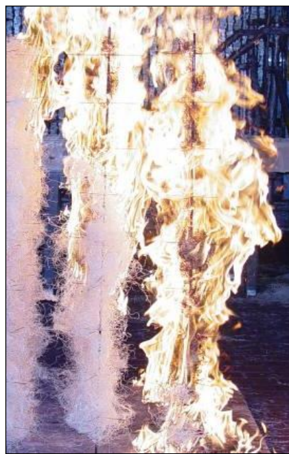
Fig. 2.2 This experimental fire is spreading from right to left through a 1.2 m deep (vertical length) fine excelsior fuel bed (shredded Populus spp. ). Observations revealed the ignition of adjoining fuels without significant pre-ignition pyrolysate emissions (clear gaps) and only after flame contact. (photograph by Jack Cohen, US Forest Service)
