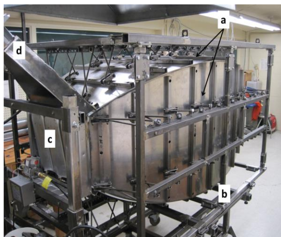
Fig. 4.2 This is the radiant panel (c) and the mirror assembly (a). The mirror assembly is supported by the shaping frame and support carriage (b). The gas fired radiant is panel (c) is vented through the exhaust duct (d).
