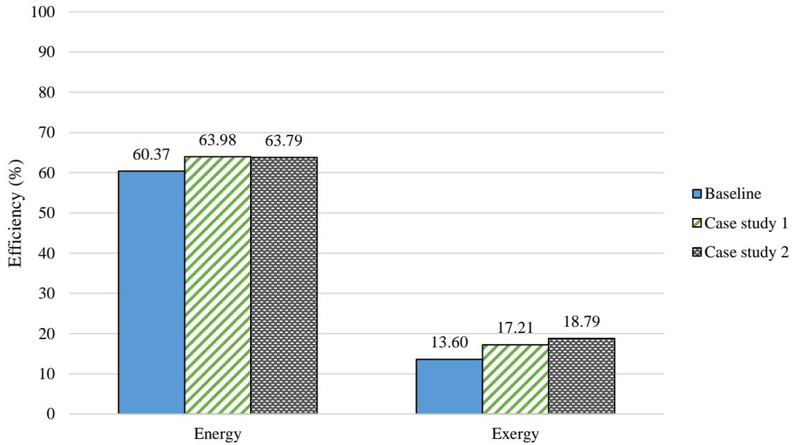
**Figure 4.6. Average system energy and exergy efficiency with a single effect chiller for July.**
