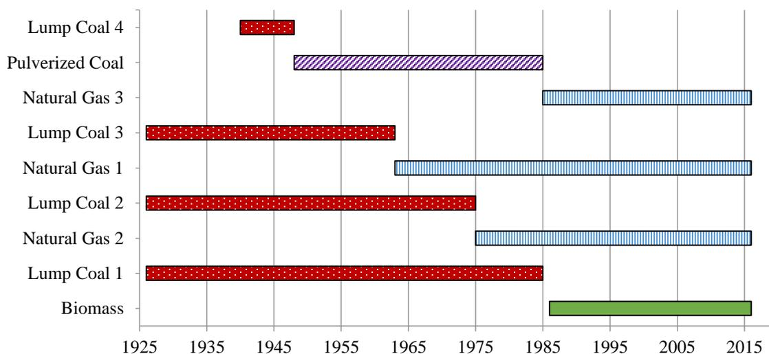
**Figure 2.5. Timeline of boiler evolution at the UI district energy plant from 1926 to 2016.**
