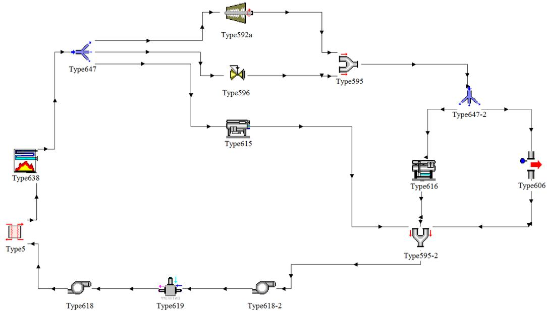
**Figure 4.1. Graphical representation of the UI energy plant in TRNSYS including steam turbine and double effect absorption chiller.**
