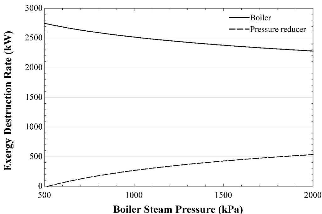
Figure 3.5. Exergy destruction rate vs steam pressure level through the boiler.
