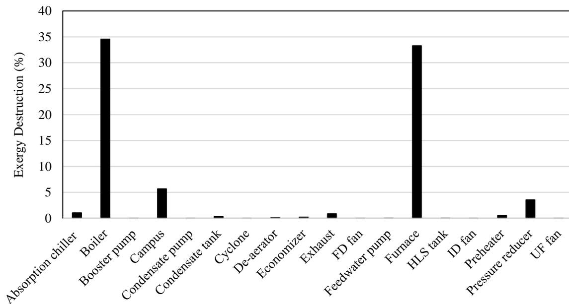
**Figure 3.4. Percentage of exergy destroyed in each component relative to exergy input with fuel.**
