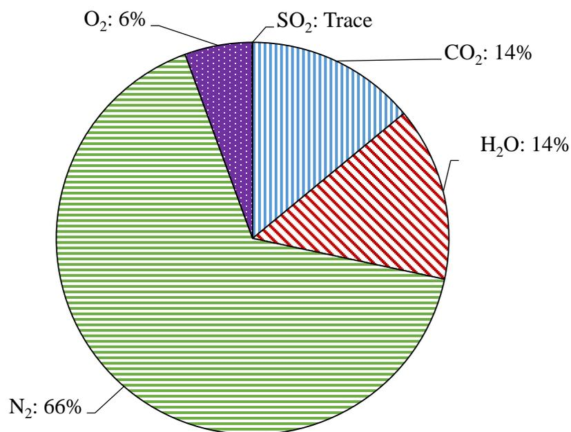
**Figure 2.9. Molar composition of actual biomass combustion products by volume.**
