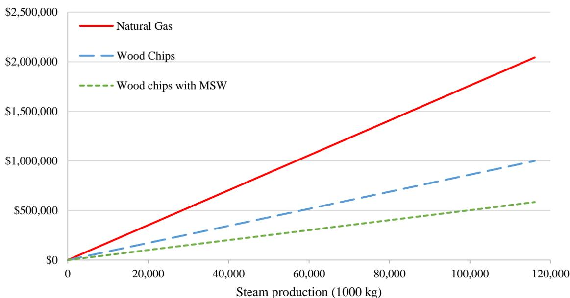
Figure 5.5. Fuel costs versus steam production for each fuel type.
