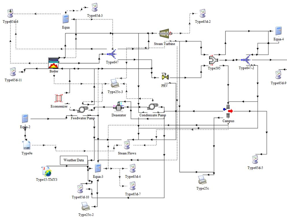
**Figure A3.3. Full graphical representation of TRNSYS model for case studies 5 and 6.**
