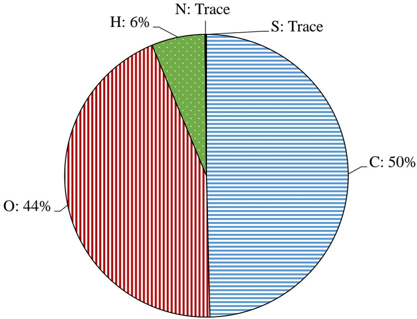
Figure 2.4. Chemical composition of bone dry wood by weight.
