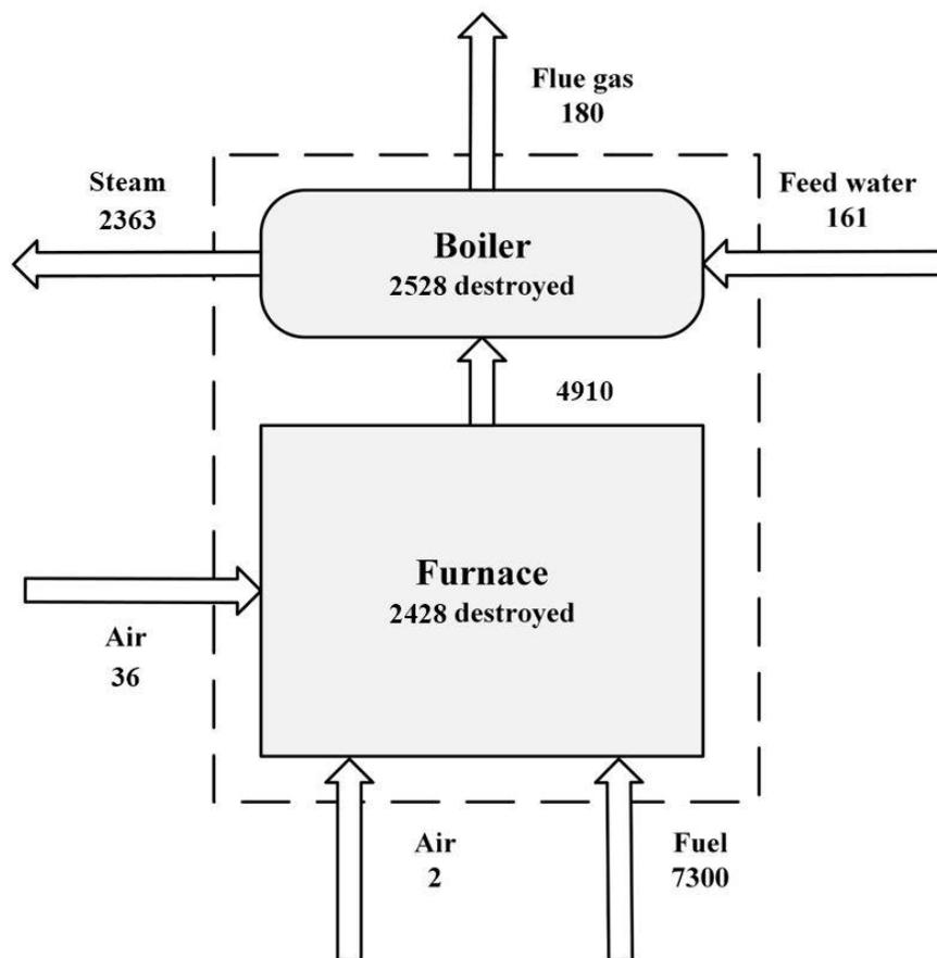
Figure 3.2. Exergy flow and destruction rates (in kW) for the biomass boiler and furnace.
