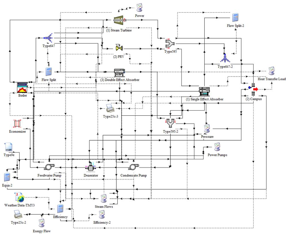
Figure A3.2. Full graphical representation of TRNSYS model for case studies 3 and 4.
