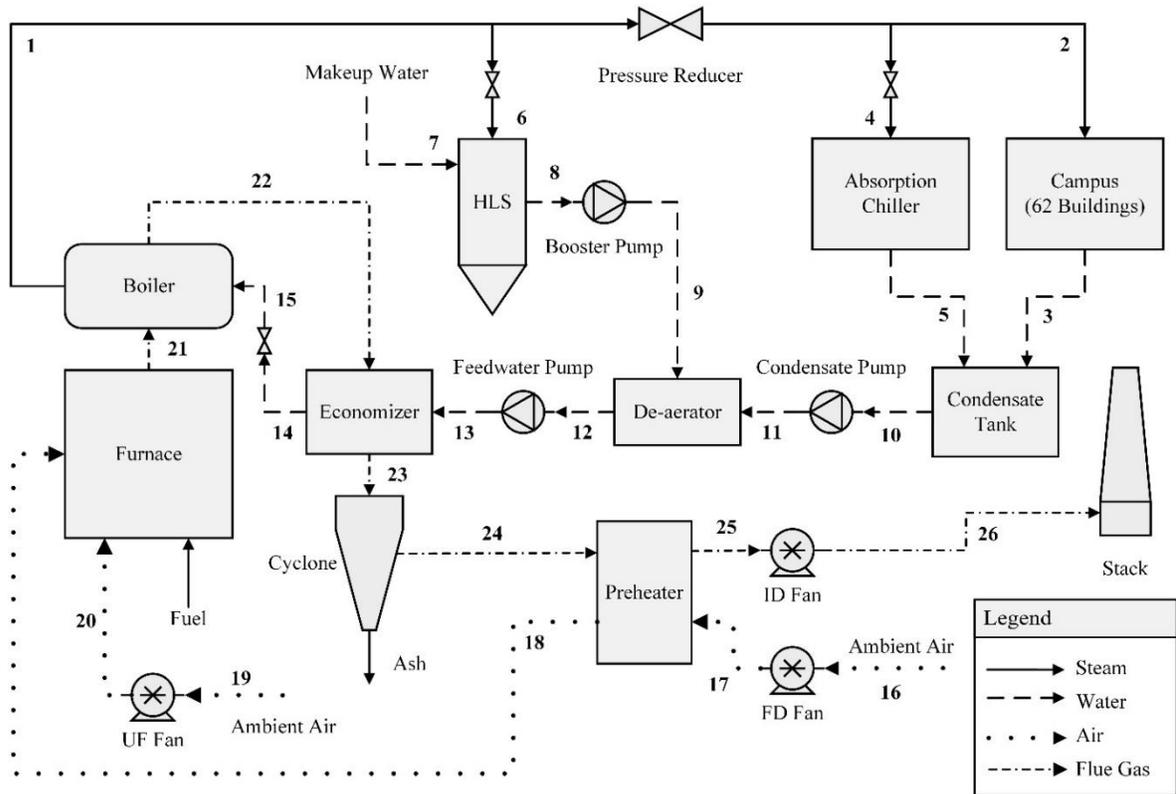
Figure 3.1. Flow diagram of the steam cycle including the biomass boiler.
