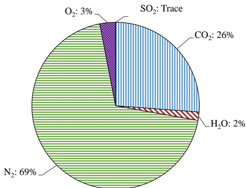
**Figure 2.7. Molar composition of bone dry biomass combustion products by volume using the combustion model.**
