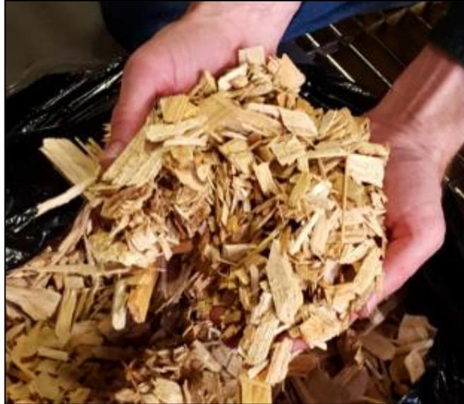
**Figure 2.3. Wood chip fuel comprised of western red cedar. Photo courtesy of UI district energy plant.**
