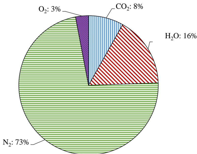
**Figure 2.8. Molar composition of natural gas combustion products by volume.**
