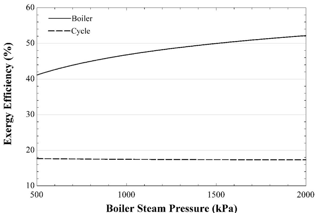
**Figure 3.6. Exergy efficiency of boiler and cycle vs steam pressure in the boiler.**
