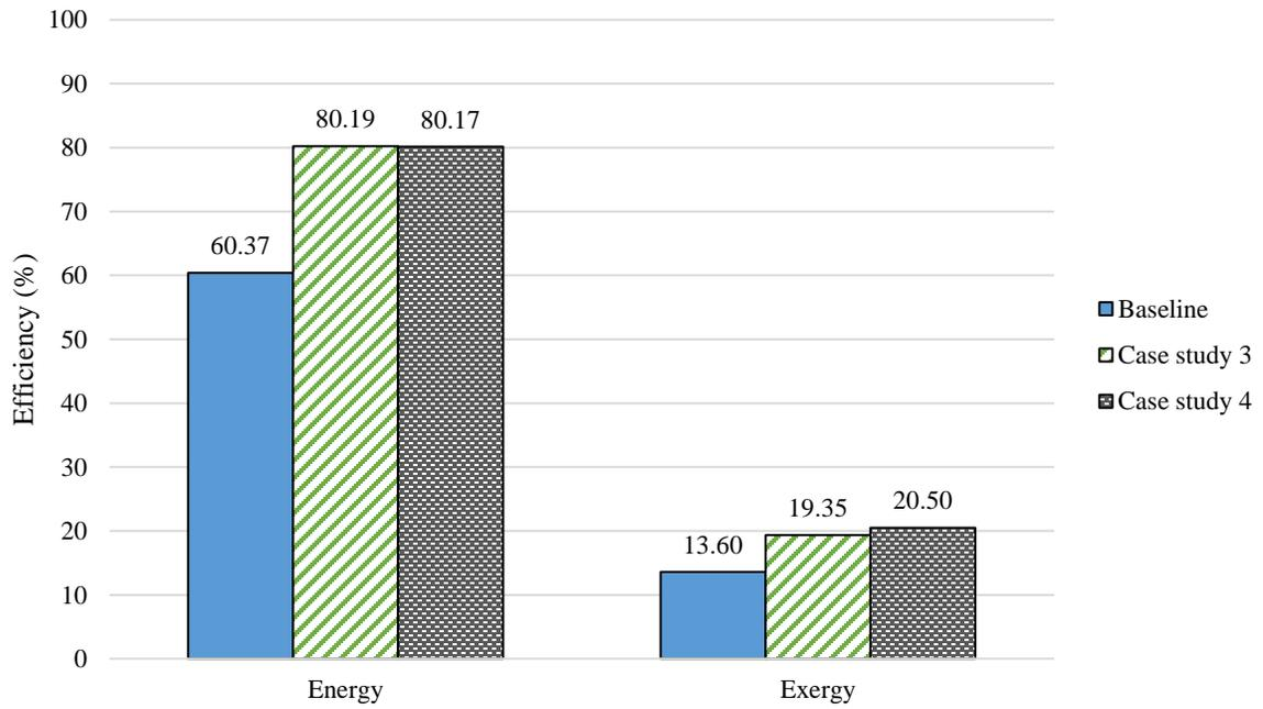
**Figure 4.7. Average system energy and exergy efficiency with single and double effect chillers for July.**
