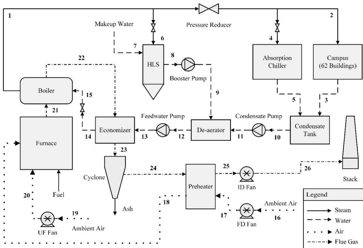
**Figure 4.2. Flow diagram of the current UI steam cycle including the biomass boiler and single effect absorption chiller.**
