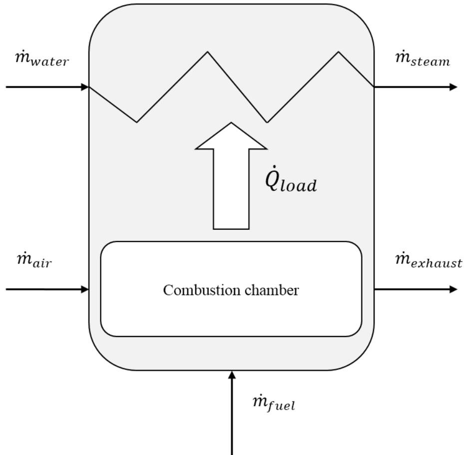
**Figure 2.6. Flow conditions through each boiler.**
