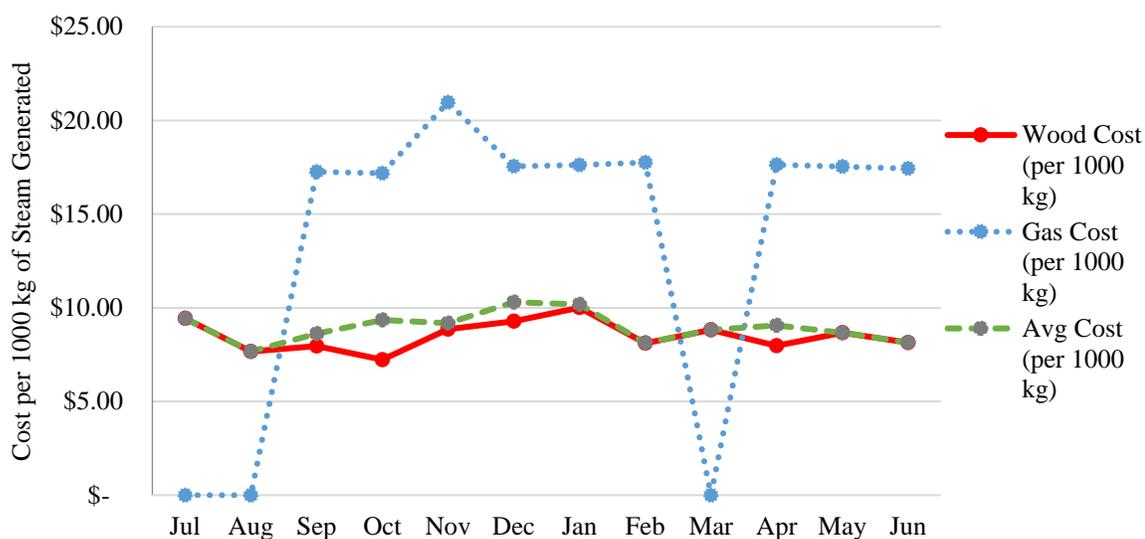
**Figure 2.10. Monthly costs of steam produced for FY15.**
