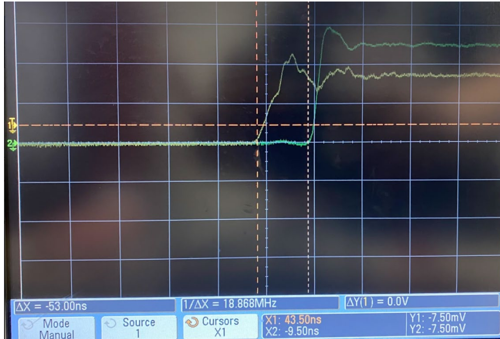
Figure 6.7 Fiber Optic TX and RX PCB Implementation with a 53 Nanosecond Delay ( \Delta X )
