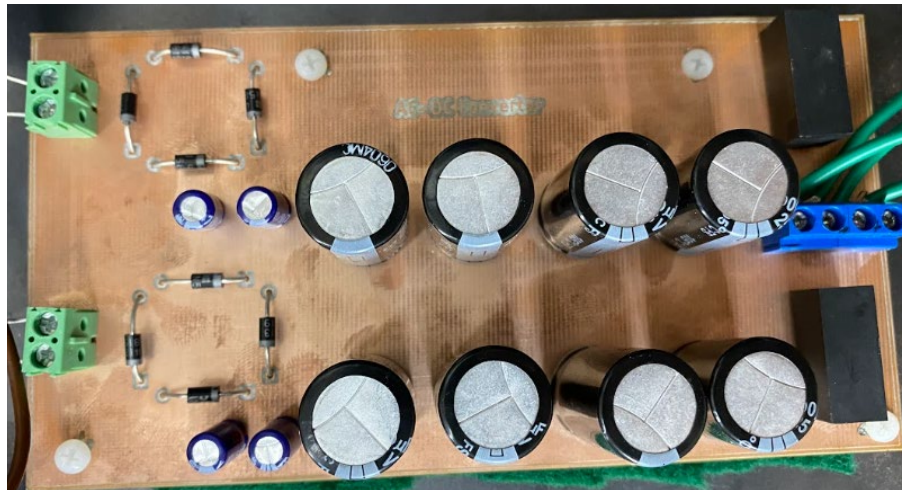
Figure 3.7 AC-DC Converter PCB
