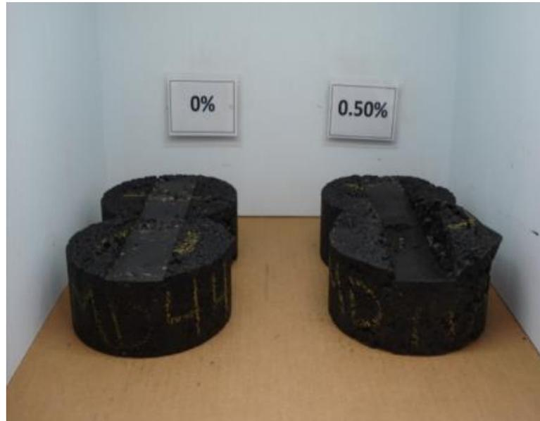
**Figure 2.10:** Hamburg Samples with PG 64-28 “Original Formulation” (DeVol, 2016)
