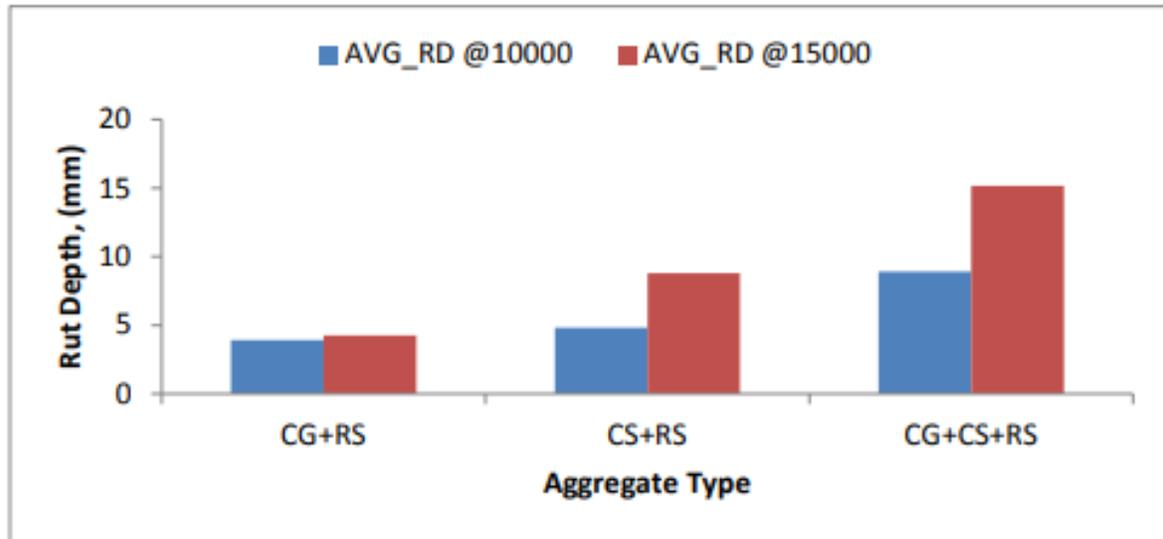
**Figure 2.17:** Effect of Aggregate Type on Hamburg Rutting Depth (Rahman and Hossain, 2014)
