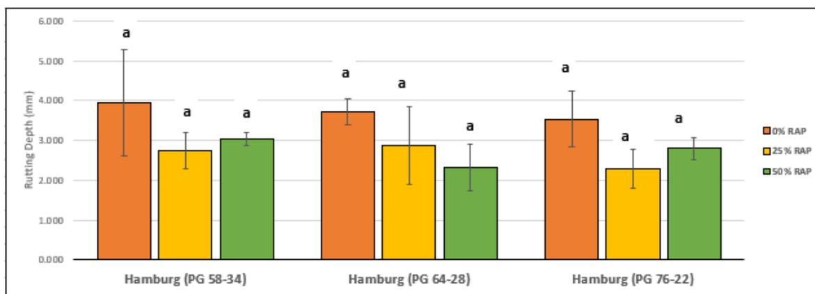
**Figure 4.8:** Comparison of Hamburg Rutting with Different Binder Grades at 5.0% Binder Content
