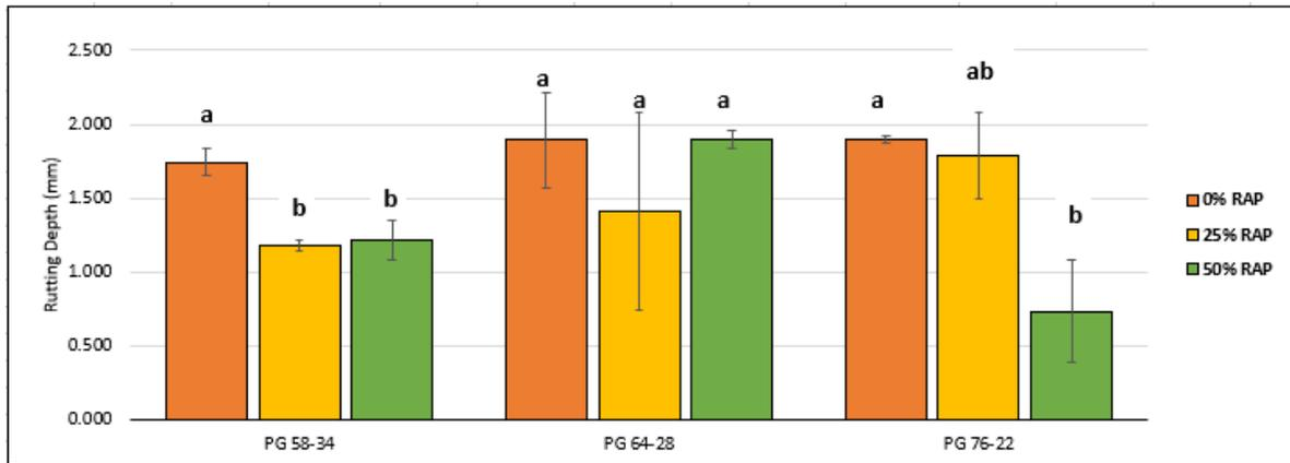
**Figure 4.6:** Comparison of APA Rutting with Different Binder Grades at 5.00% Binder Content
