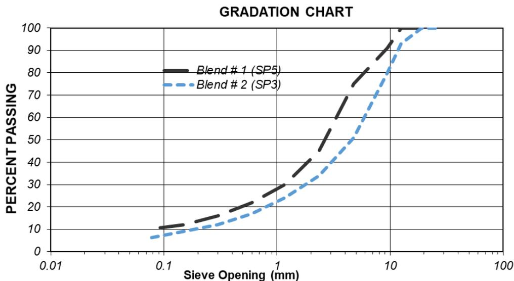
**Figure 3.3:** LMLC Aggregate Gradation (SP3 & SP5)
