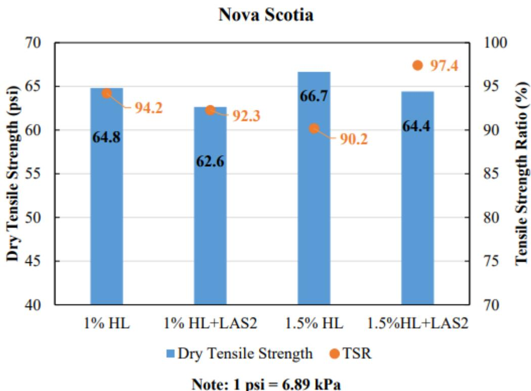
**Figure 2.28:** TSR Test Results for Nova Scotia FC-5 Asphalt Mixtures (Gu et al., 2020)
