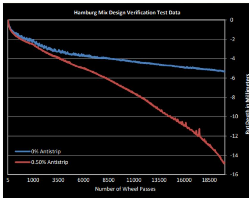
**Figure 2.11:** Graph of Rutting Depth for PG 64-28 Hamburg Samples (DeVol, 2016)
