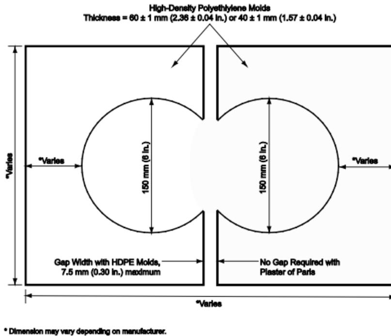
**Figure 2.3:** Dimensions of Hamburg Samples (AASHTO T324-16, 2016)
