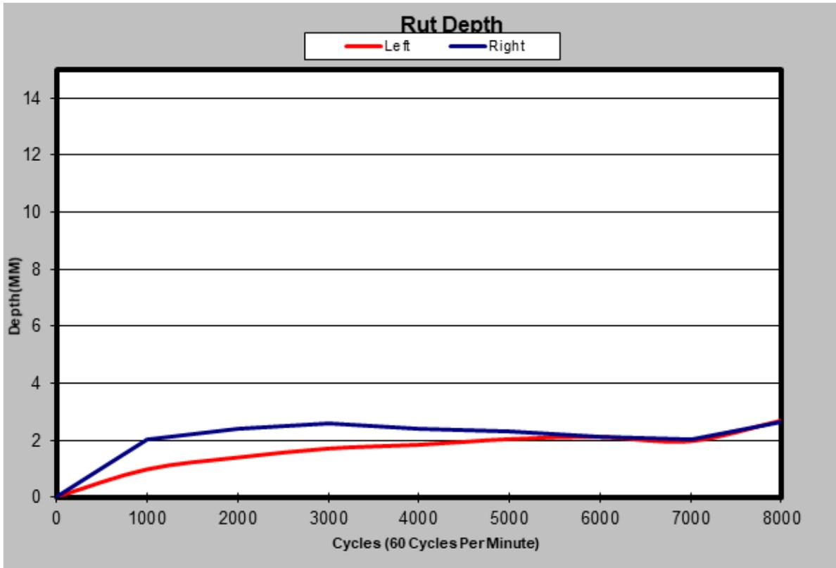
**Figure 9B:** APA Rutting Data Sample @ PG 76-22, 50% RAP and 5.75% B.C.
