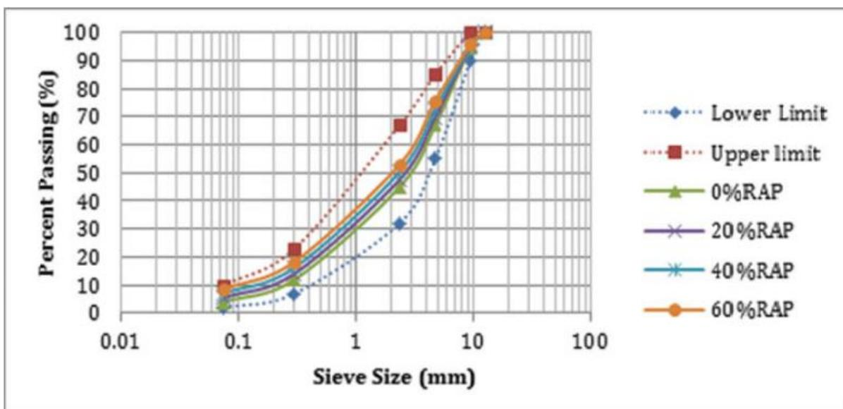
**Figure 2.15:** Gradations of Designated Aggregate and RAP sources (Alireza et al., 2016)
