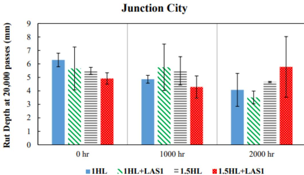
**Figure 2.29:** Rut Depth of Junction City FC-5 Asphalt Mixtures after 20,000 Passes (Gu et al., 2020)
