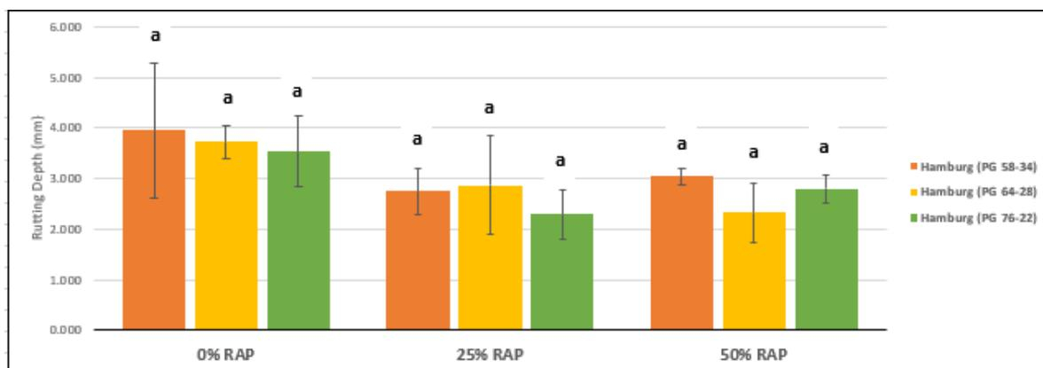
**Figure 4.12:** Hamburg Comparison of RAP Percentage at Different Binder Grades at 5.0% Binder Content
