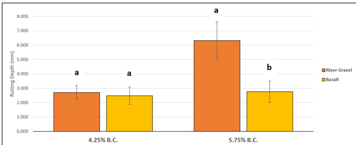
**Figure 4.31:** Effect of Aggregate Type on HWTT Results
