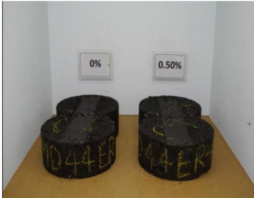
**Figure 2.12:** Hamburg Samples with PG 64-28 “Polymer Modified” (DeVol, 2016)
