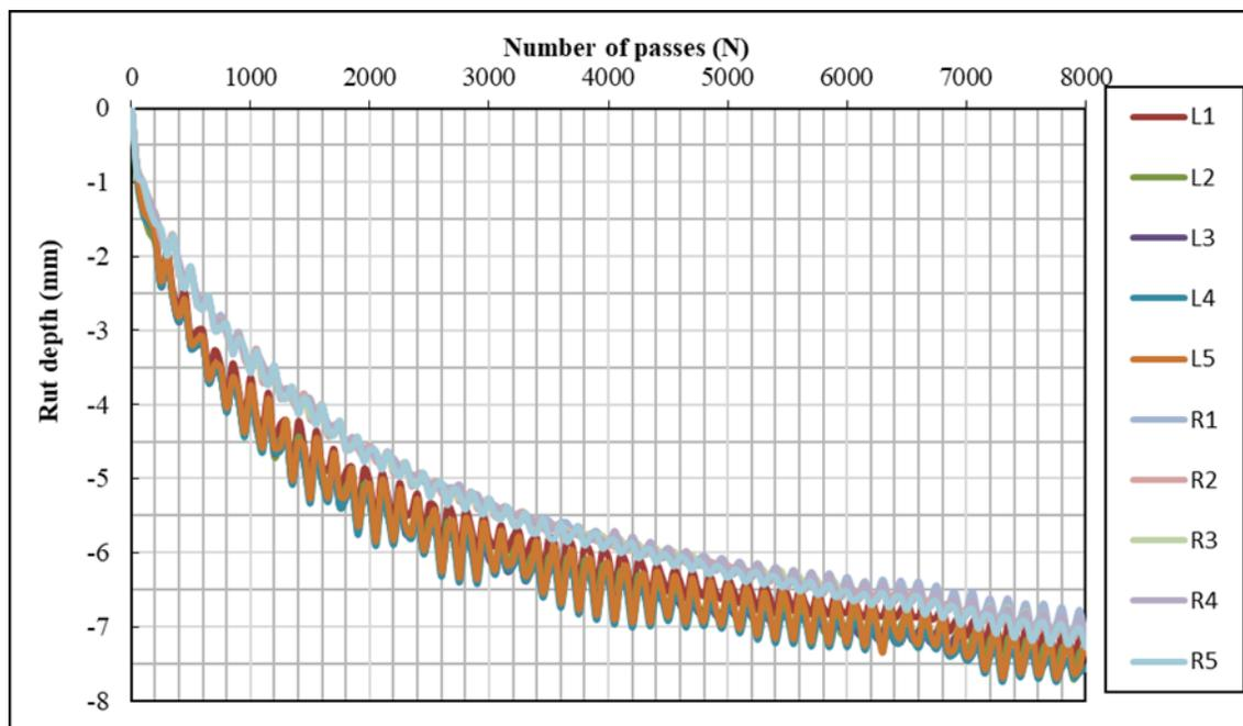
**Figure 3.5:** APA Rut Test, Left & Right (L1-L5, R1-R5) Wheel Deformation Measurement
