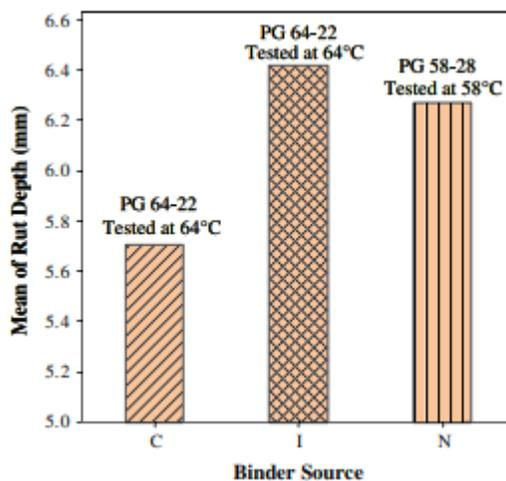
**Figure 2.26:** Binder Source Effects on Rutting Performance (Zhao et al., 2012)
