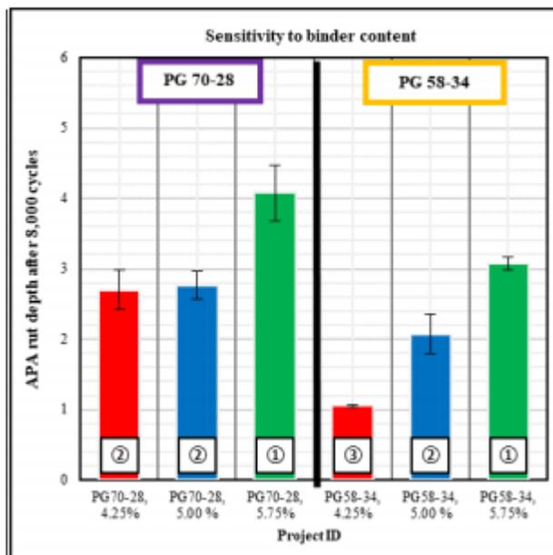
**Figure 2.25:** Sensitivity of APA Rut Depth at 8,000 Cycle to Binder Content (Kassem et al., 2019)
