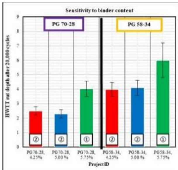
**Figure 2.24:** Sensitivity of HWTT Rut Depth after 20,000 passes to Binder Content (Kassem et al., 2019)
