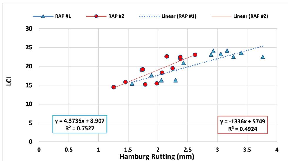
**Figure 4.26:** Correlation between LCI and HWTT Rut Depth at Different RAP Sources
