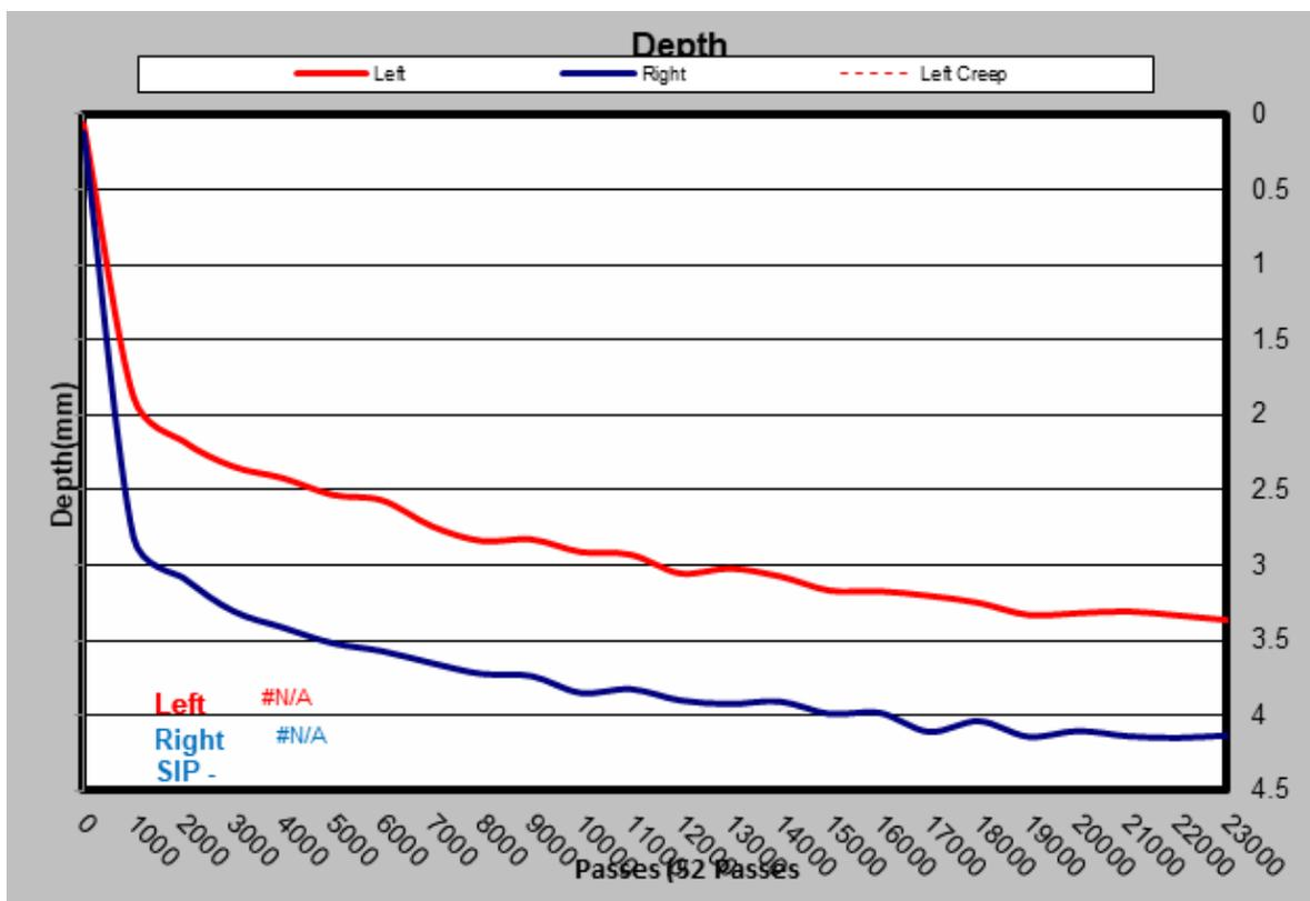
**Figure 12B:** Hamburg Rutting Data Sample @ PG 58-34, 50% RAP and 5.75% B.C.
