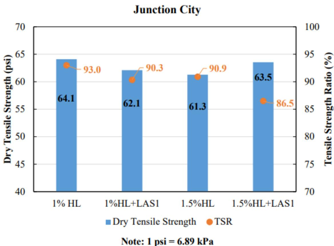
**Figure 2.27:** TSR Test Results for Junction City FC-5 Asphalt Mixtures (Gu et al., 2020)
