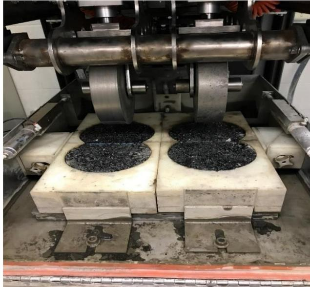
**Figure 2.2:** Hamburg setup inside the Asphalt Pavement Analyzer Jr.
