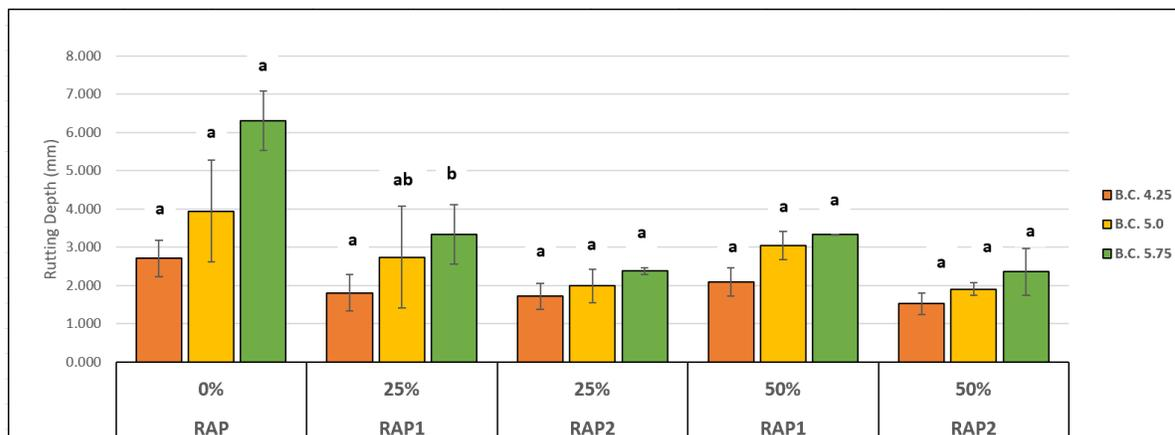
**Figure 4.2:** HWTT Rut Depth at Different Binder and RAP Contents
