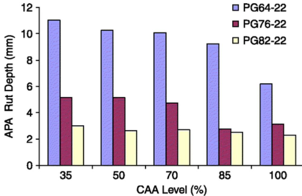
**Figure 2.22:** APA Rut Depths of HMA Mixtures (Baoshan et al., 2009)
