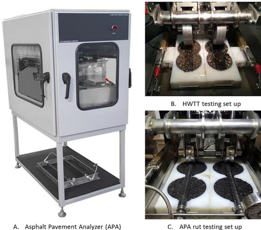
**Figure 3.4:** APA and HWTT Rutting Test in the Asphalt Pavement Analyzer (APA)
