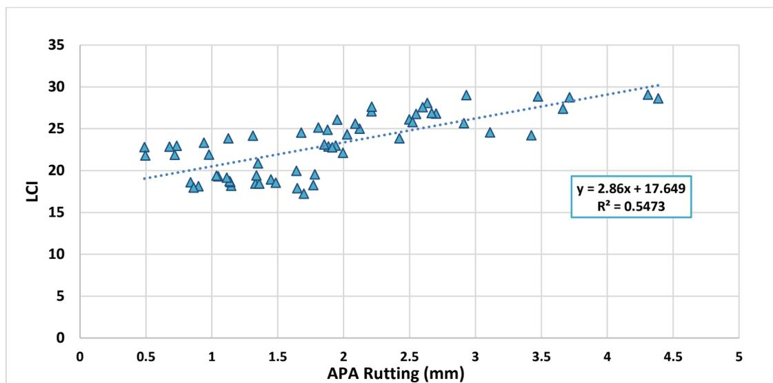
**Figure 4.20:** Correlation between LCI and APA Rut Depth for LMLC Mixes
