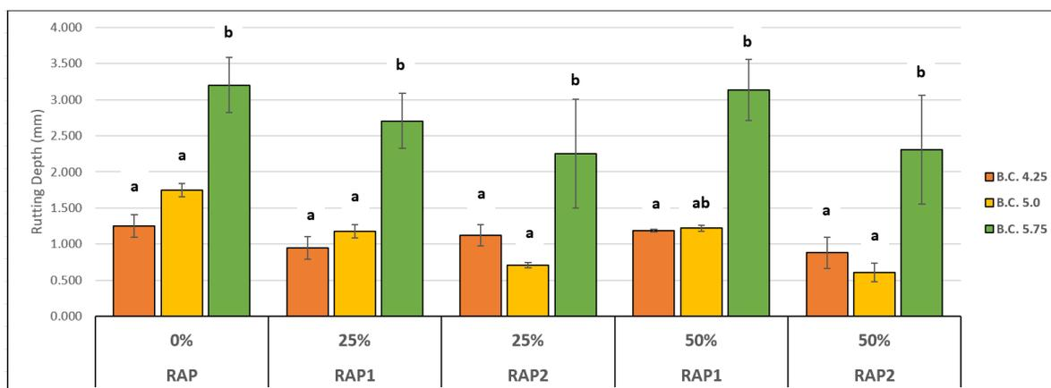
**Figure 4.1:** APA Rut Depth at Different Binder Contents for PG 58-34 Mixtures
