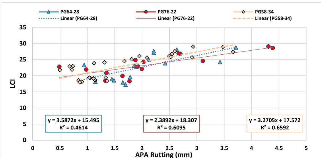
**Figure 4.21:** Correlation between LCI and APA Rut Depth at Different Binder Grades
