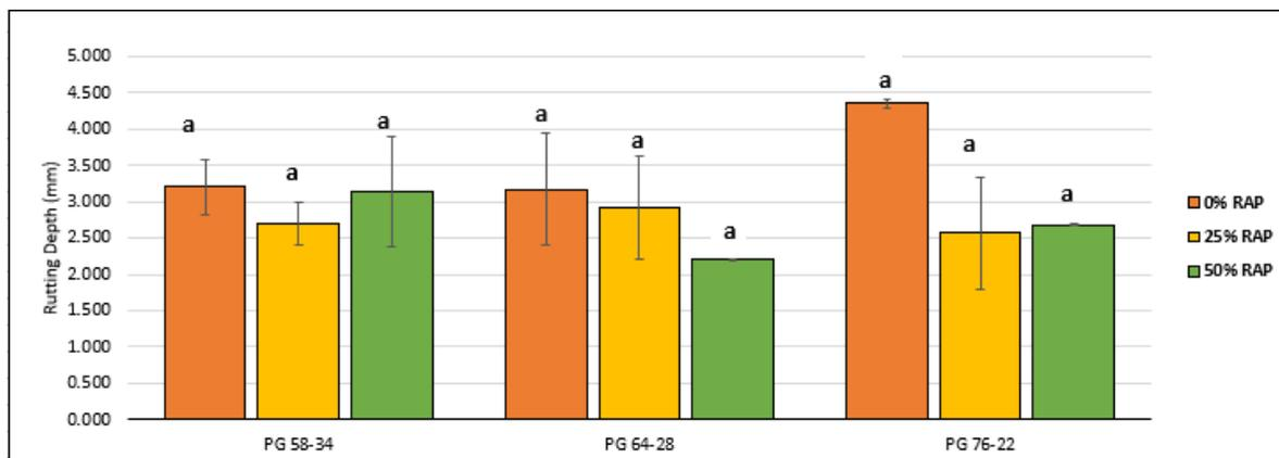
**Figure 4.7:** Comparison of APA Rutting with Different Binder Grades at 5.75% Binder Content
