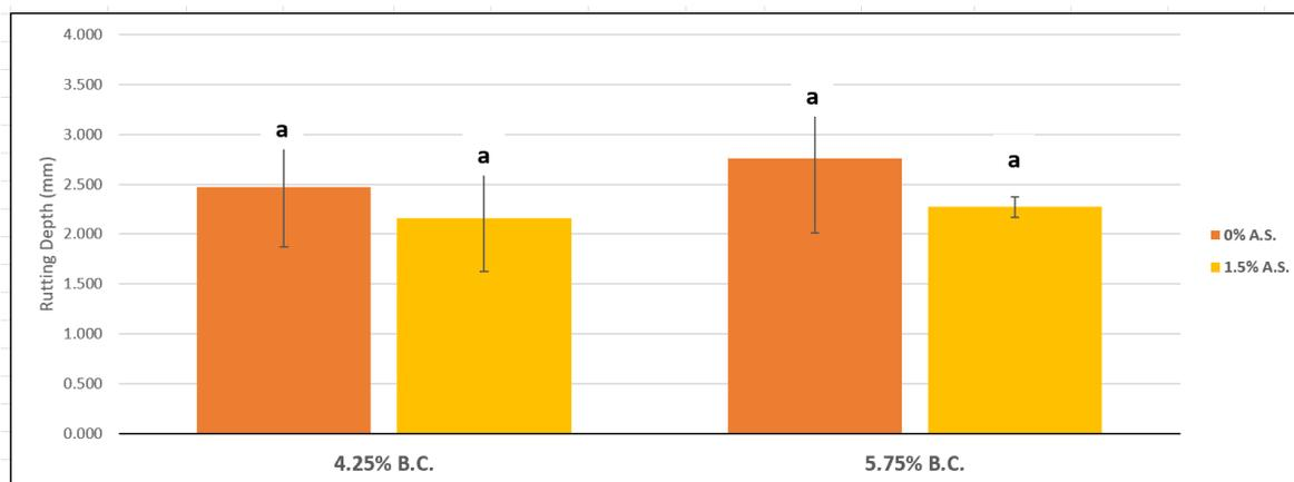
**Figure 4.30:** Effect of Anti-Strip Agent on HWTT Rutting
