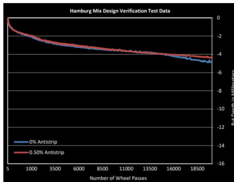
**Figure 2.13:** Hamburg Rutting Depth using Polymer Modified Binder (DeVol, 2016)
