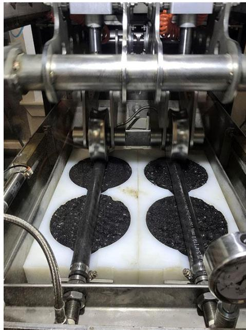
**Figure 2.1:** APA setup for Rutting Analysis (Asphalt Testing Solutions, 2021)
