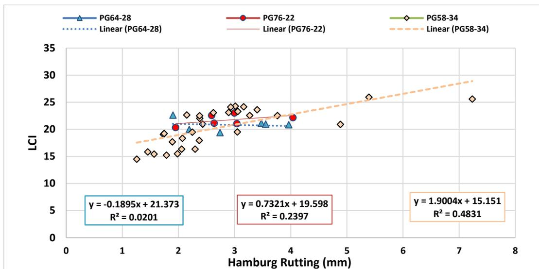
**Figure 4.25:** Correlation between LCI and HWTT Rut Depth at Different Binder Grades
