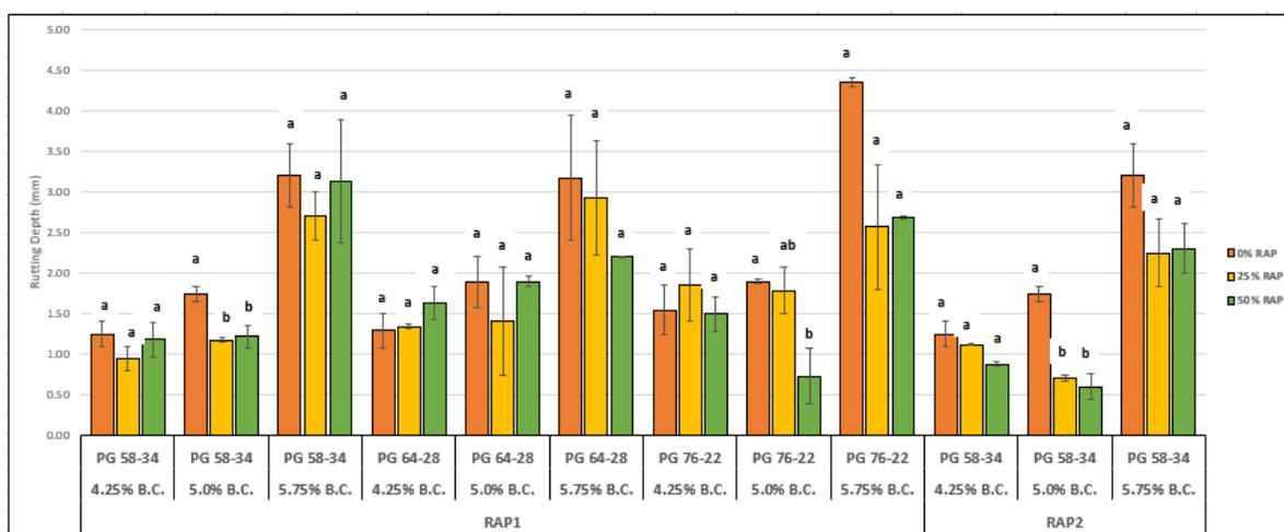
**Figure 4.3:** APA Rut Depth of LMLC Mixes
