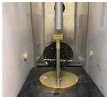
b. IDT testing Set up
