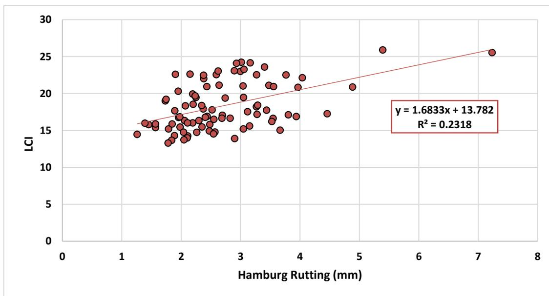
**Figure 4.24:** Correlation between LCI and HWTT Rut Depth
