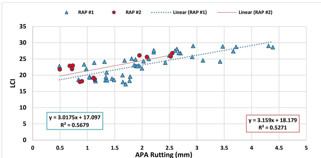
**Figure 4.22:** Correlation between LCI and APA Rut Depth at Different RAP Contents
