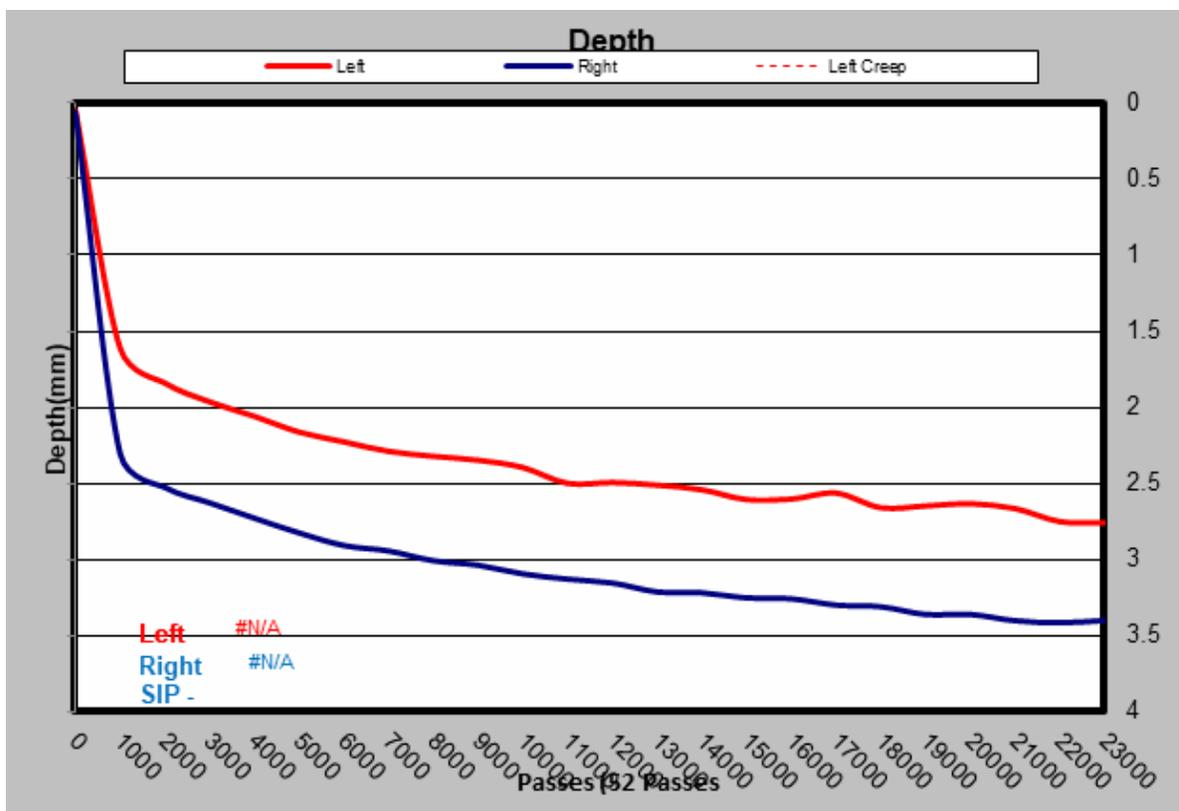
**Figure 10B:** Hamburg Rutting Data Sample @ PG 58-34, 0% RAP and 4.25% B.C.
