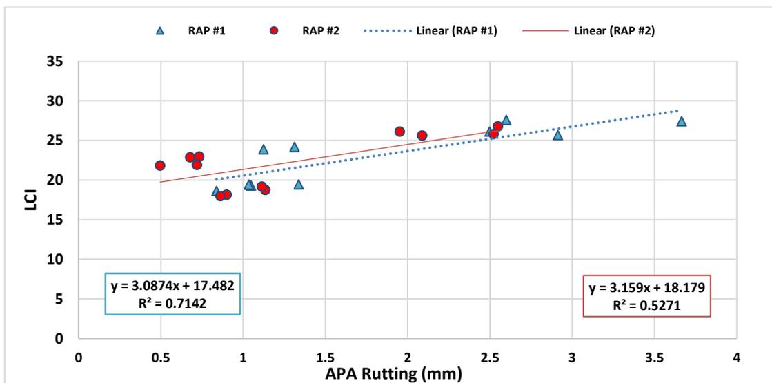
**Figure 4.23:** Correlation between LCI and APA Rut Depth at RAP Contents using PG 58-34
