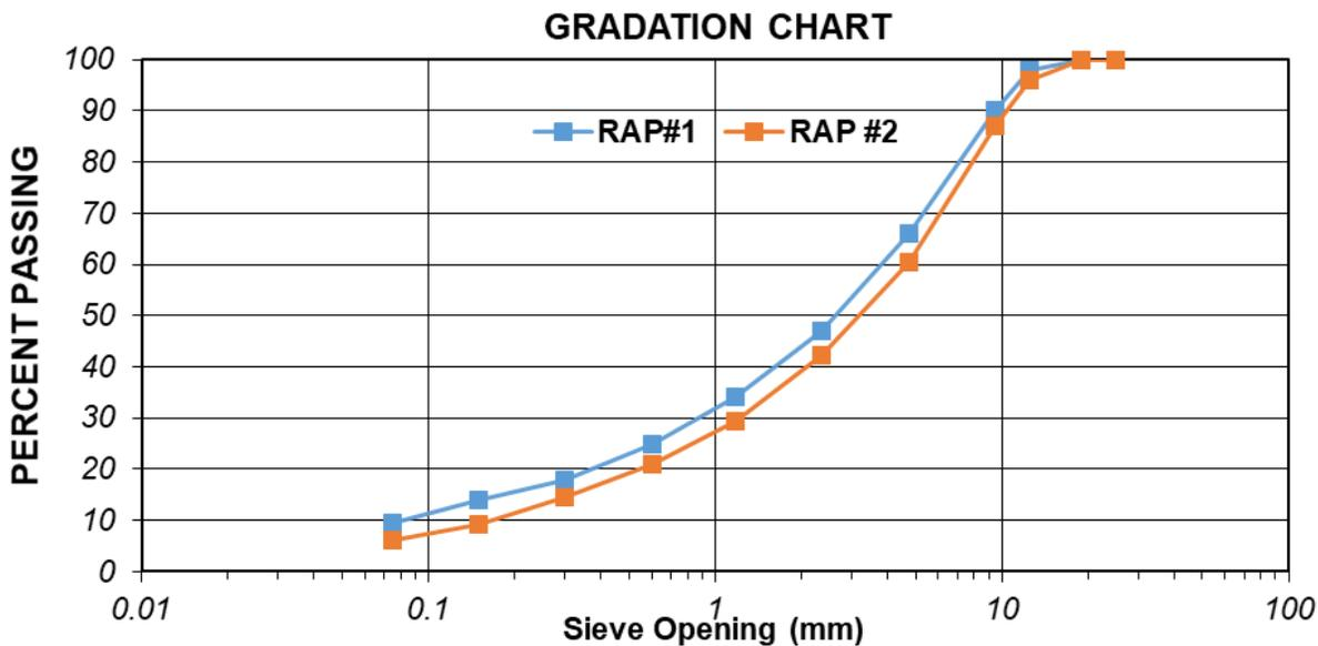
**Figure 3.2:** Aggregate Gradation of RAP #1 and RAP #2
