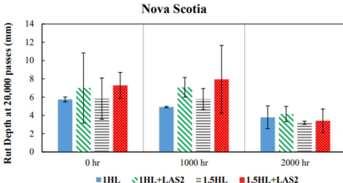
**Figure 2.30:** Rut Depth of Nova Scotia FC-5 Asphalt Mixtures after 20,000 Passes (Gu et al., 2020)
