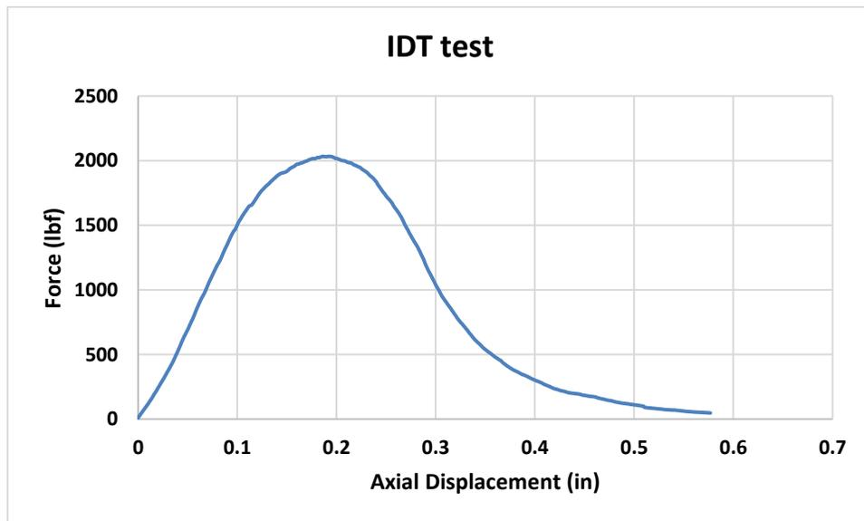
**Figure 16B:** Lottman Wet IDT Testing Sample 0% RAP, 0% ASA, 4.25% B.C.
