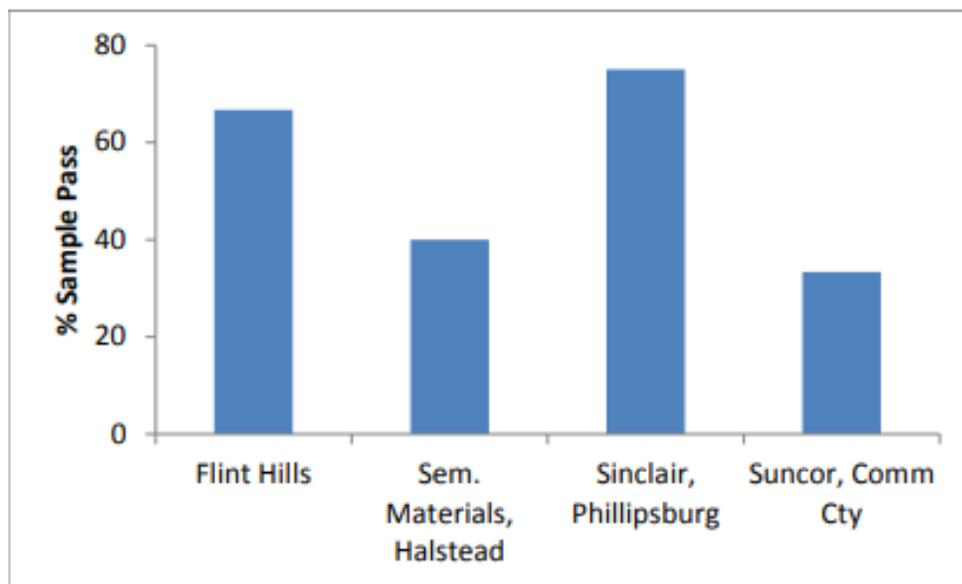
**Figure 2.23:** Effect of Binder Source on HWTT Test Results (Rahman and Hossain, 2014)
