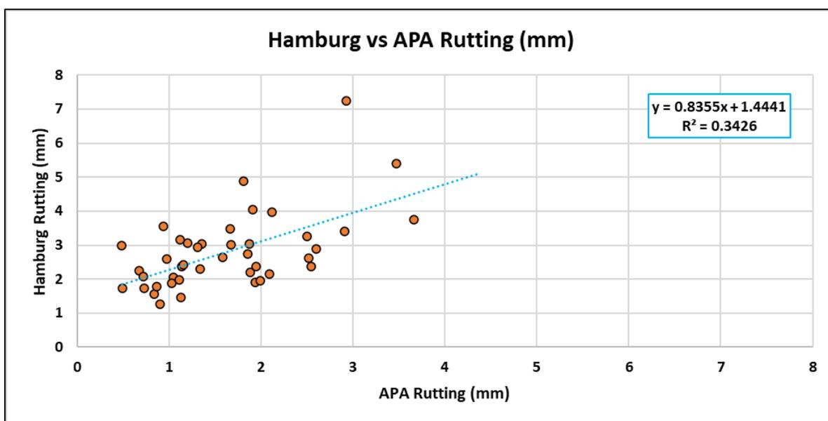
**Figure 4.13.** Correlation between APA and HWTT for LMLC Mixes
