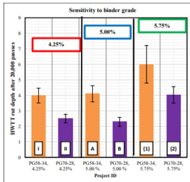
**Figure 2.20:** Sensitivity of HWTT Rut Depth after 20,000 Passes to PG Grade (Kassem et al., 2019)
