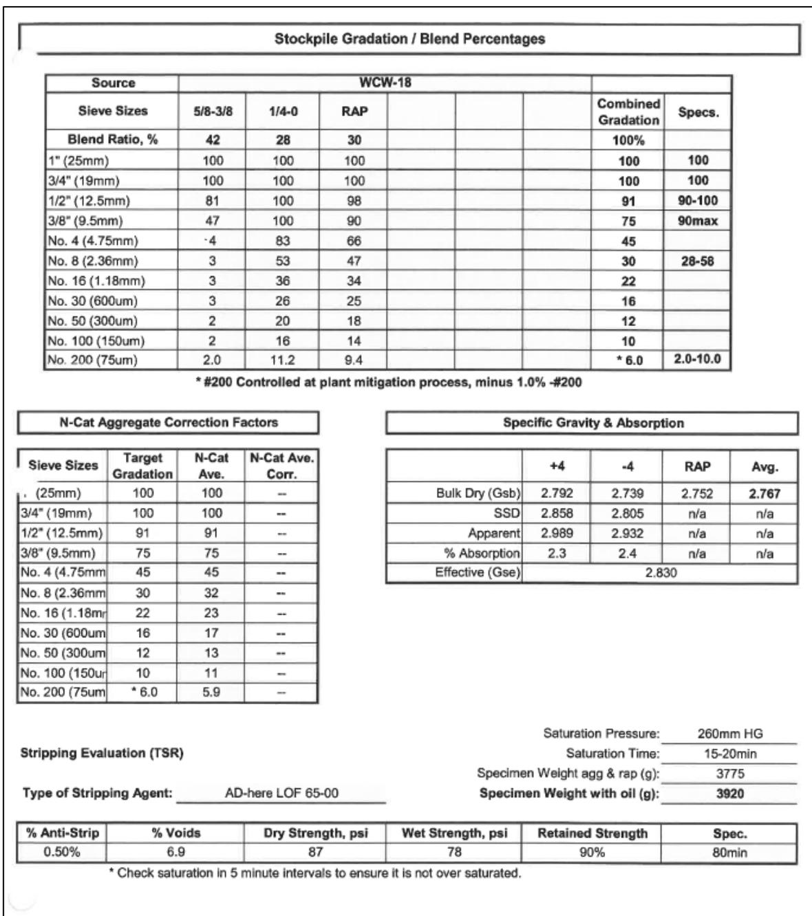
Figure 1A: SP5 Mix Design for the First Source of RAP (cont.)
