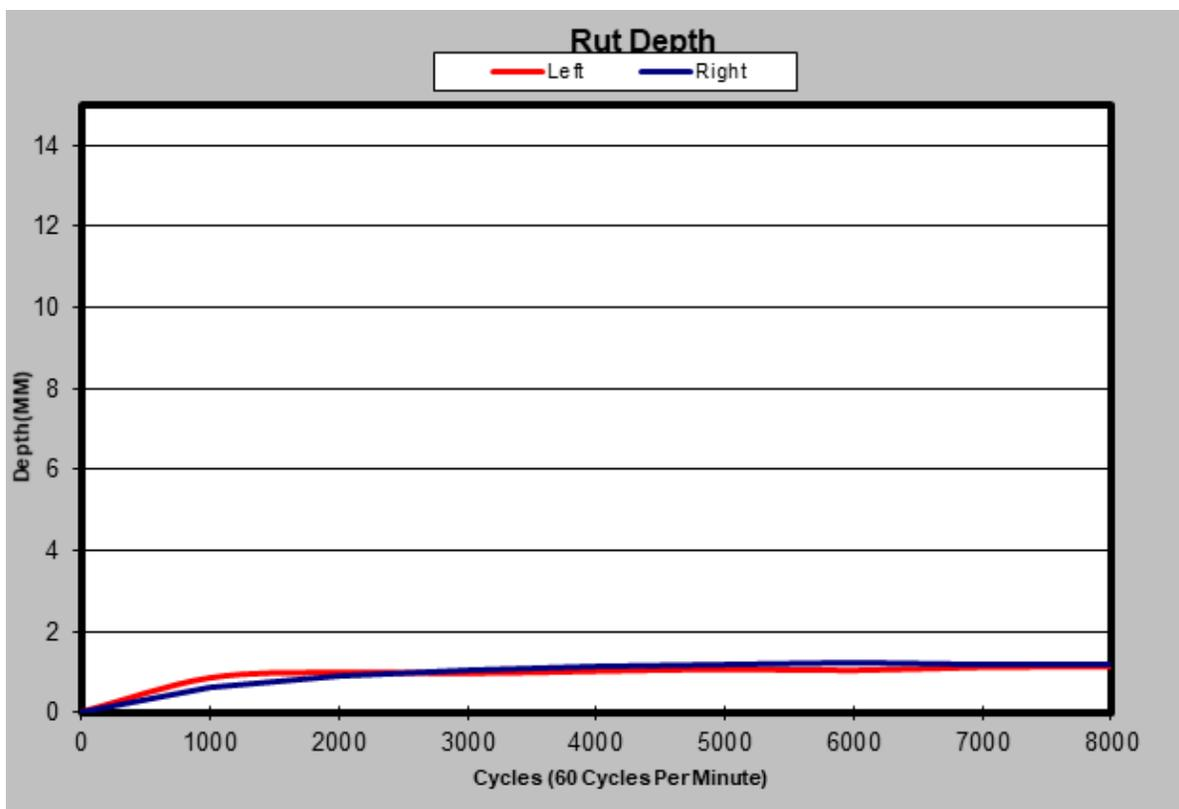
**Figure 8B:** APA Rutting Data Sample @ PG 58-34, 25% RAP and 5.0% B.C.
