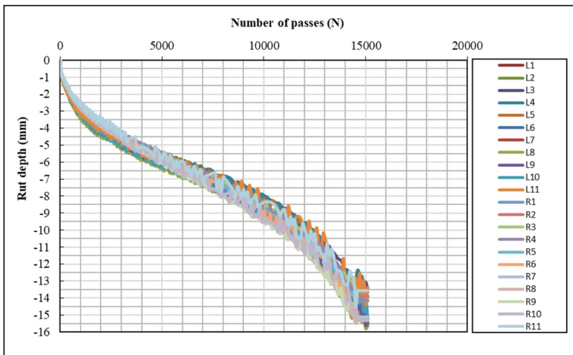
**Figure 3.6:** HWTT Left and Right (L1-L11, R1-R11) Wheel Data Points
