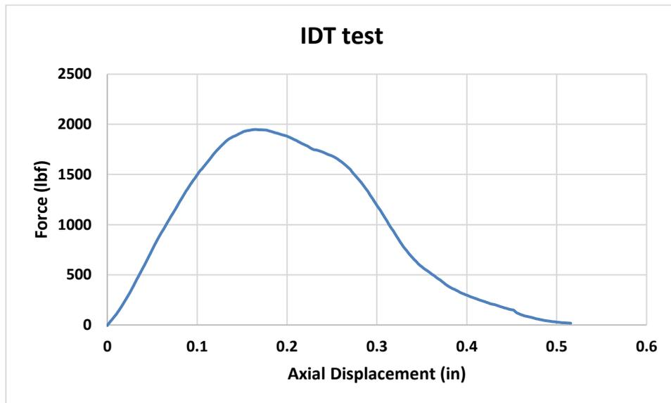
**Figure 14B:** Lottman Wet IDT Testing Sample 0% RAP, 0% ASA, 5.0% B.C.
