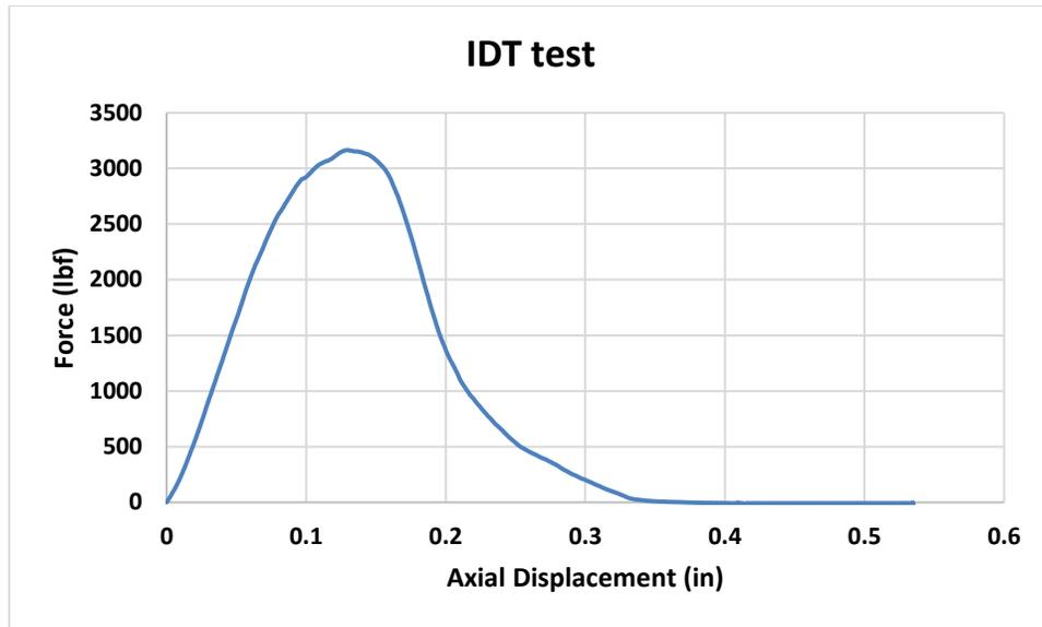
**Figure 15B:** Lottman Dry IDT Testing Sample 0% RAP, 0% ASA, 4.25% B.C.
