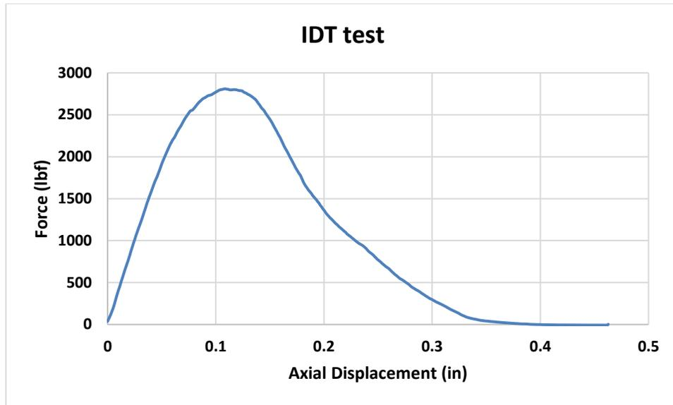
**Figure 13B:** Lottman Dry IDT Testing Sample 0% RAP, 0% ASA, 5.0% B.C.
