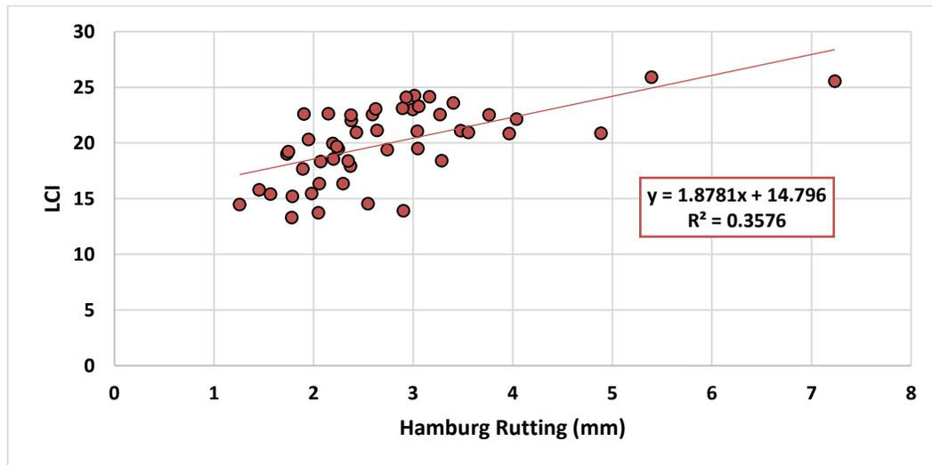
**Figure 4.28:** Correlation between LCI and HWTT Rut Depth for LMLC Mixes
