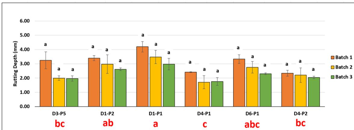
**Figure 4.14:** Hamburg Testing of Field Prepared Mixes
