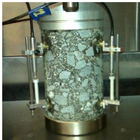
**Figure 2.7:** Dynamic Modulus Test Setup (Masad et al., 2011)
