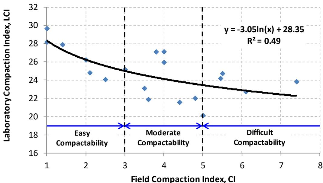
**Figure 2.9.** Relationship between laboratory and field HMA compaction as proposed by Kassem et al. (2012)
