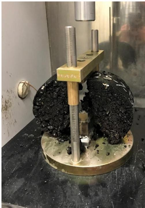
**Figure 2.6:** IDT Test Sample after Testing
