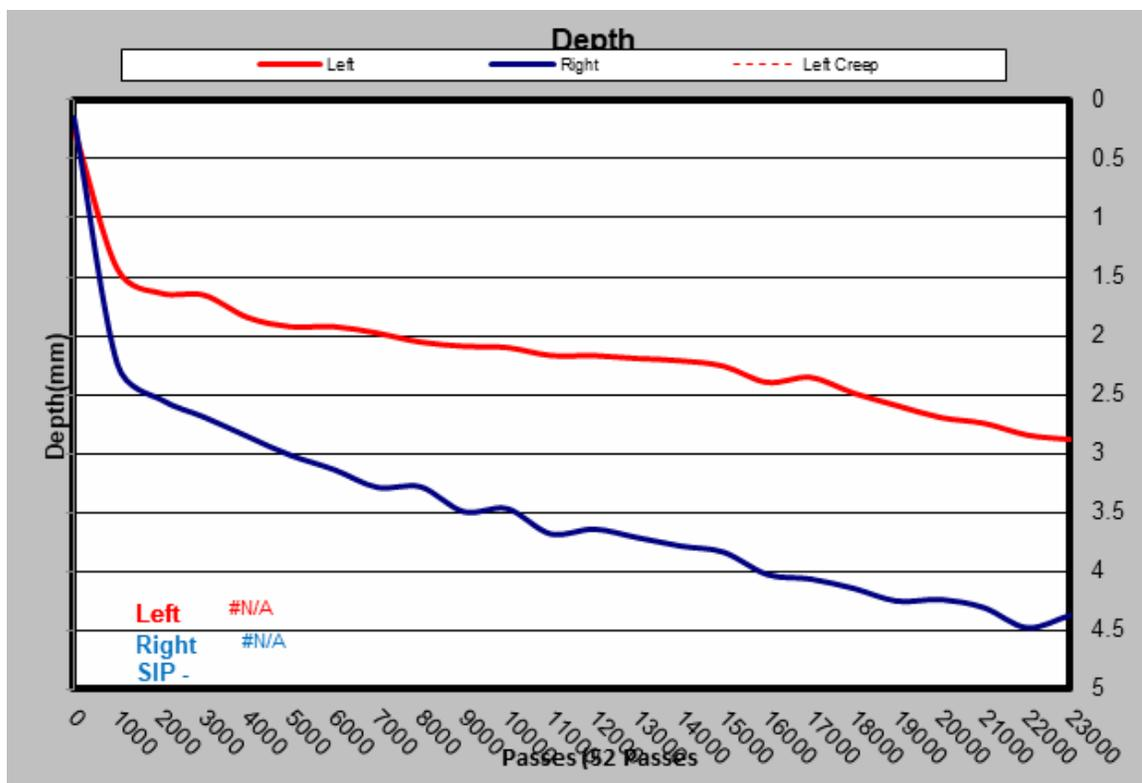
**Figure 11B:** Hamburg Rutting Data Sample @ PG 64-28, 25% RAP and 5.0% B.C.
