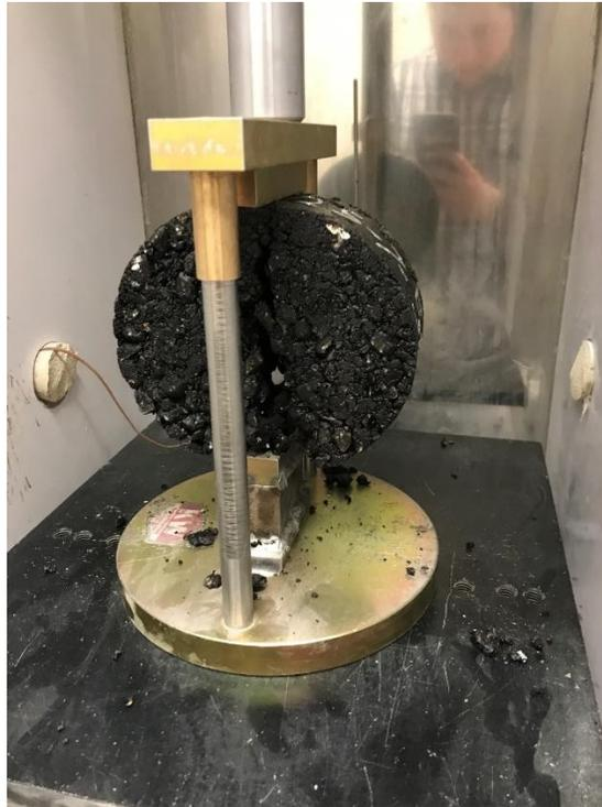
**Figure 2.5:** Sample Setup inside the MTS
