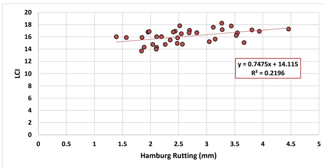
**Figure 4.27:** Correlation between LCI and HWTT Rut Depth for PMLC Mixes
