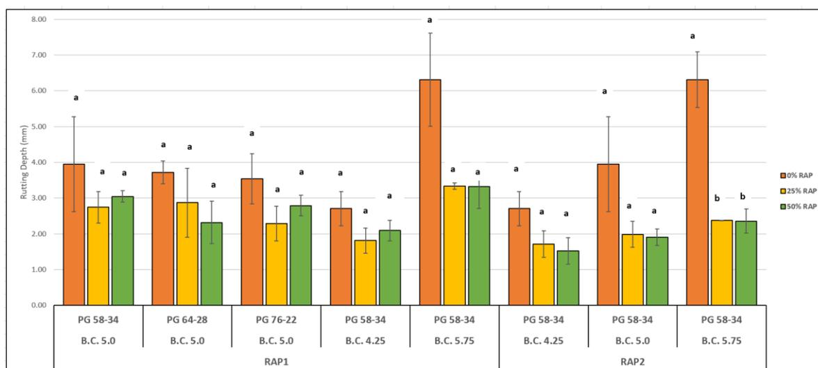
**Figure 4.4:** HWTT Rut Depth of LMLC Mixes
