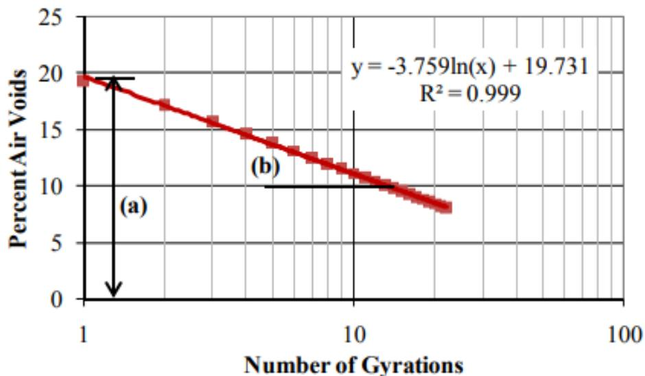
**Figure 2.8:** Example of SGC Compaction Curves (Kassem et al., 2012)
