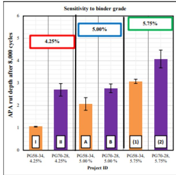
**Figure 2.21:** Sensitivity of APA Rut Depth at 8,000 Cycles to PG Grade (Kassem et al., 2019)
