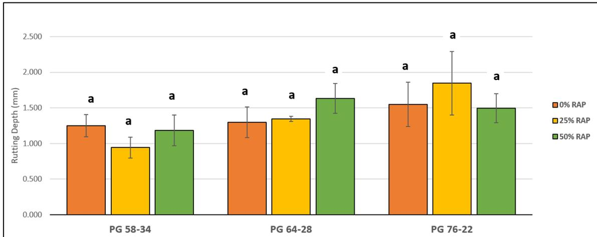
**Figure 4.5:** Comparison of APA Rutting with Different Binder Grades at 4.25% Binder Content
