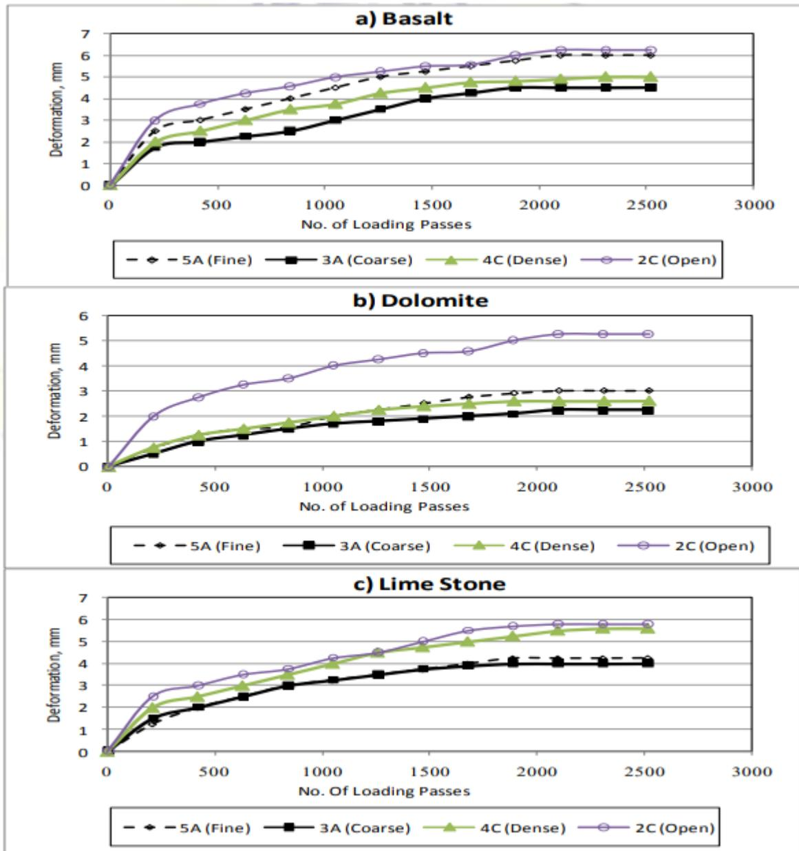
**Figure 2.18:** Effect of Aggregate Gradation on Rutting Resistance (Ahmed and Attia, 2013)
