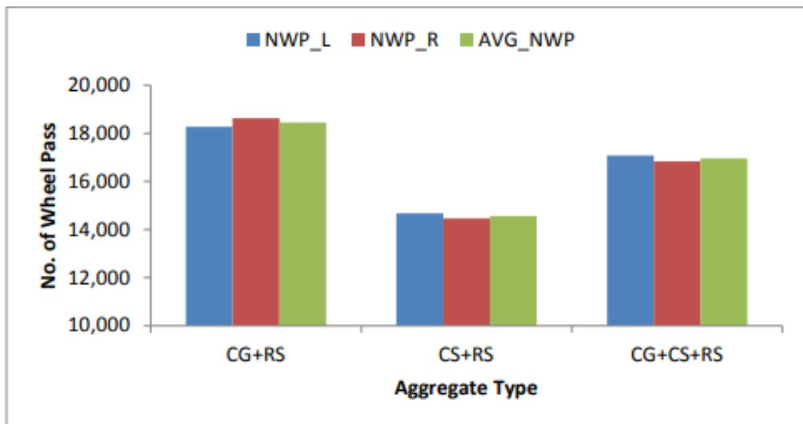
**Figure 2.16:** Effect of Aggregate Type on Hamburg wheel passes (Rahman and Hossain, 2014)
