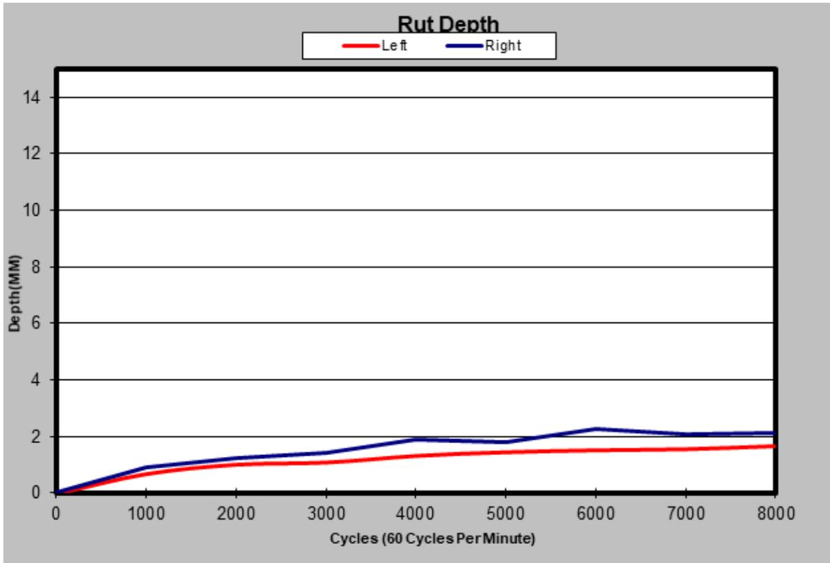
**Figure 7B:** APA Rutting Data Sample @ PG 64-28, 0% RAP and 5.0% B.C.
