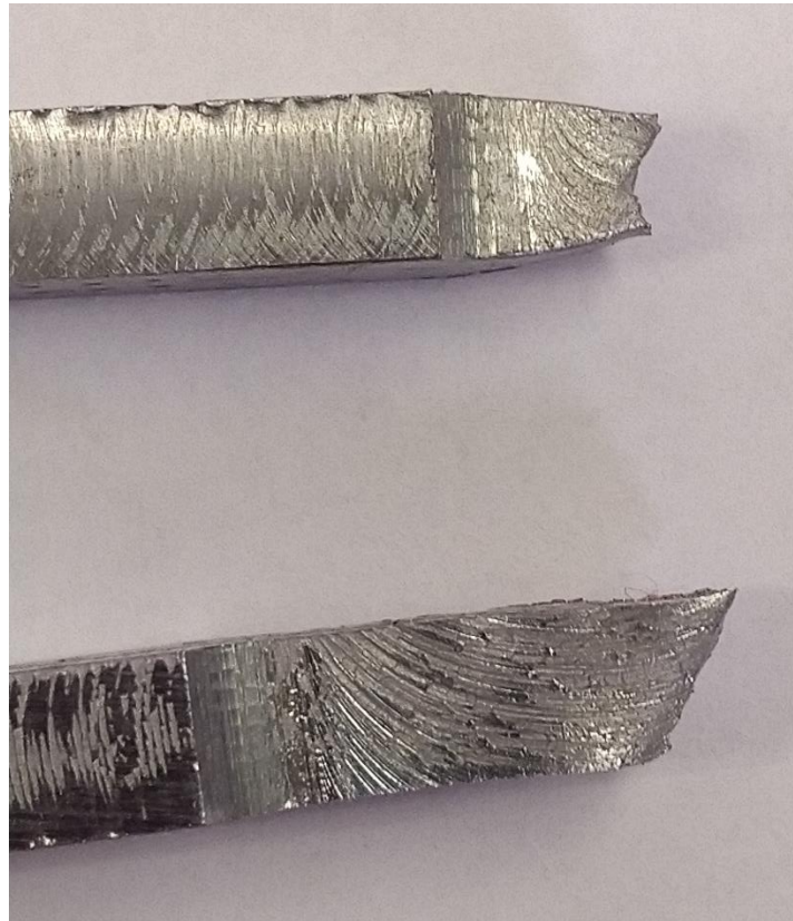
Figure 3.2 - Fracture surfaces of tensile specimens, control sample (top) test sample (Bottom).
