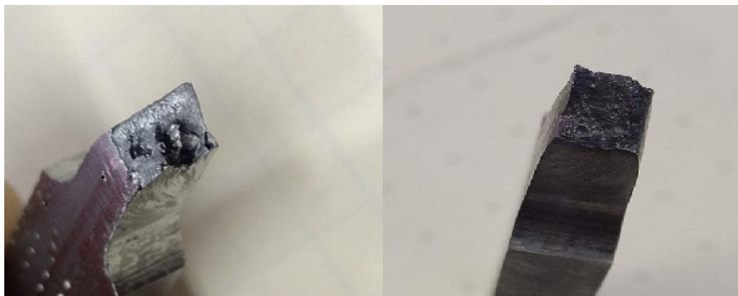
Figure 3.1 - Image of the porosity in test sample No. 2 (left) and a good sample with no porosity (right)
