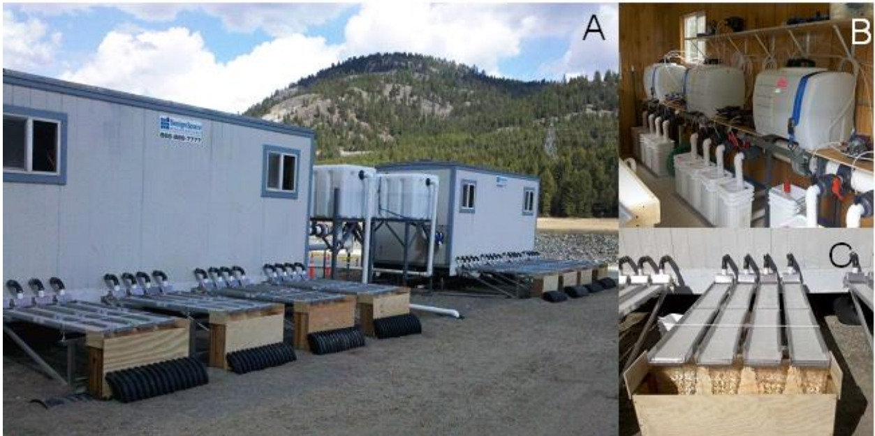
Figure 3-1. Mobile experimental flume system (MEFS) at the Kootenai River Research Station downstream of Libby Dam in Libby, MT, USA. A) Mobile experimental flume system (MEFS) with 32 external flumes supplied by water from the Kootenai River. B) Internal structure of MEFS with 120 L stock tanks on shelving and mixing header tanks for individual flumes below. C) External flumes of the MEFS. Flumes were lined with 6 mm open-celled Styrofoam for substrate.
