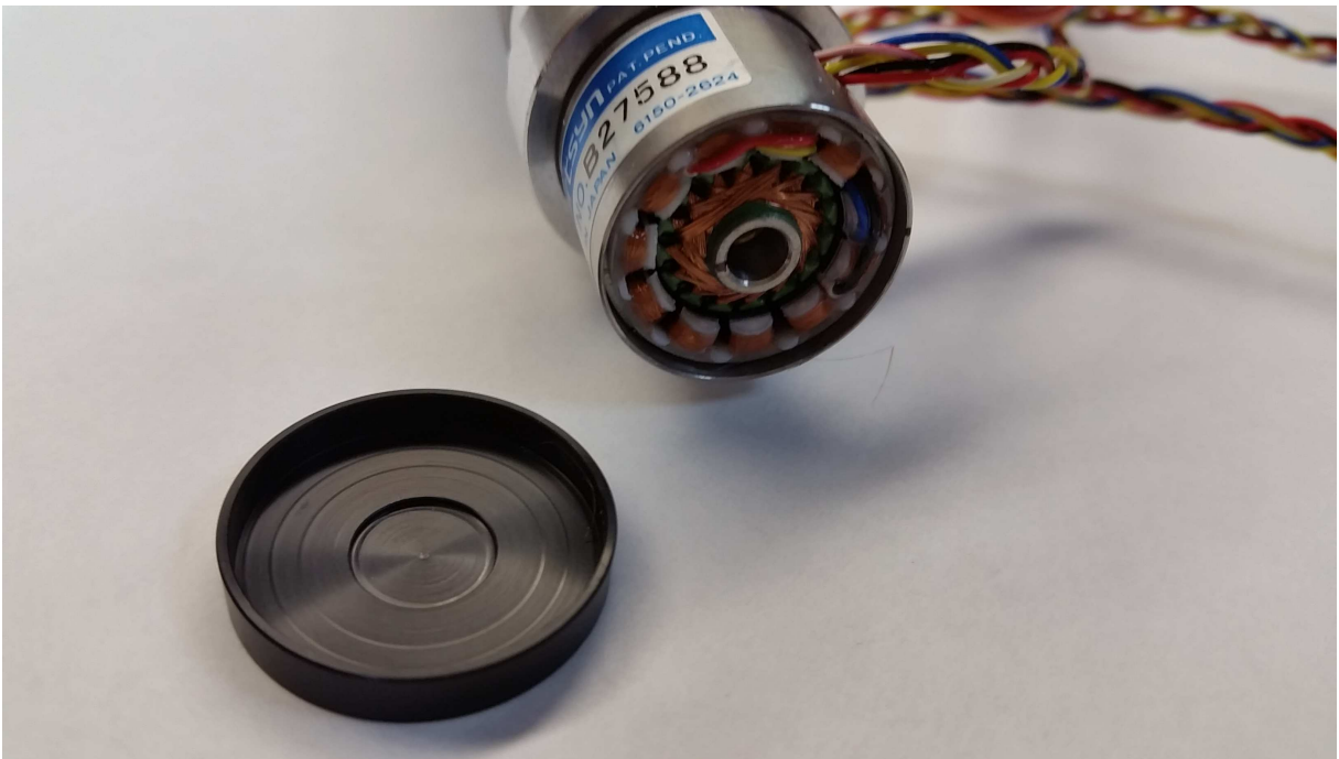
Figure I 7: Tamagawa Smartsyn TS2605N31E64 resolver employed in this project.
