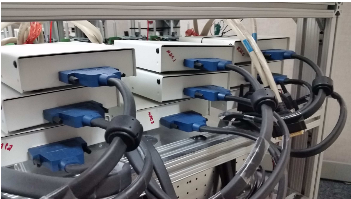
Figure I 2: Array of SCB-68 M Series Devices Connectors used to link driver and resolver circuit with NI system.
