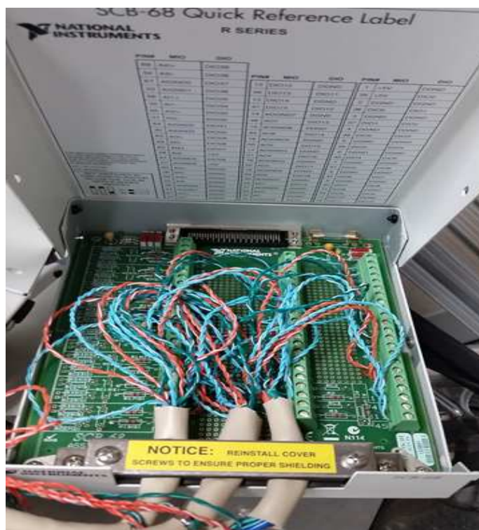
Figure I 3: Labeled SCB-68 M Series Devices Connectors used to link driver and resolver circuit with NI system.
