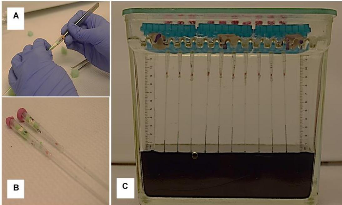
Figure 4.1. Measurement of Respiration rate of the potato psyllid. Preparation of respirometers (A); respirometers containing live psyllids (B) are placed in the chamber to run the experiment (C).
