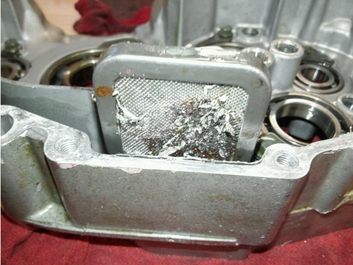
Figure 24. Plugged oil pickup screen.
