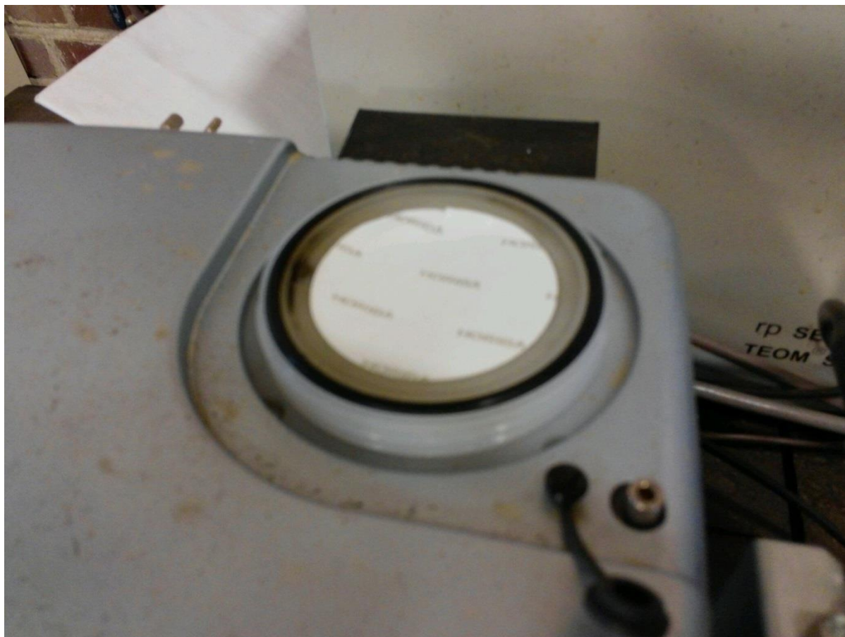
Figure 26. Dust filter element.
