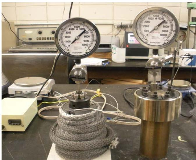
Figure 2.1 High pressure pretreatment reactors: 75 mL (left) and 500 mL (right)
