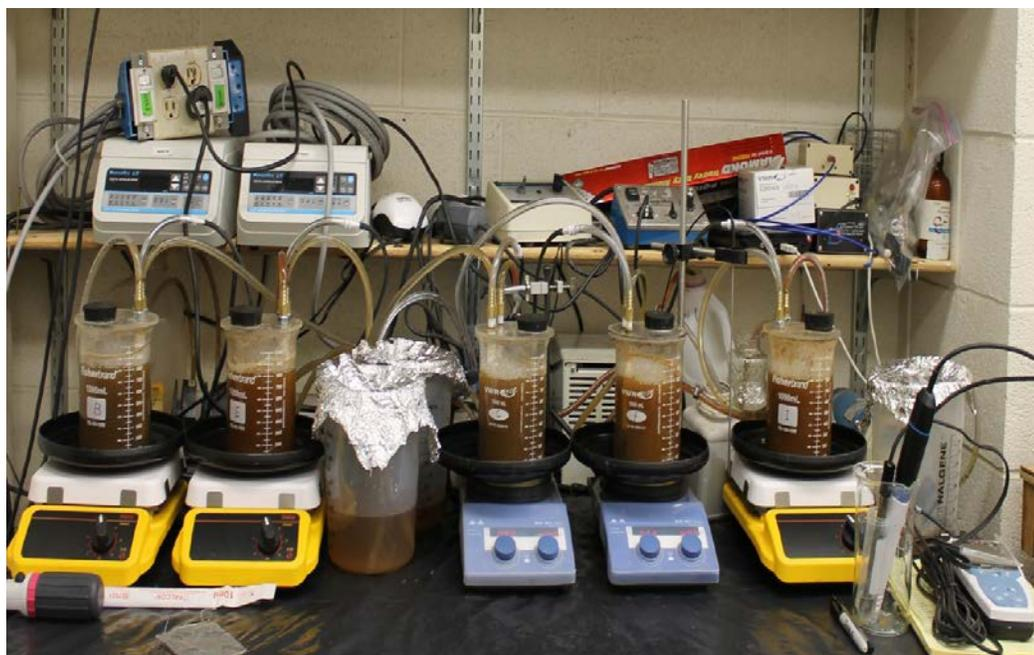
Figure 3.1 Continues fed-batch bioreactors set-up
