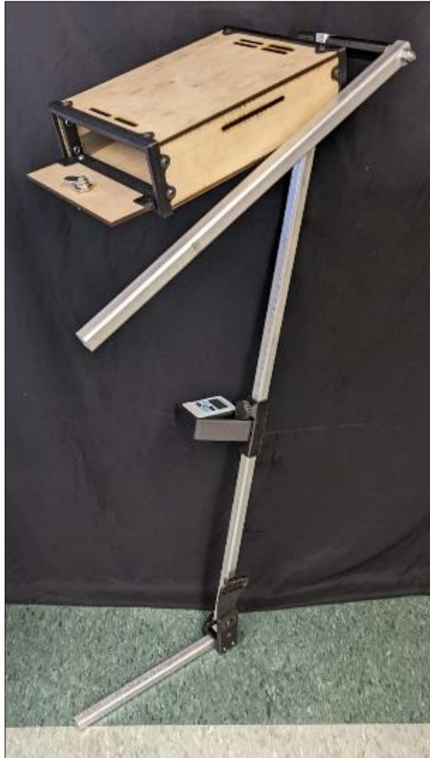
Figure 29: DARLING Lite configuration 1. Being the highest level of the configuration line, this combination provides a custom writing desk supported by bending strength measurement, and angular deflection measurement gauges.
