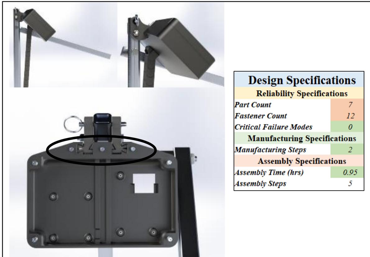
Figure 12: Final iteration of the casing design and specifications. No additional features are provided by this design, with the significant change being a reinforcement of the notched mounting joint. Green fill in the specification table indicates a positive change, and red fill indicates a
