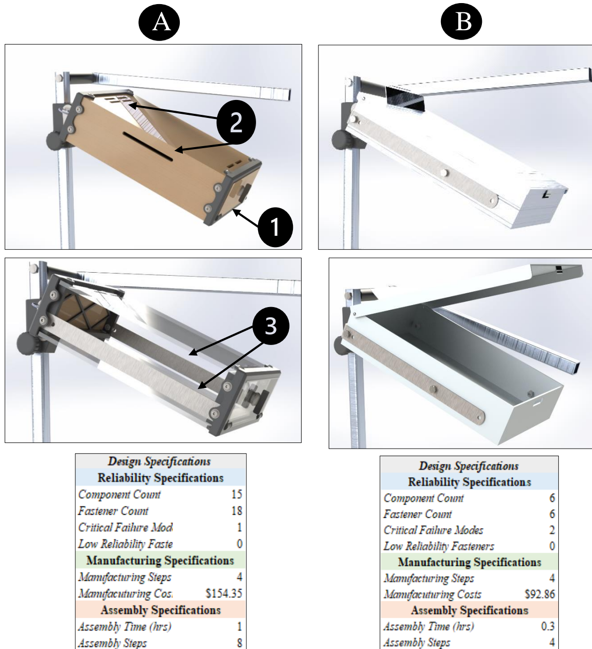
Figure 23: LEFT: Data management module hardware options A. RIGHT: Hardware option B and its respective specifications. The unit cost measurements include all material, fabrication, and assembly related costs.
