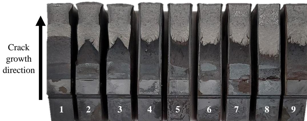
Fig. 4.1. Fracture surfaces of all nine specimens.
