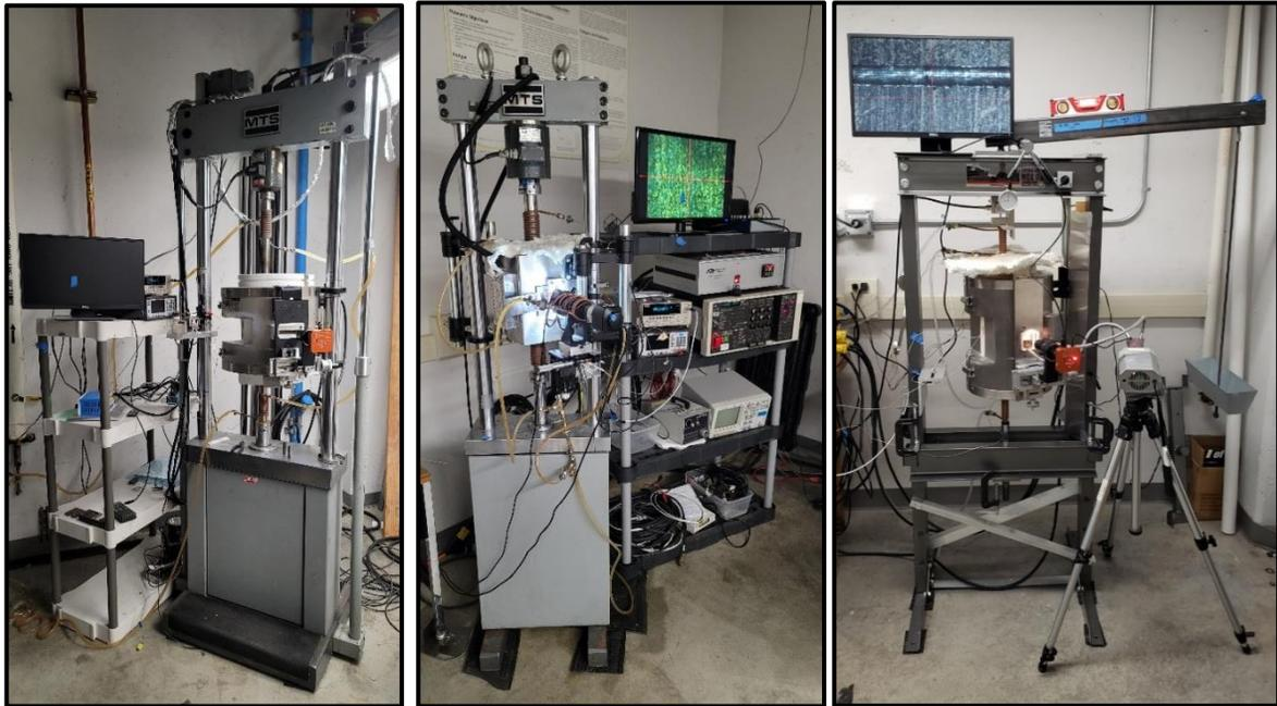
Fig. 3.2. Load frames from left to right: MTS 312.11 44 kN (10 kip), MTS 312.12 97 kN (22 kip), deadweight creep frame.
