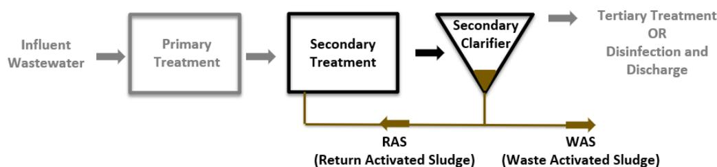
Figure 2. Basic diagram of the primary elements of wastewater treatment.
