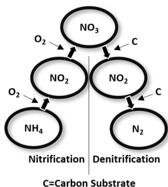
Figure 3. Diagram of nitrification and denitrification.
