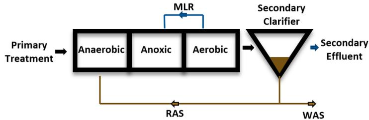
Figure 1. Common layout of a BPR WRRF.
