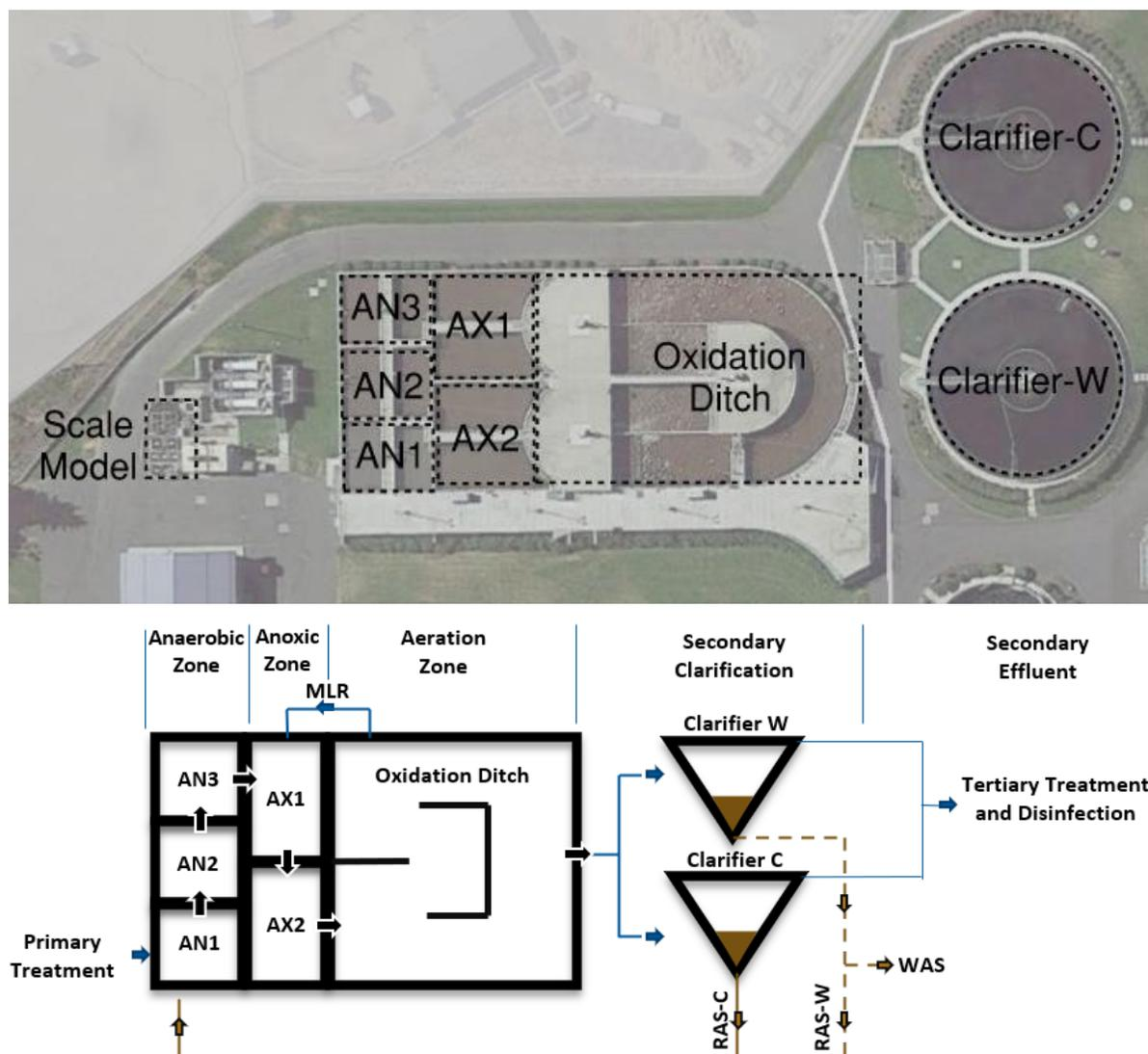
Figure 4. Diagram and aerial of the Moscow BPR WRRF. Background aerial image from Google Earth 6-2021.
