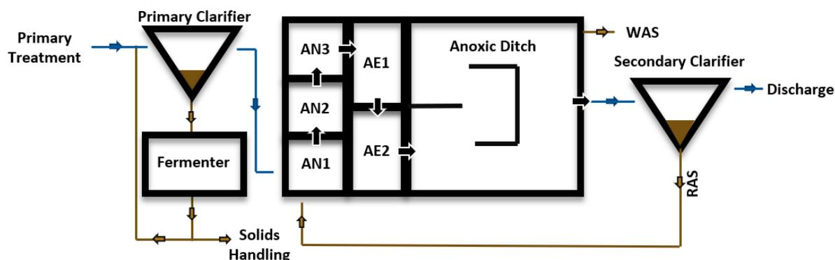
Figure 6. Diagram of the Moscow scale model WRRF.
