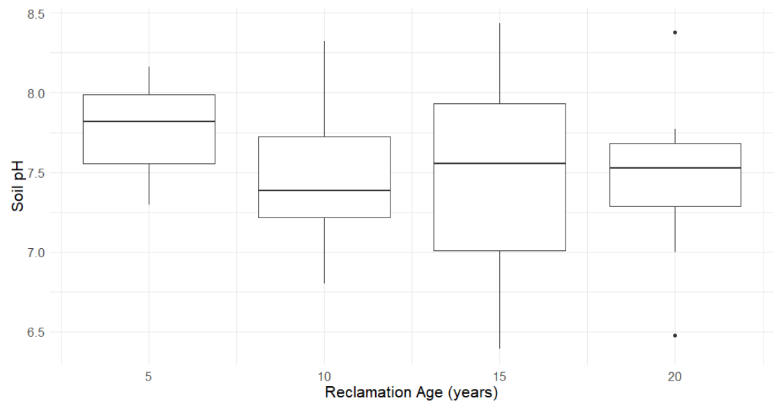
Figure 4.2: Boxplots of soil pH values for each time period since reclamation completion (reclamation age).
