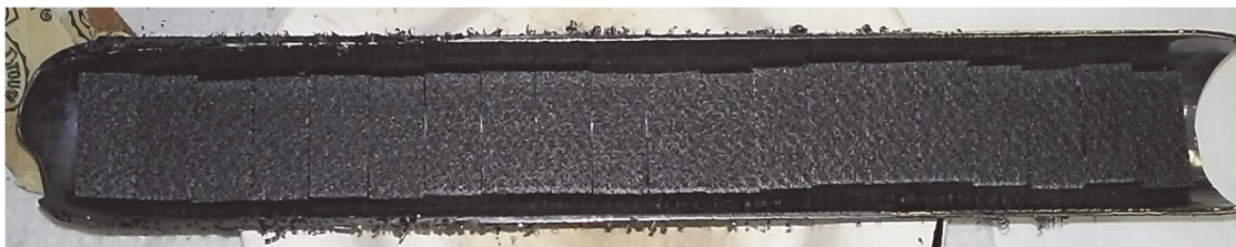
Figure 2.5 Graphite felt samples in quartz boat after GUITAR coating.
