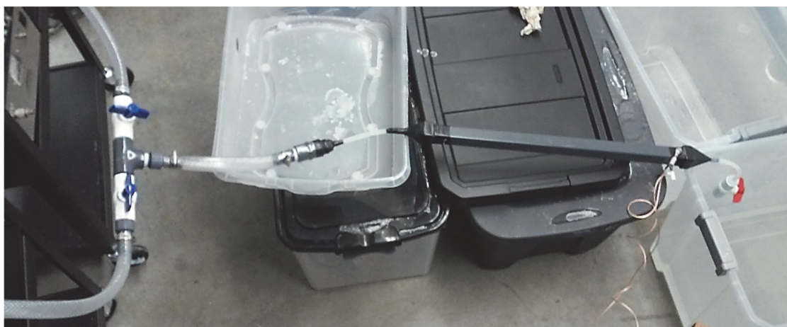
Figure A.2 Flow control valve setup and experimental channel. Ball valves used at outlet to control the flow rate.
