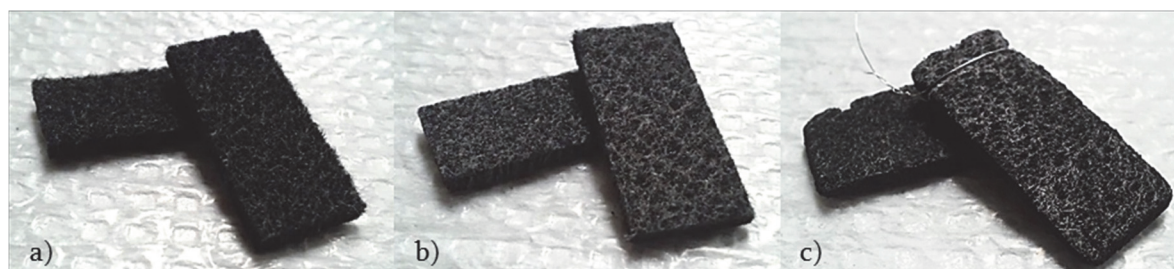
Figure 2.3 Electrodes used in experiments: a) SGL bare graphite felt, b) GUITAR-coated SGL graphite felt, and c) GUITAR-coated SGL graphite felt with nanosprings.
