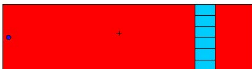
Figure 4.29: Vised rendering of general TC homogeneous vs. heterogeneous model. Top view. Red indicates air, dark blue is the Pu source, light blue is the TC array. See Figure 3.5 for homogeneous arrangement of TC's.
