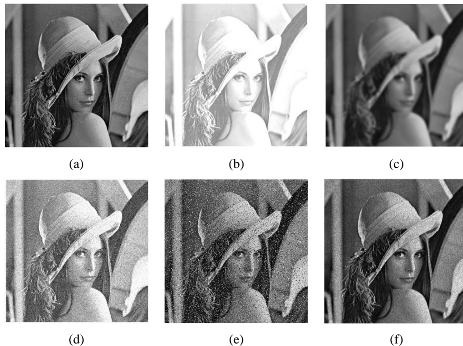
Figure 4.8. Samples of different types of distortions (a) Original (b) Brightness change (c) Blur distortion (d) Gaussian noise distortion (e) Salt and peppers distortion (f) Multiplicative noise distortion
