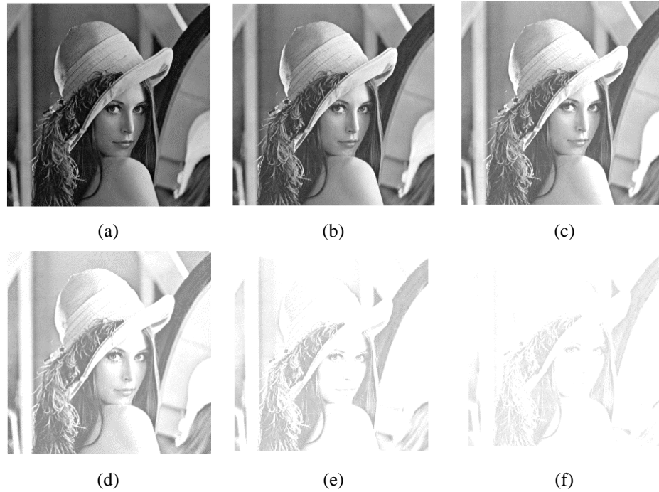
Figure 4.9. Brightness increasing of Lena image from +40 to +200 (a) Original (b) +40 (c) +80 (d) +120(e) +160 (f) +200
