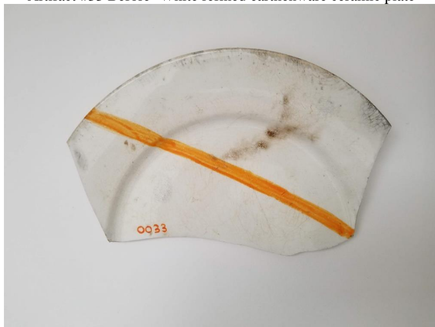
Artifact #33 After- Note new staining in center and increased staining in crazed glaze of rim on right
