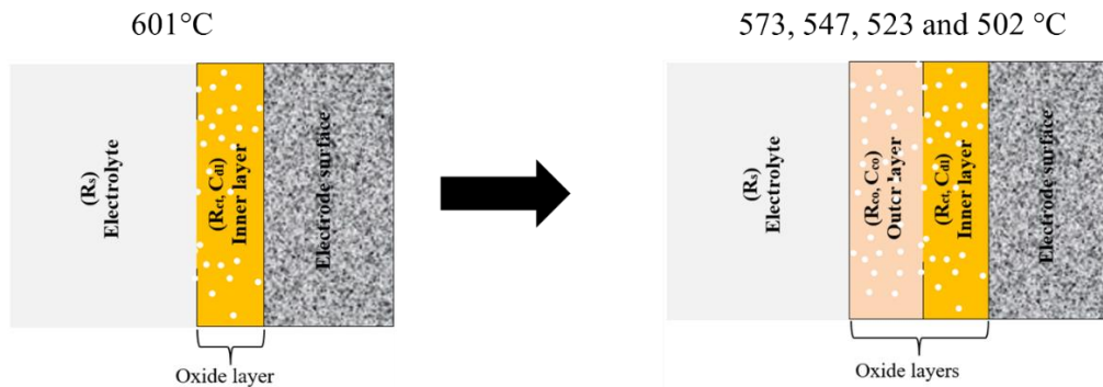
Figure 4.67. Corrosion mechanism for Inconel 600 in molten carbonate 0.3 GDC – 0.7 (0.67Li 2 CO 3 -0.33K 2 CO 3 ) salts with varying temperatures of 502 °C, 523 °C, 547 °C, 573 °C and 601 °C, displaying the number of oxide layers formed of the surface of the electrode as modelled by Figure 4.61.
