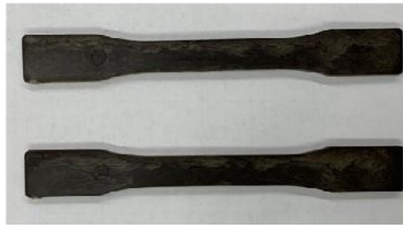
Figure 2.2 Tensile dog-bone specimens
