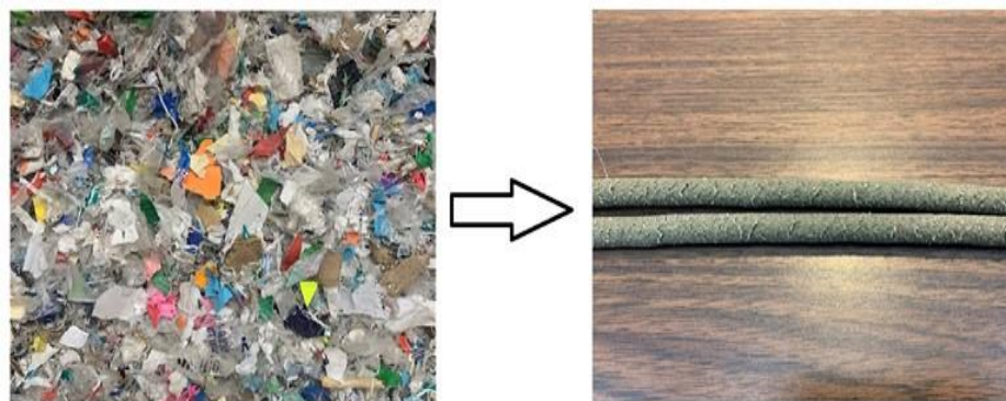
Figure 2.1 Shredded MPW to extruded rod
