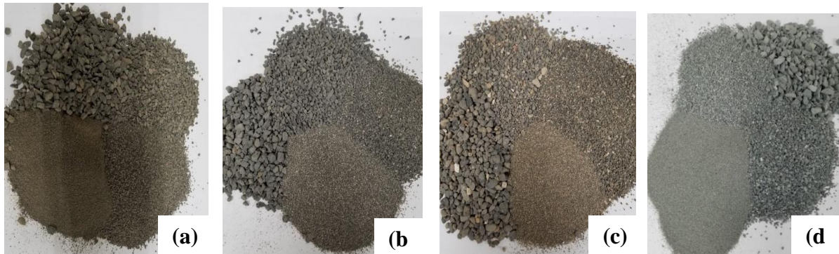
Figure 5.1: Reactive aggregates considered a) Wn-56; b) Basalt rocks; c) Manufactured Sand; d) non-reactive aggregates (granite)
