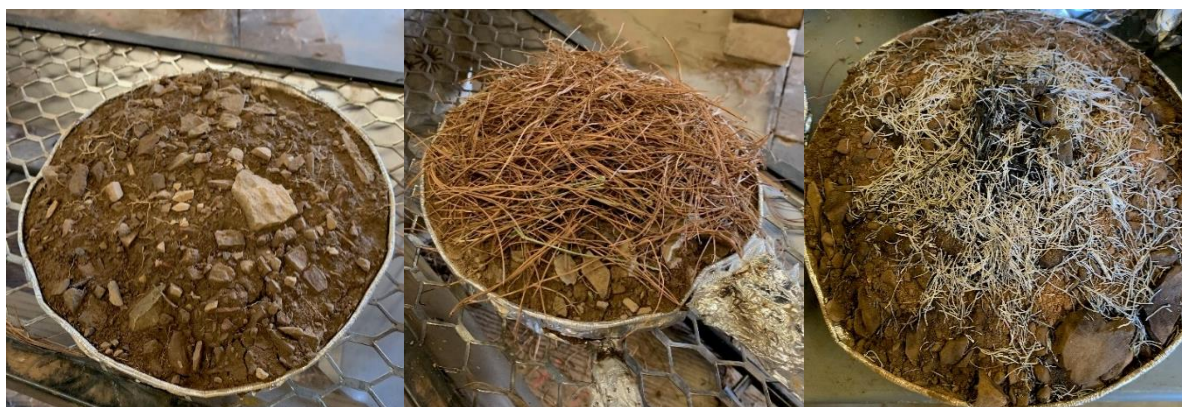
Figure 3-2: Reconstituted Soil Core constructed to match the coarse and fine size distribution and the average bulk density from bulk density samples collected in the field. The picture in the middle shows a reconstituted soil core in the aluminum pie pan with pine needles and thermocouples inserted (wrapped in an aluminum heat shield) ready to burn. The bulk density was reproduced by packing the soil core back to the original bulk density. The picture on the right shows a sample after burning.
