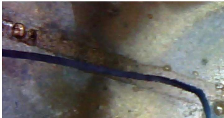
**Figure 19. Cracked spark gap specimen**
