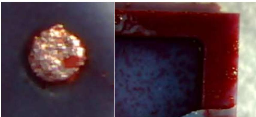
**Figure 17. Dye penetration in LTCC-via specimen**
