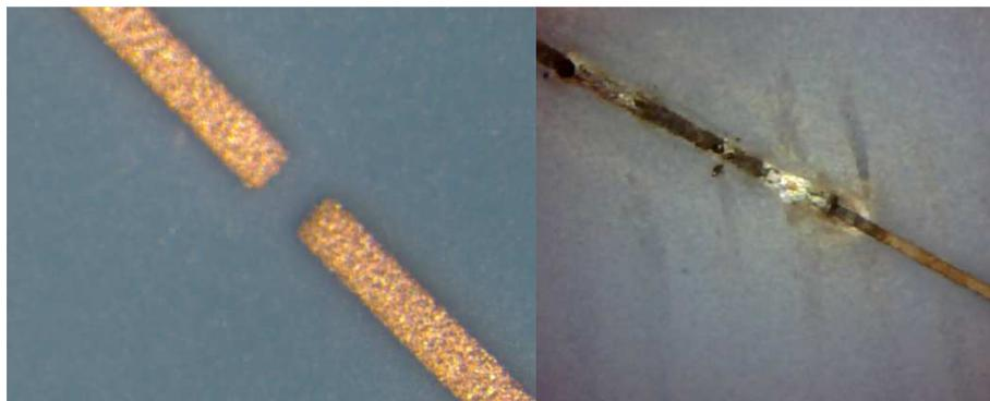
**Figure 18. Spark gap (left: pre firing, right: post firing)**
