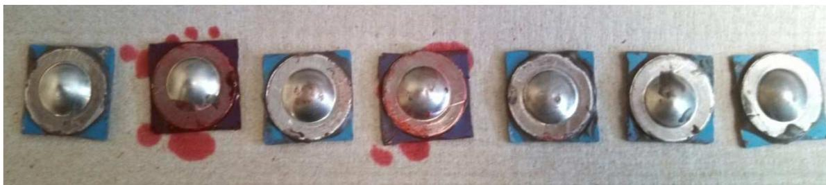
**Figure 6. Dye penetrant test on LTCC prototypes**
