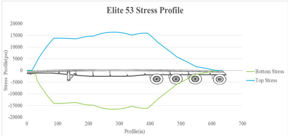
Figure 3.5: Elite 53 Numerical vs Experimental Data Stress Plot
