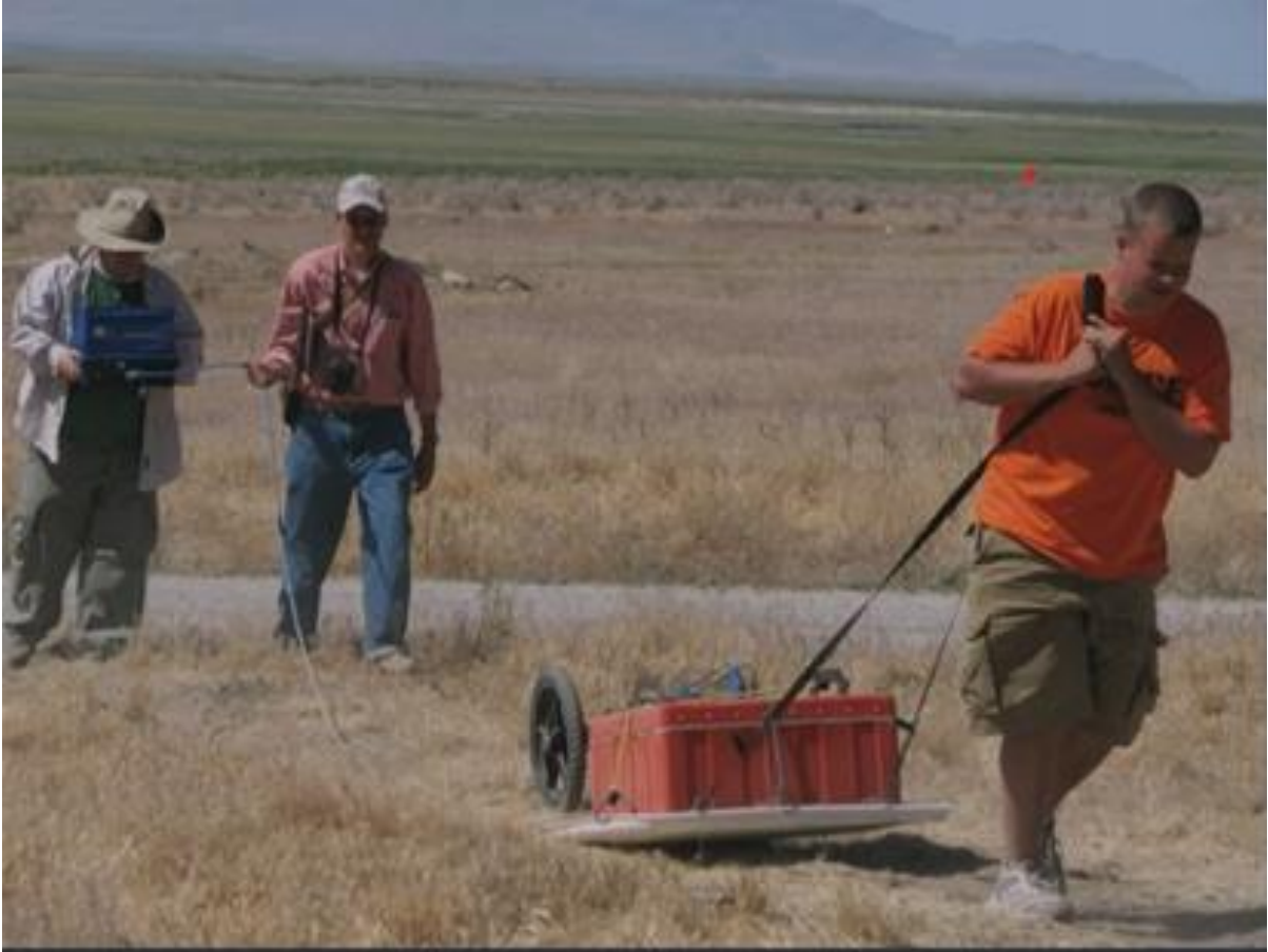
Figure 3.14 GPR being conducted at Iosepa townsite. Photo courtesy of Benjamin Pykles.
