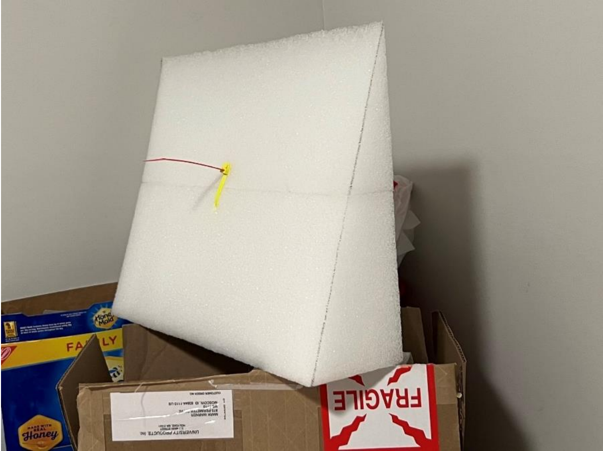
Figure 5.7 Wedge glued with Paraloid B-72 and cable tied together to set. Photo by author.
