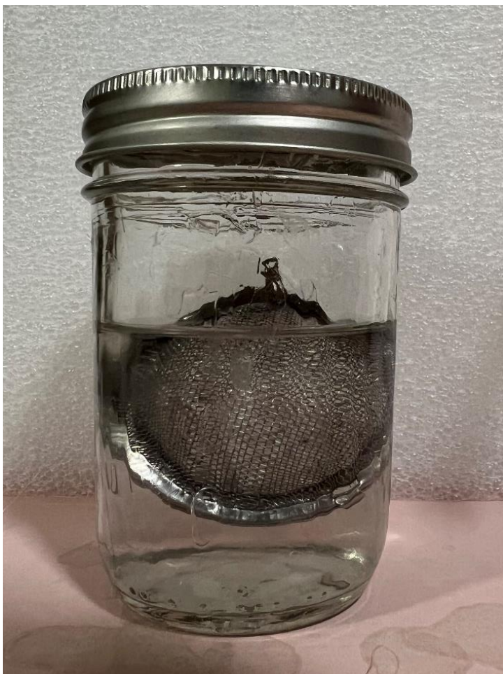
Figure 5.1 Paraloid B-72 pellets in tea ball suspended in acetone. Photo by author.
