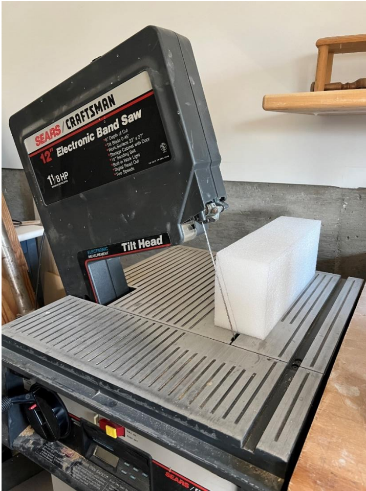
Figure 5.4 Bandsaw set to angle of slope. Photo by author.
