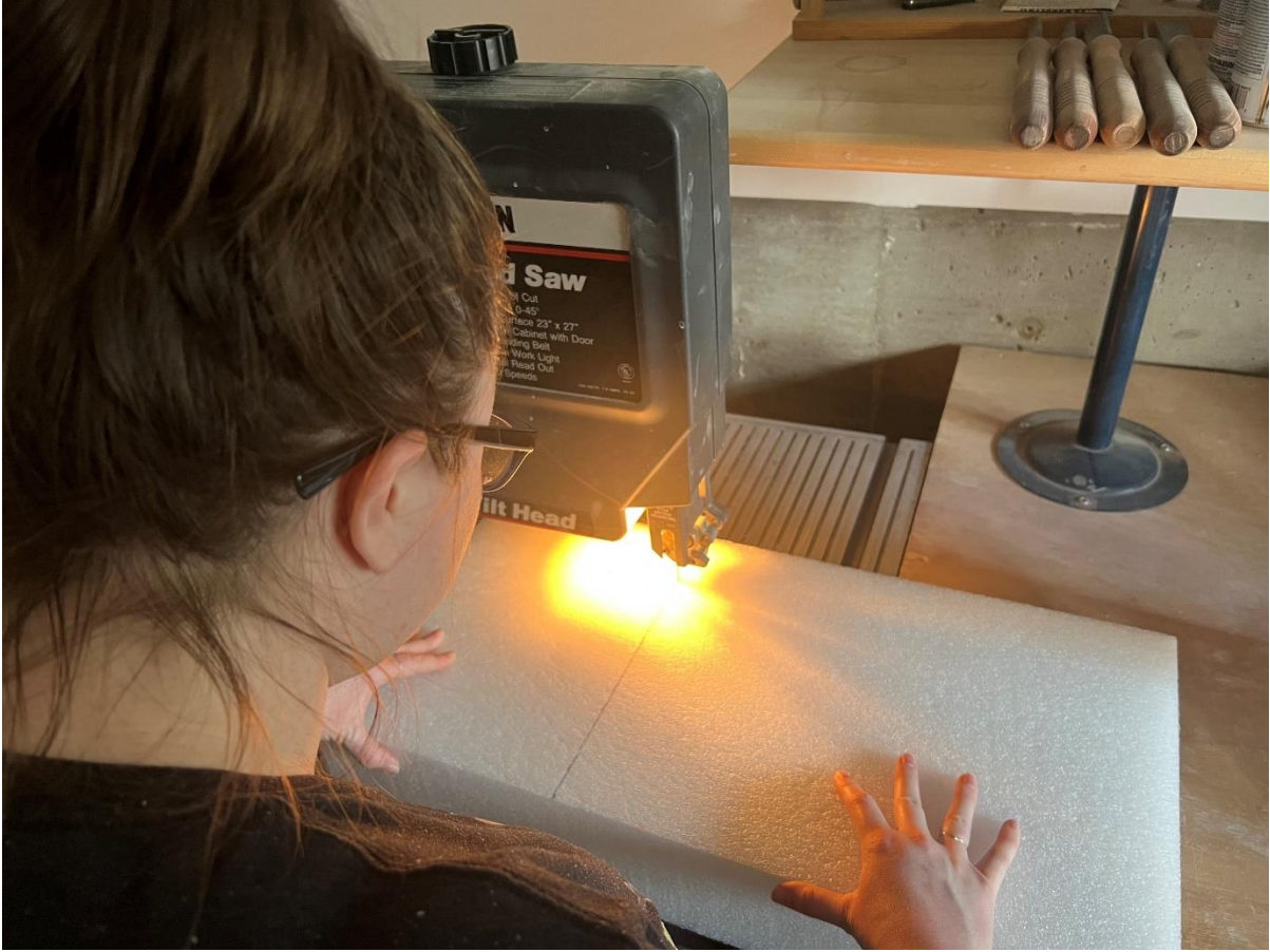
Figure 5.3 Author using bandsaw to cut Ethafoam plank to 16 inches. Photo by Rus Gerlach.
