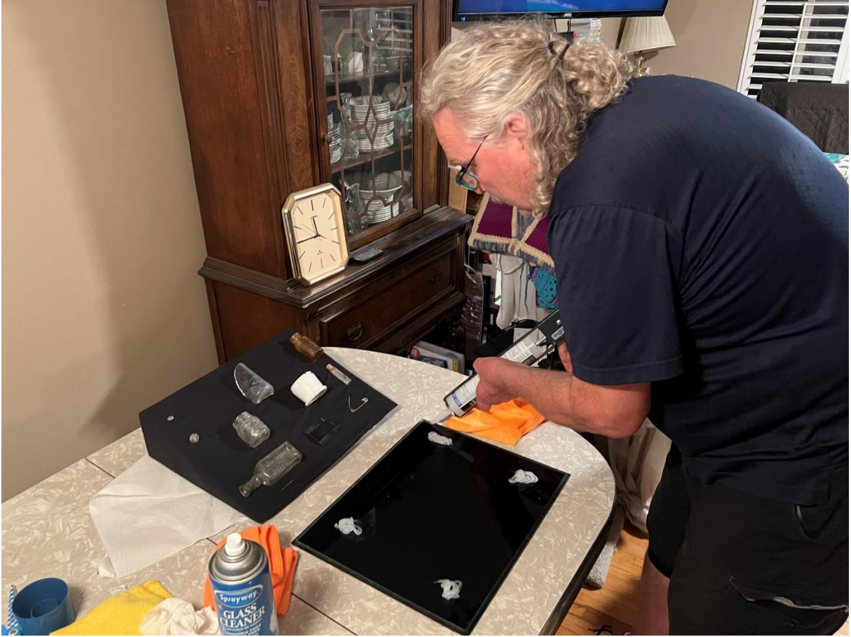
Figure 5.24 Placement of silicone rubber on base to adhere Ethafoam wedge. Photo by author.
