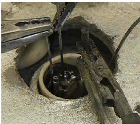
Figure 19. Electrolysis of LiCl-Li<sub>2</sub>O in attempt to remove moisture contamination for 2 hour at -0.7 V, Mo WE, Mo RE and graphite CE.
