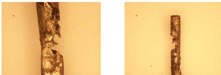
Figure 85. Optical images of pre- (left) and post-Tafel polarization (middle and right) of Ni electrode in LiCl-2wt% LiOH.
