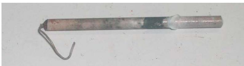
Figure 59. Post-testing reference electrode composed of silver wire immersed in LiCl-KCl-2.5 wt% Ag/AgCl inside mullite with fritted end.
