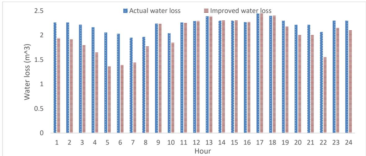
Figure 3. 7: Actual cooling tower water loss versus improved output
