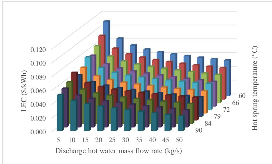
Figure 4. 11: LEC value for hot springs with different mass flow rates and temperatures
