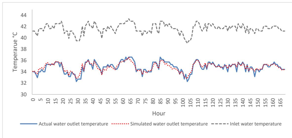
Figure 3. 10: Validation of the modeling results by using actual outlet water temperature
