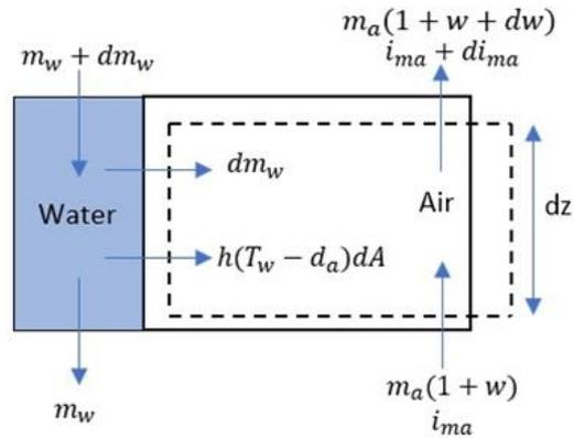
Figure 2. 5: Air volume control in the filling section
