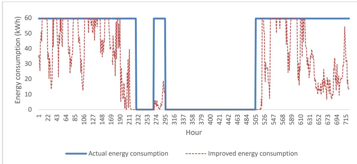
Figure 3. 8: Cooling towers fans energy consumption in actual and improved model in one month operation
