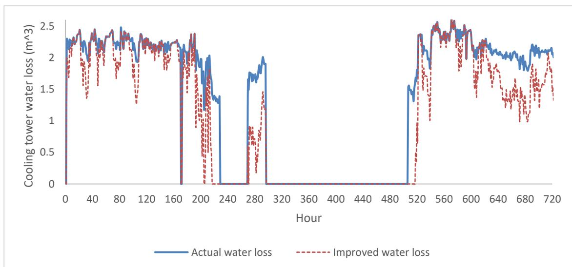
Figure 3. 9: Cooling tower water loss in actual and improved model in one month
