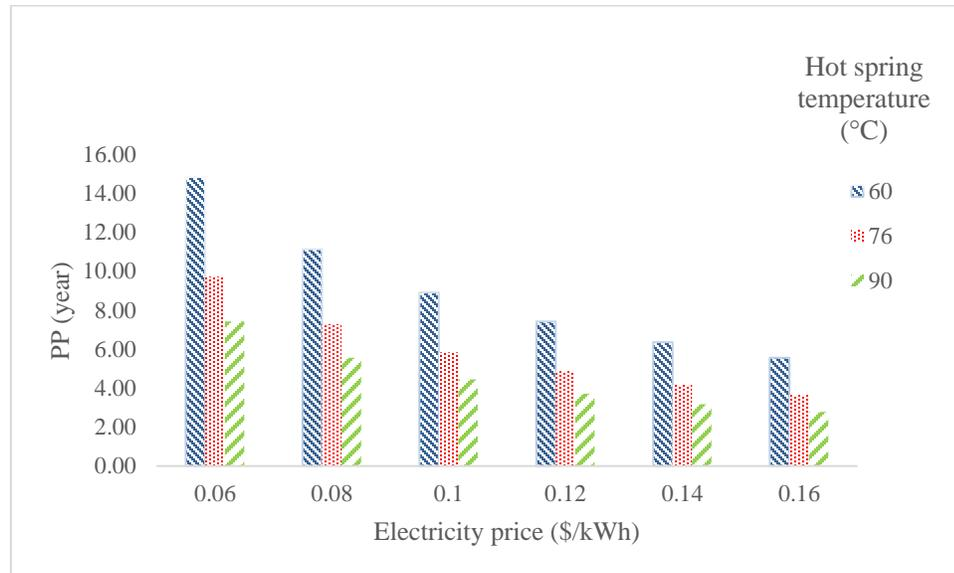
Figure 4. 14: The impact of electricity price on the Payback Period
