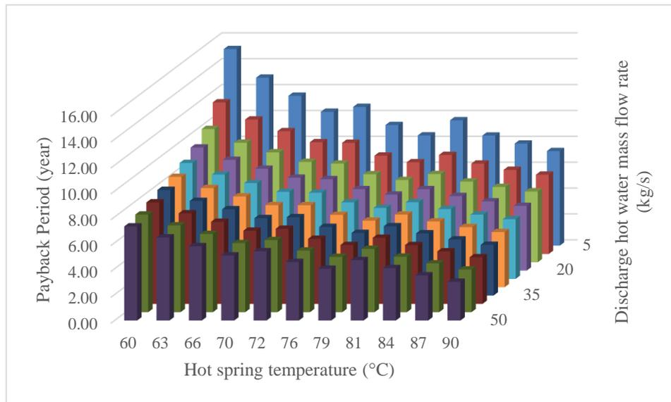
Figure 4. 12: The impact of hot water temperature and mass flow rate on the Payback Period
