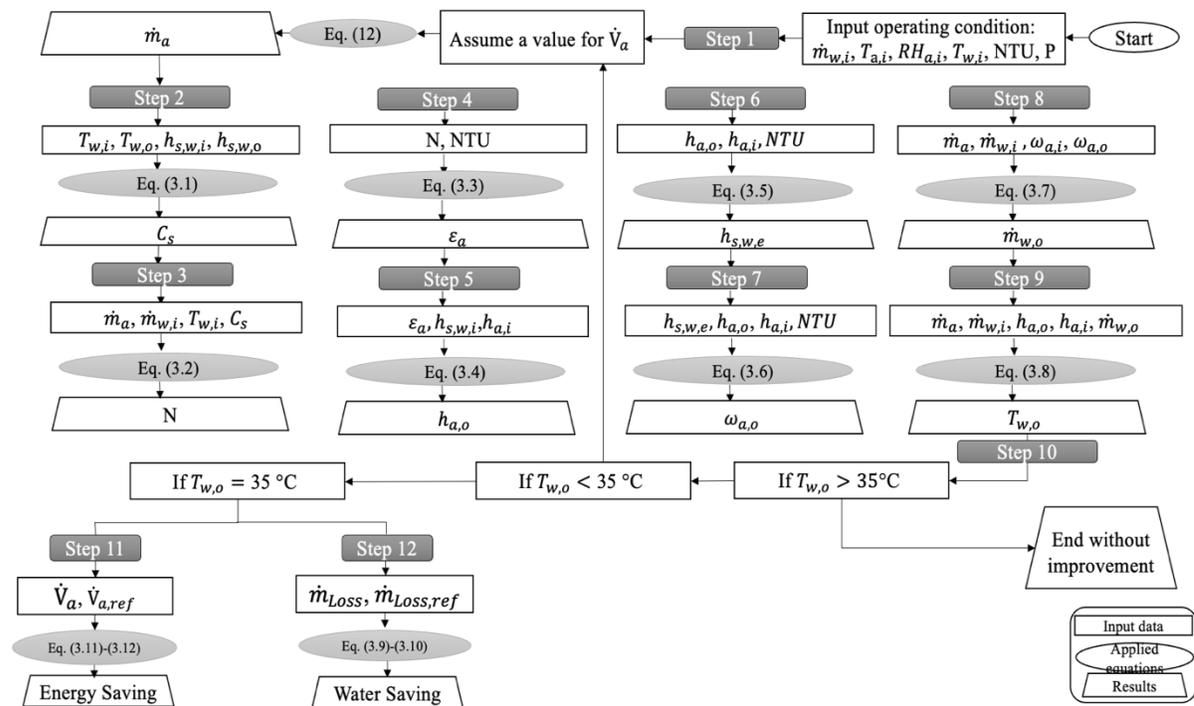
Figure 3. 3: Flowchart of using the developed model for improving the cooling tower water and energy consumption
