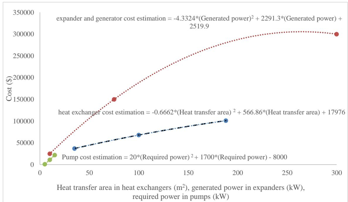
Figure 4. 5: Cost estimation curve for ORC components
