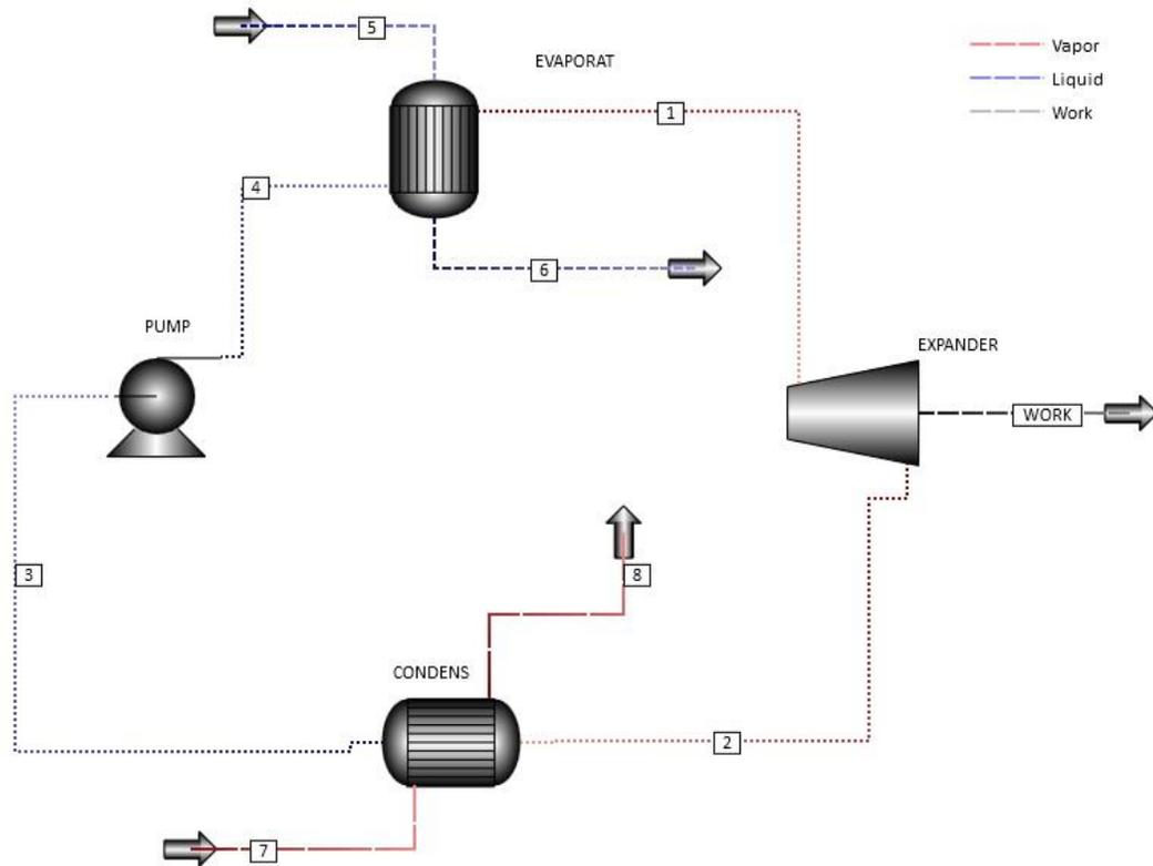
Figure 4. 3: Simplified model for ORC power generation
