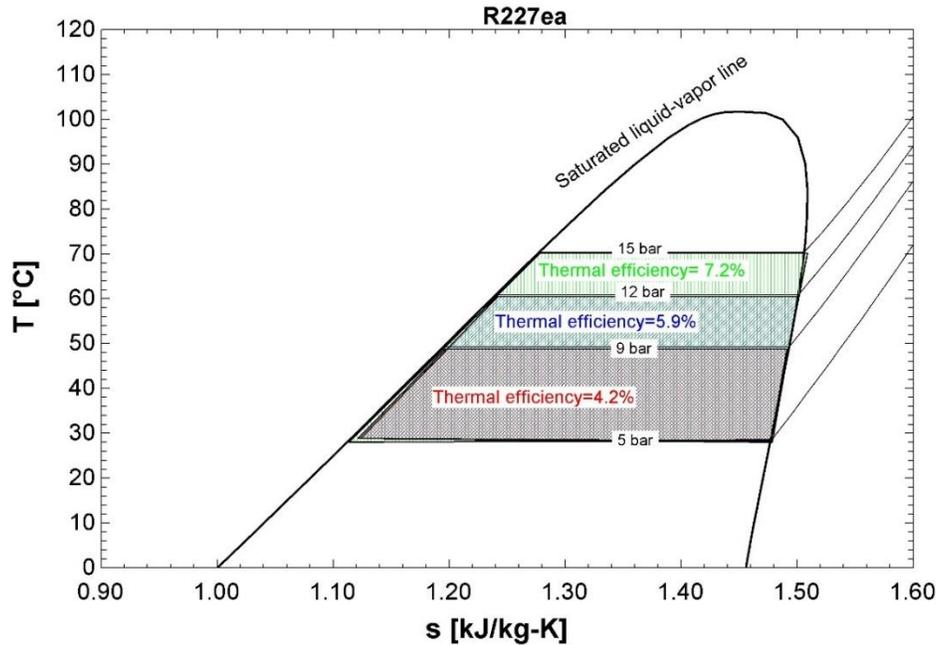
Figure 4. 8: Thermal efficiency of the ORC in the T-S diagram for three working pressures in the evaporator
