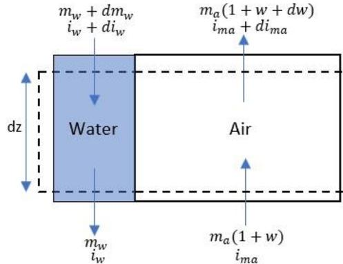
Figure 2. 4: Control volume related to the cross-section of the filler section
