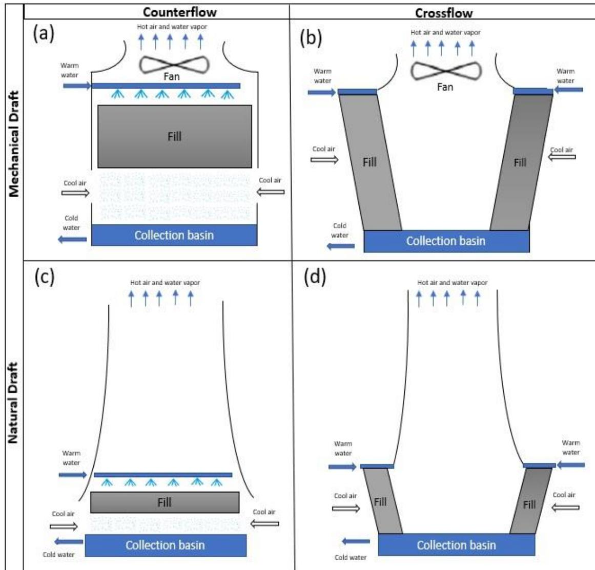
Figure 2. 1: The schematic of different types of wet cooling towers
