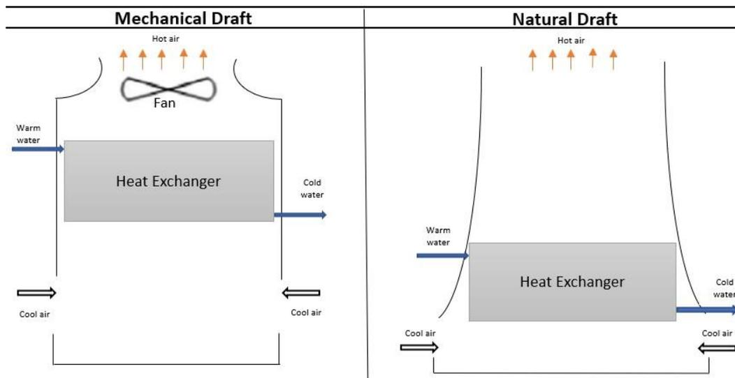
Figure 2. 2: The schematic of natural and mechanical draft dry cooling towers
