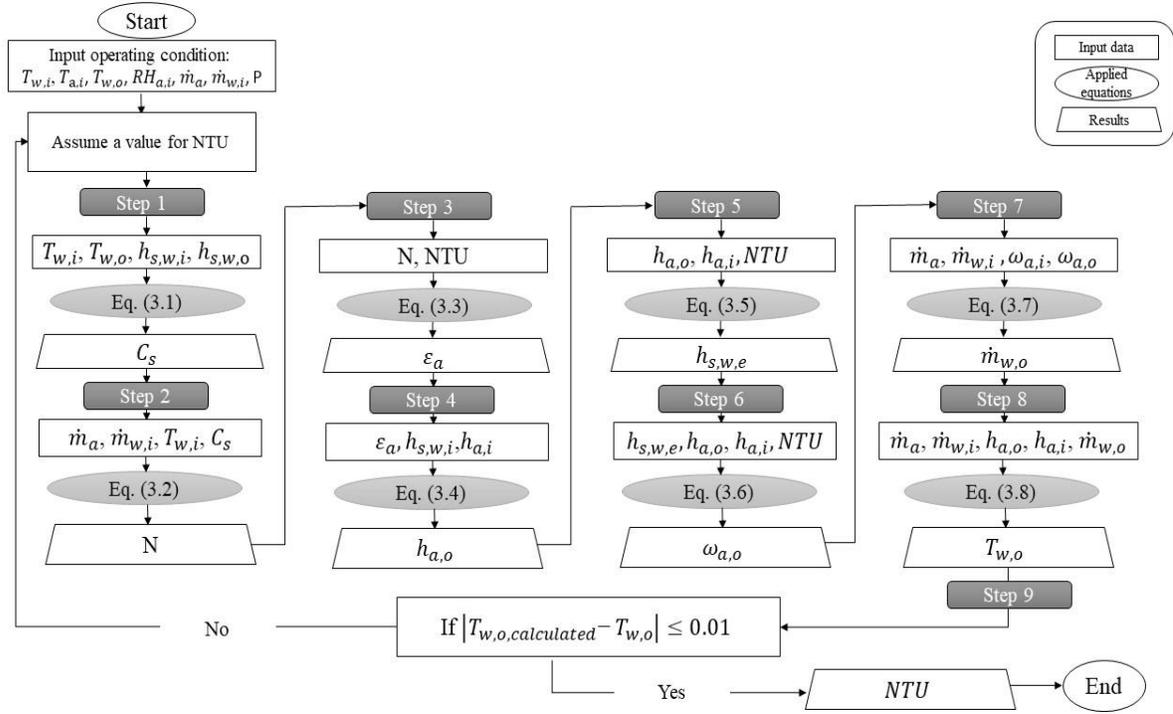
Figure 3. 2: Flowchart of using the developed model for finding NTU value
