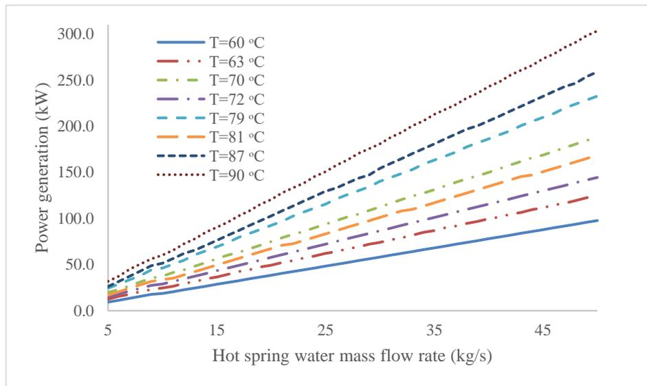
Figure 4. 7: The total working output of ORC using hot spring
