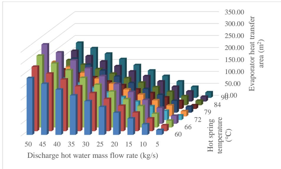
Figure 4. 9: The heat exchanger total heat transfer area for different hot springs
