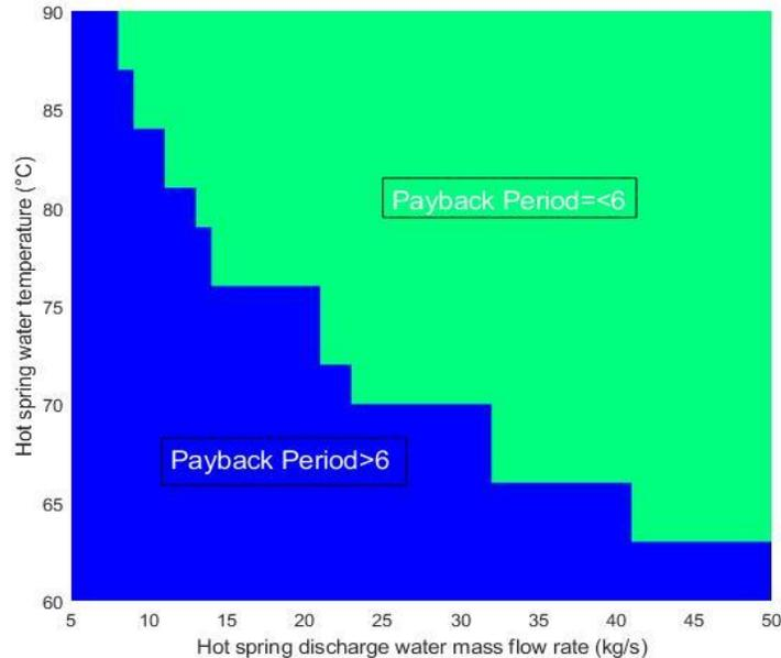
Figure 4. 13: The energy plant PP in different hot spring temperature and water discharge mass flow rate
