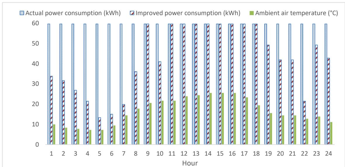
Figure 3. 6: Actual cooling tower fan power consumption versus improved output
