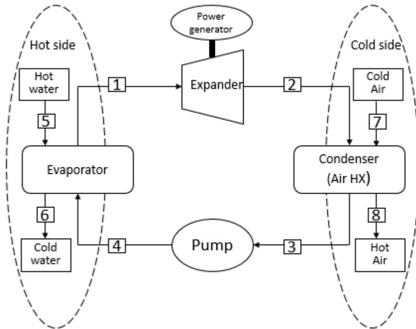
Figure 4. 2: Schematic of ORC power generation by using hot springs
