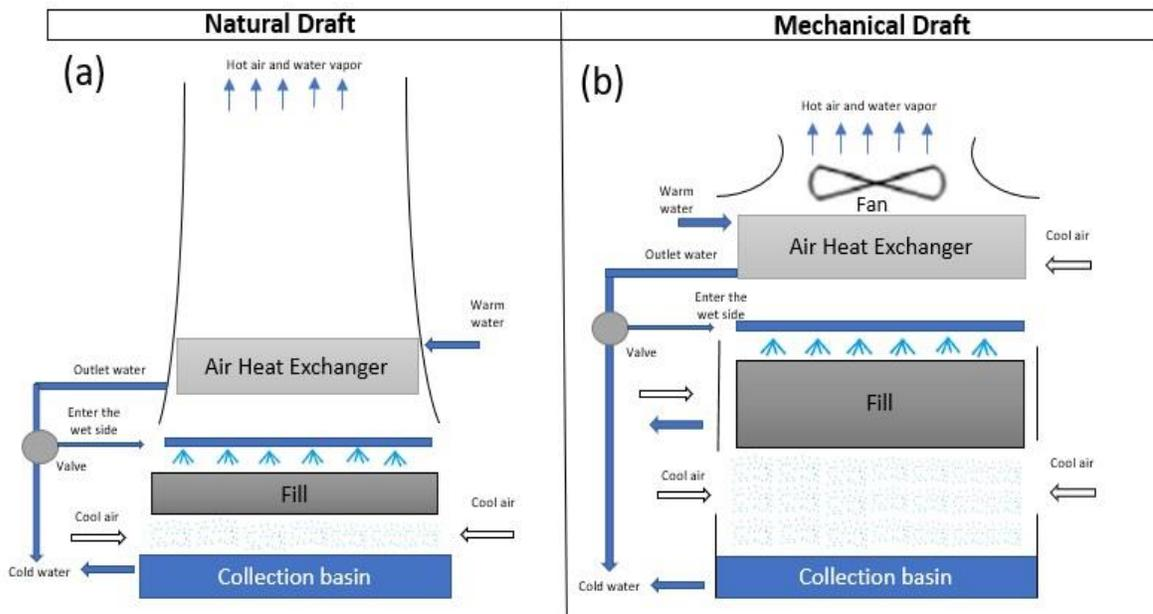
Figure 2. 3: The schematic of natural and mechanical draft hybrid cooling towers
