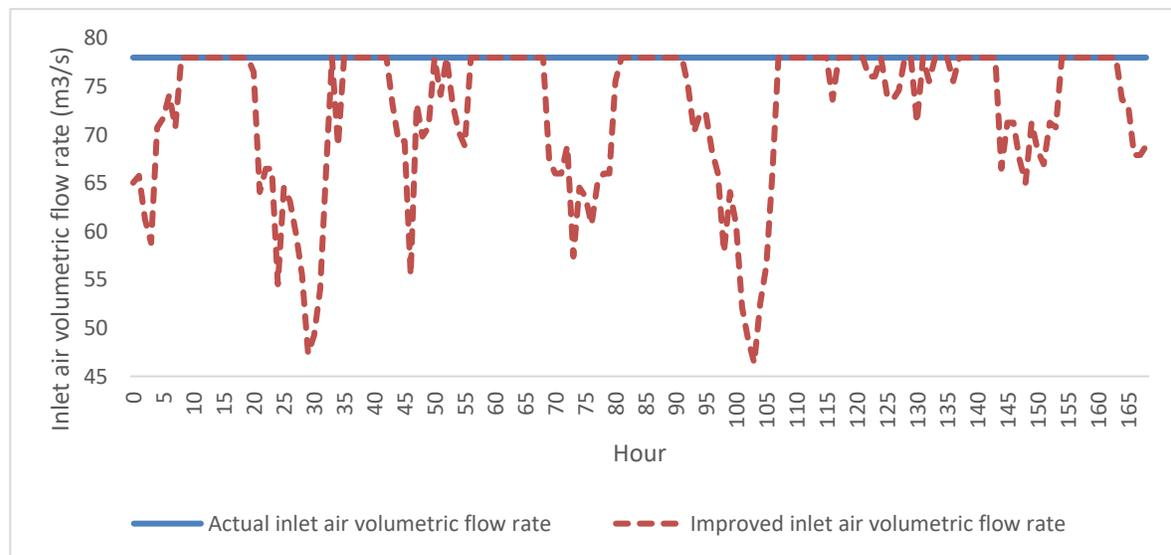
Figure 3. 5: Actual cooling tower air inlet volumetric flowrate versus the improved output
