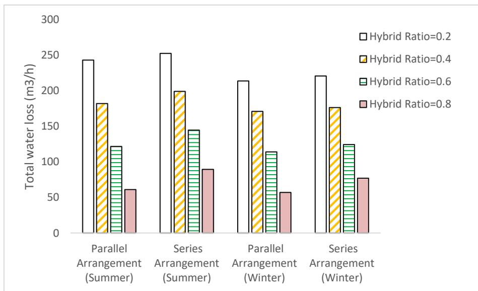
Figure 2. 6: The impact of heat-exchangers arrangement and hybrid ratio on water loss in different seasons at Tabriz refinery plant
