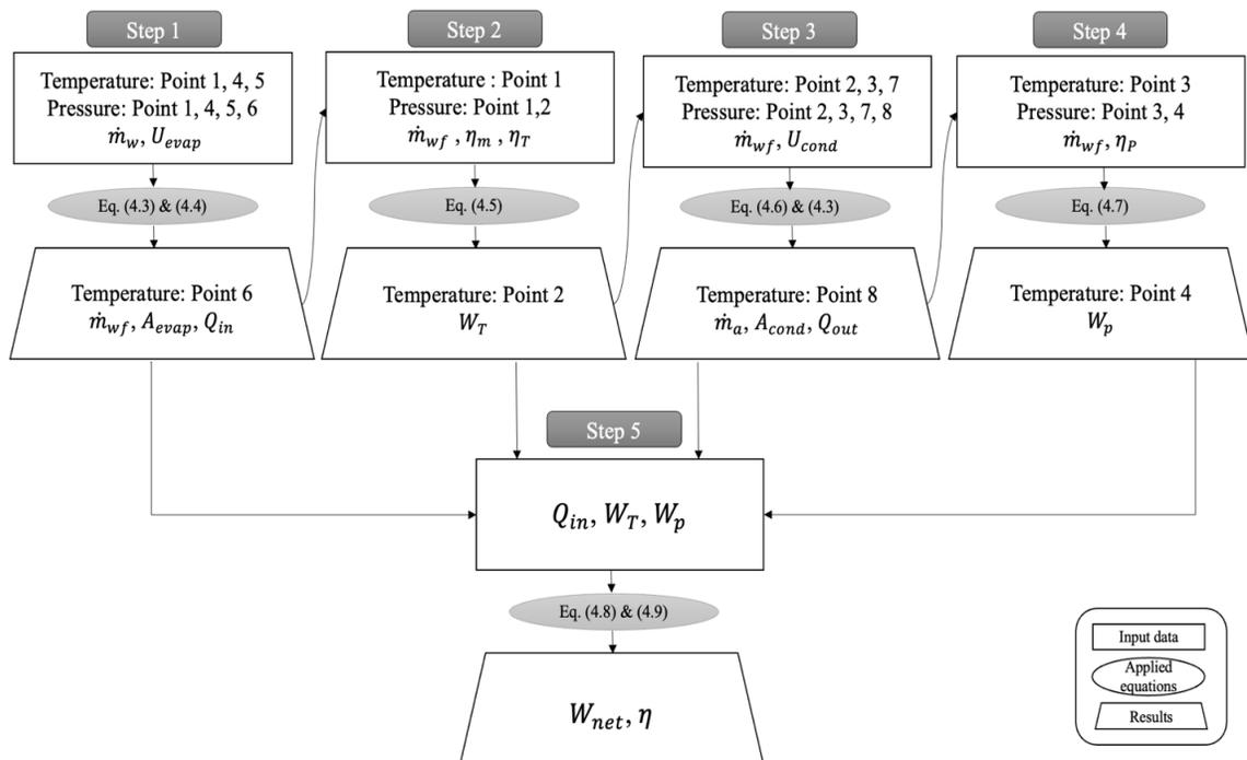
Figure 4. 4: Flowchart of the Technical Analysis of ORC energy plant
