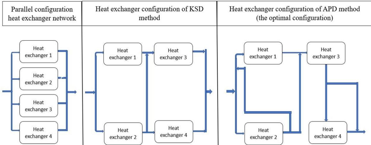
Figure 2. 7: Different heat exchangers network configurations
