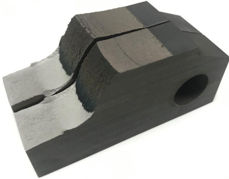
Figure 4. 13: Fractured halves of N-type C(T) specimens.
