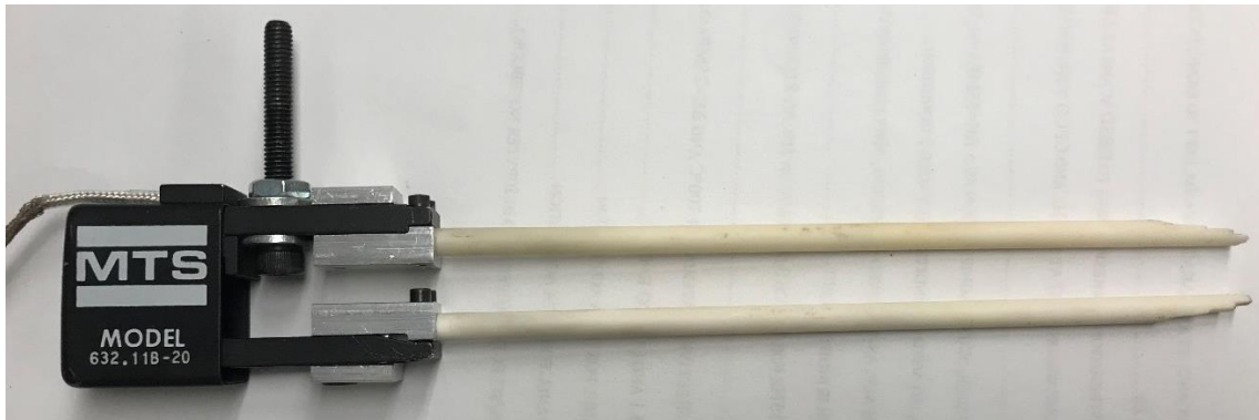
Figure 3. 9: Extensometer used in measuring COD of C(T) specimens.
