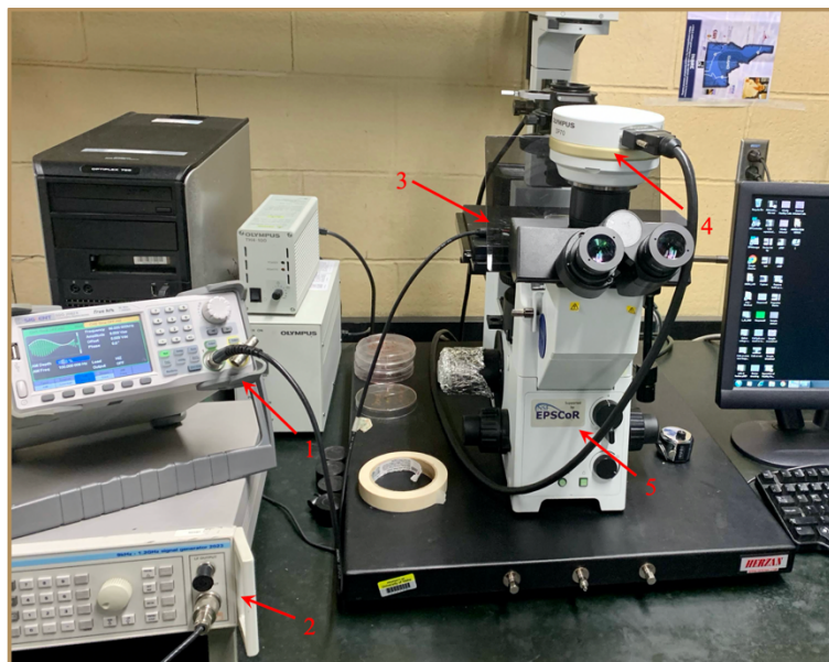
Figure 4.3: Image showing the experimental setup 1) Function Generator (Upto 80 MHz), f_{x1} experiments. 2) Function Generator (upto 1200 MHz), f_{x2} experiments. 3) Plane on which DEP microwell is placed. 4) Camera to record/visualize the experiments. 5) Olympus IX-71 Inverted Microscope.
