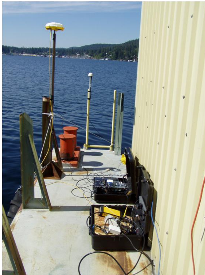
Fig. 10 The experimental floating buoy setup used in HBL navigation. Shown bottom-center are the hardware housing for the WHOI micro-modem. At top left is the DGPS receiver, directly below which is submerged the acoustic transducer. Visible at the building's corner is the tail of the AUV used to control communication and quantize DGPS position data
