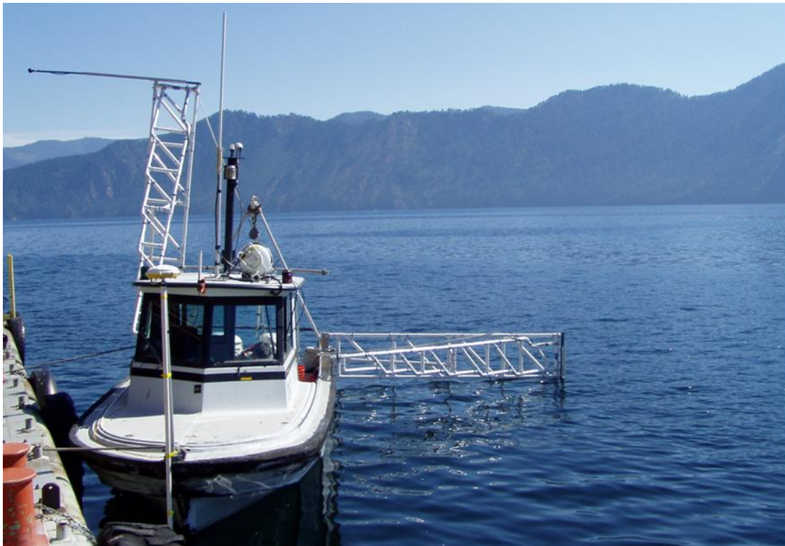
Fig. 9 The objective ship used in HBL navigation testing, moored to the barge test facility. Shown are the two outriggers supporting the transponders (sides of the ship), one of which is raised, and one of the differential GPS receivers (raised from the bow of the ship) used to acquire ship state data
