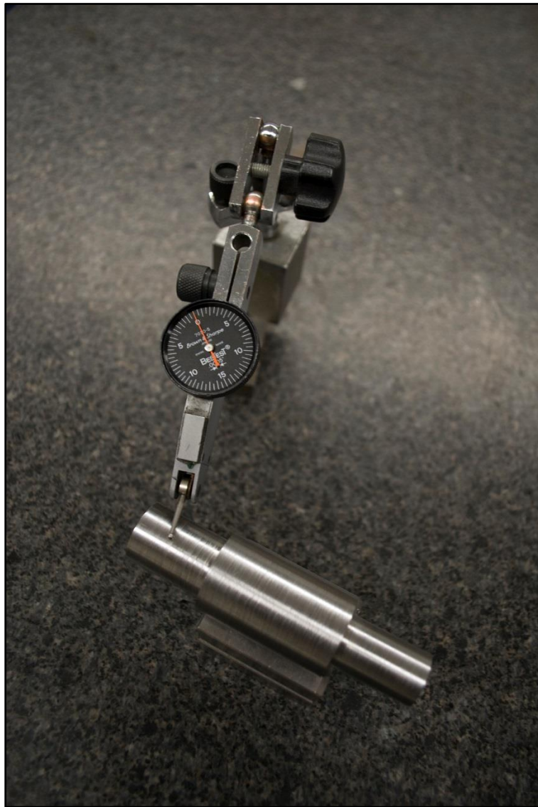
Figure 20: Measuring runout using a dial indicator and V-block.
