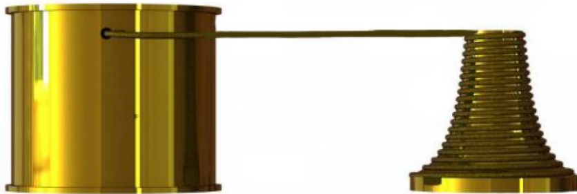
Figure 4.6: Fusee Mechanism Attached to a Spiral Spring Inside a Barrel
