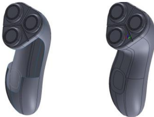
Figure 2.5: Left: Starting Model, Right: Complete Model in the Boundary Surface vs. Lofted Tutorial in the SOLIDWORKS Surfacing Workbook (See Appendix A)
