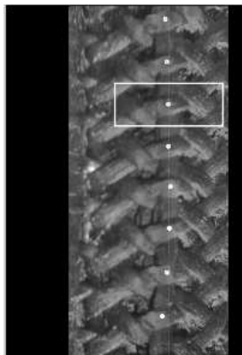
Figure 72: The effects of non-uniformity of illumination were removed using a morphological algorithm.
