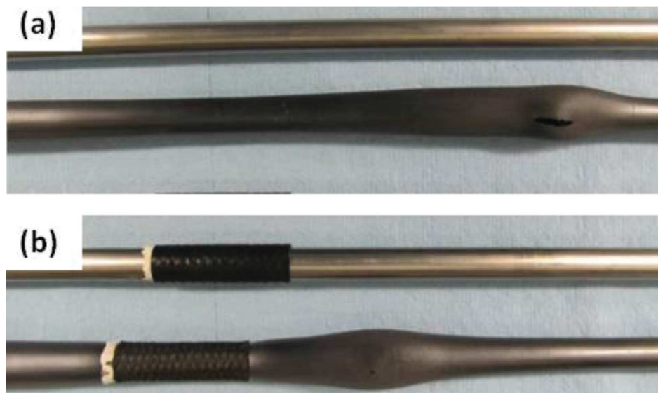
Figure 27: Photographs of starting samples (above) and ruptured samples (below) of (a) Zy-702 tube, and, (b) Zy-702 tube fitted with a SiC CMC sleeve [16].
