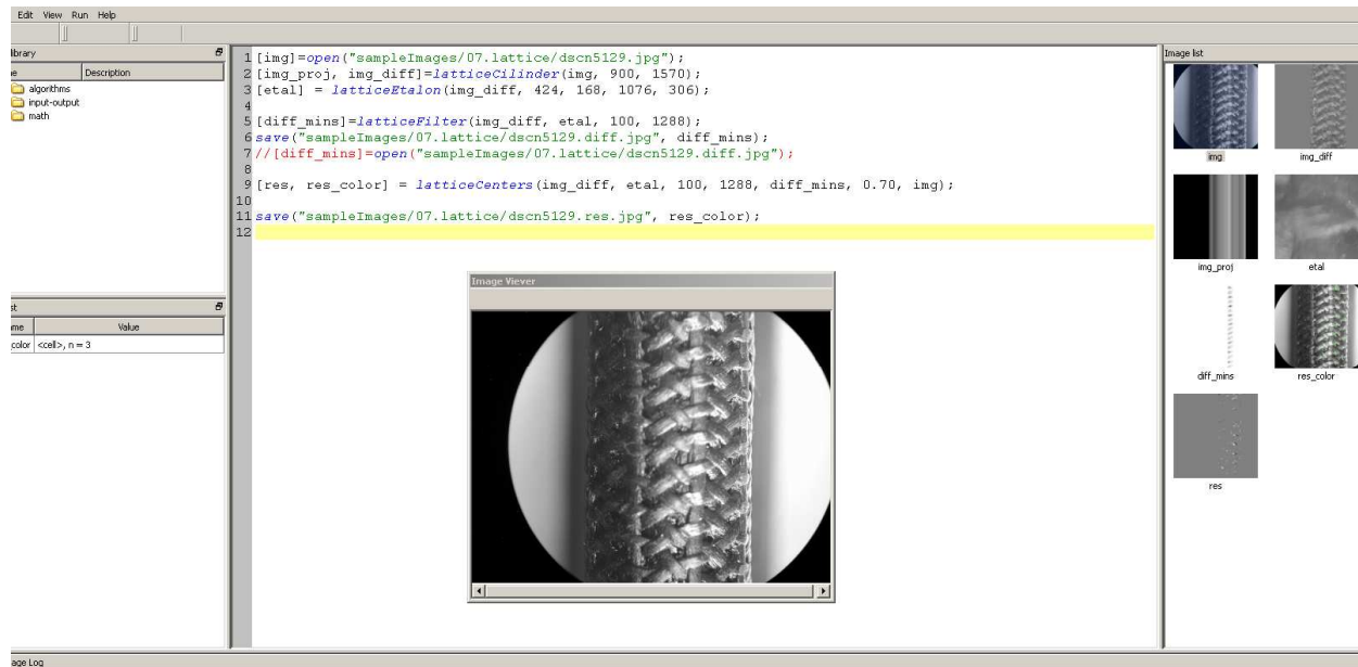
Figure 77: General view of the MorphoHawk platform and of the images generated by the developed MEX modules (the results of morphological processing).
